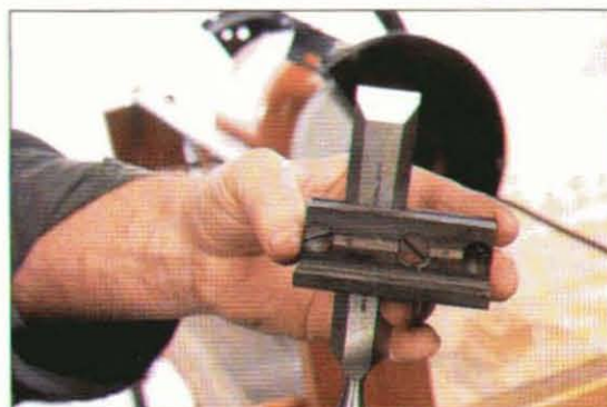
Grind chisels using exactly the same technique as you would with the plane blade. Note that chisels require a different tool holder.
