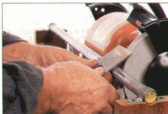
Successful grinding requires proper technique and equipment. This slow-speed grinder has been upgraded with a cool-running wheel, plus a tool rest and holder designed by the author.
