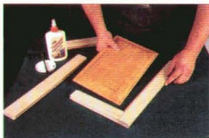
With raised panel doors, finish the panels first to avoid an unfinished line later.
