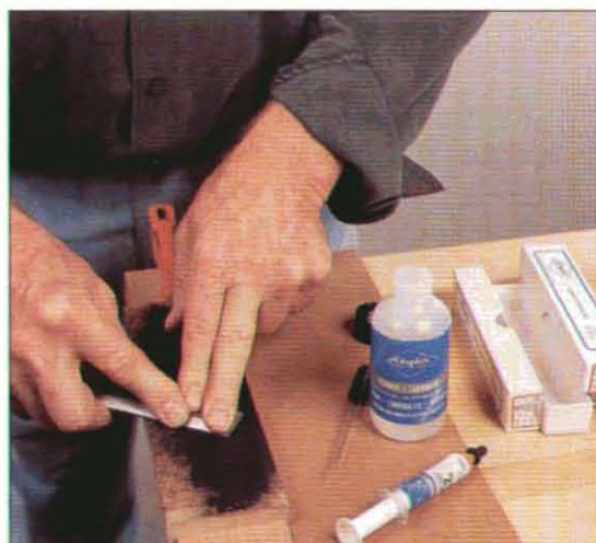
Resist the temptation to add too much paste. It won't increase the speed of your cut. Plan on an average polishing time of about five minutes per grit.
