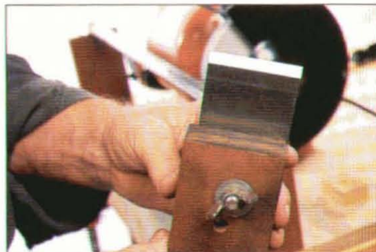
Produce an accurate grinding bevel (without burning), by applying light pressure and a moderate feed speed — don't extend the bevel to a feather edge.
