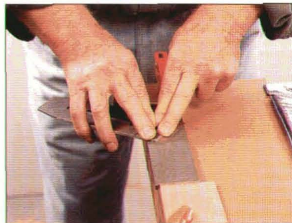
Diamond plates cut steel well. There's no water, no adhesives, no flattening, and no fuss. Of course, they are twice the cost of waterstones.
