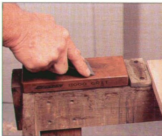
Freehand sharpening on a waterstone is fast and effective. The speed is due to the pressure concentrated on the small surface of the sharpening bevel. Use a honing guide if you're concerned about gouging the stone.
