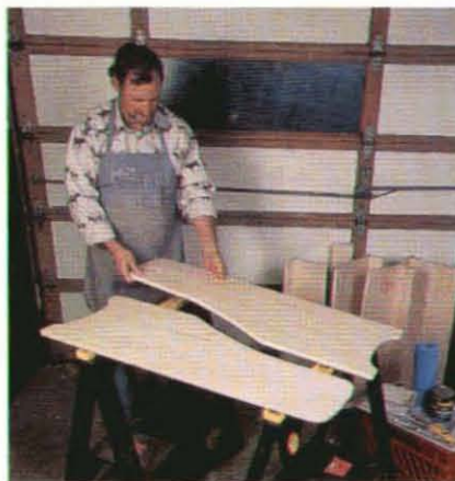
It's a lot easier to finish the sides of a bookcase as separate flat panels laid horizontally on a couple of horses.
