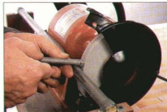
Dress the wheel to remove glaze and to make it perfectly round and square across its face. A diamond-coated block dresser provides proper control.
