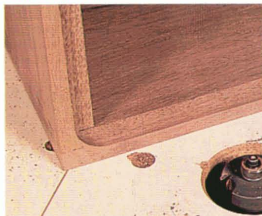
Form the 1/4" deep back panel rabbet with a bearing guided rabbeting bit. To be safe, the author used a table mounted router set up.
