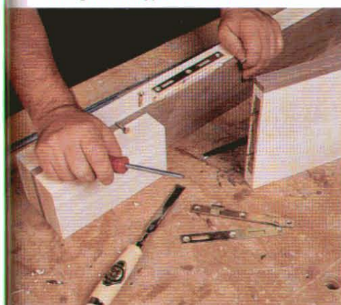
Installing knock-down bed rail hardware in mortises keeps it invisible when assembled.
