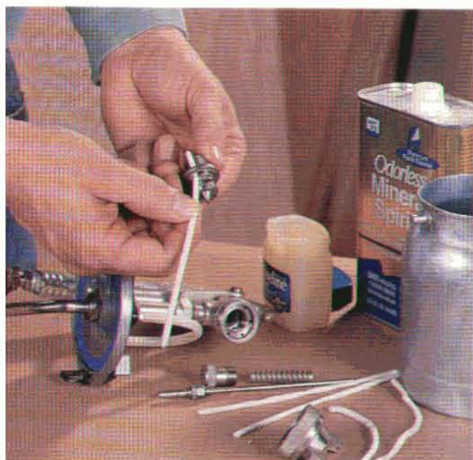
Break down your gun by removing the air cap, fluid tip and needle. Soak them in solvent until they are clean.
