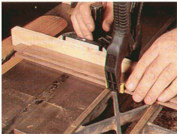
Cut the door rail tenon cheeks on your table saw using both the miter gauge and a wide dado head.
