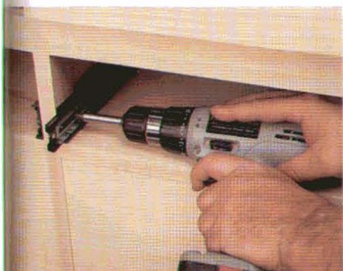
Heavy-duty drawer slides are an important feature, as the drawers (when open) do double duty as door supports.
