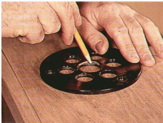
Use your router's base plate as a template when you're ready to drill both the bit access hole and the router base's mounting holes.
