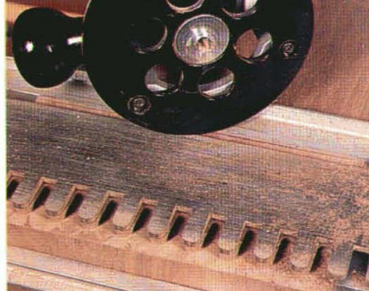
The author's aging Porter-Cable jig was up to the job of forming the half-blind dovetails.
