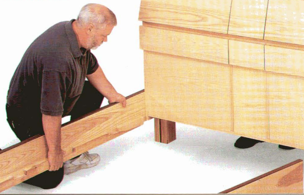
Installing knock-down bed rail hardware in mortises keeps it invisible when assembled.
