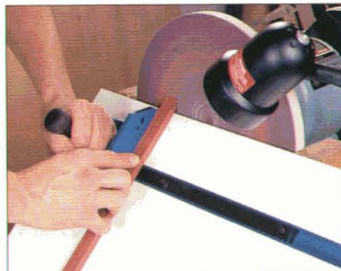
By adding a miter gauge slot, this shop-built disc sander can help create compound angles.
