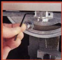
Fine tune micro-adjust trunnion.
