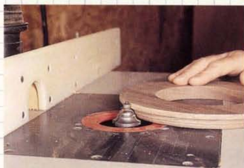
The jig works well with straight bits to cut circles, but it's easier to mill decorative edges on a standard router table.
