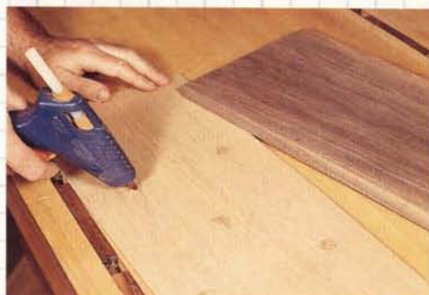
Locate spots of hot melt glue under each of the parts you are making, so that when a part is cut free it can't fall into the revolving bit.
