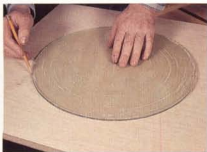
Figure 2: Center the Plexiglas disk on the sheet of MDF that will become the top of the jig, and scribe around the edge with a pencil.
