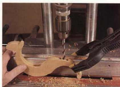
Figure 2: The loose mortises in the body can be chopped on the drill press: A mortising attachment is not necessary.
