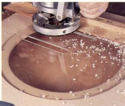
Figure 4: With a kerf cut through one edge of the jig top, clamp the disk in place and use a straightedge to mill the various grooves.
