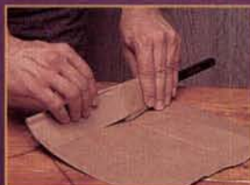
Roll up the ferrule and the clean wet bristles in brown paper bag material.
