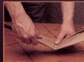
Feel for the end of the bristles and fold the paper over about 1" past the end of the bristle.
