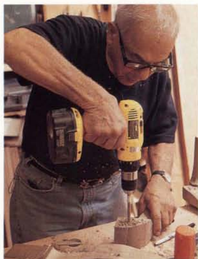
"I always keep a few kinds of washers" around the shop, Sam said. He uses them for tracing the holes he's about to drill.
