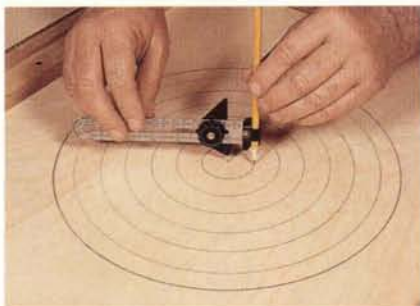
Figure 6: Draw a series of concentric circles 1" apart on the base, to center the workpiece under the router and minimize waste.
