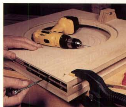
Figure 5: Predrill pilot holes for the screws in the continuous hinge that keeps the top and bottom of the jig properly aligned.
