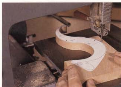
Figure 1: After attaching a full-size pattern to each blank, band saw close to the line and finish up with a sander.
