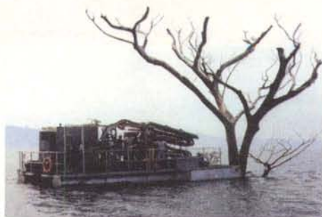
The original Aquatic Timber Harvester can reach to 60 foot depths. Production began this year on an ATH with a 120 foot reach.
