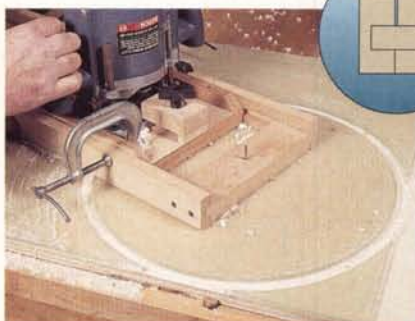
Figure 1: Use your regular circle-cutting jig to create the Plexiglas™ disk at the heart of the new jig. Back up the cut with scrap plywood.
