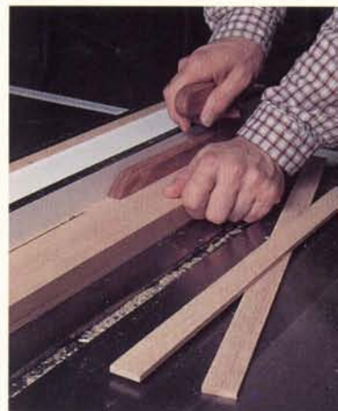
The author's over-the-top push stick requires only a single setup per slat dimension.
