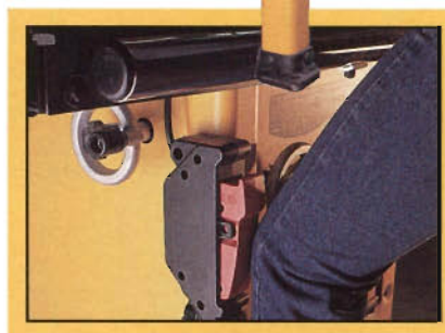
It's easy to reach the large paddle on the ON/OFF switch with your hand or knee. A padlock easily locks the saw.
