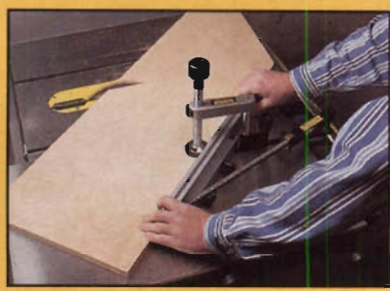
The DeWalt miter gauge is a modified version of the Osborne miter gauge and allows for mitering 45 degrees both right and left.
