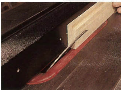
Figure 8: Once you've completed the V-groove and rabbet on your molding, switch to a fine rip blade for the chamfer cut. Be sure to use a feather board and push stick for this operation.
