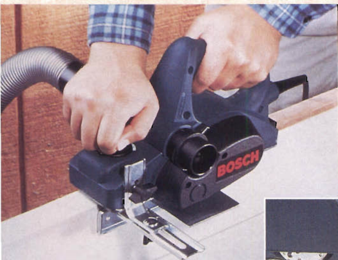
Bosch's new 3365 features the Woodrazor tungsten carbide blade.
