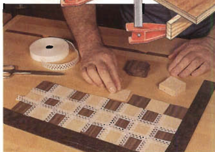
Figure 4: Use special, quick-sanding veneer tape to assemble the squares of veneer into a grid. Apply the tape to the best side.
