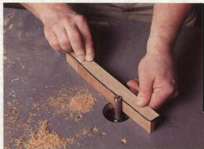
Template routing a subtle curve is the first step in making the desk's drawer handles. Use double-sided tape to attach the template.
