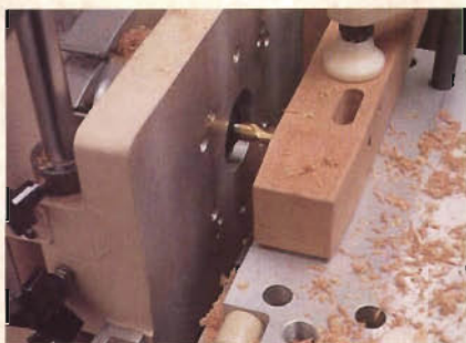
The author chops his mortises with a Multi-router. This project's mortises are all straightforward mortises which can be formed just as easily in the traditional manner.
