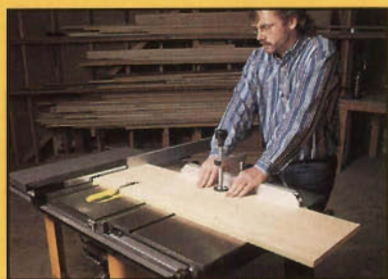
The author uses the slider to cross cut some sheet stock. Note that the aluminum rip fence is drawn back to prevent crosscut binding.
