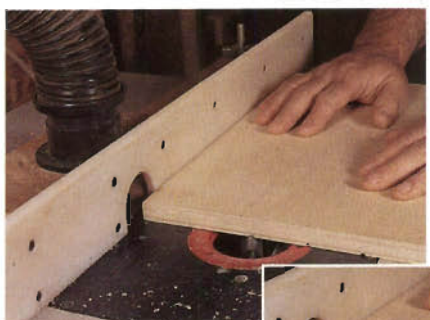
Figure 6: Use the same 45° V-groove bit to plow the groove in the top of the frame (inset) as you did for the checkerboard grid.
