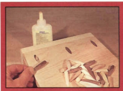
The company offers precut wood plugs in a variety of wood species. Here, I used a plug of a contrasting color (walnut) to add visual interest.
