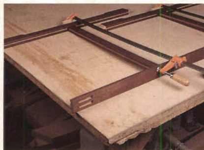
Begin assembling the pedestal's side subassemblies as shown above. Note the top rails' orientation and pocket screw joints.
