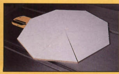
To test the angular error of a miter cut, I make multiple wedges to form a circle. This will compound any error, making it easier to measure. Here, the error for a 22½° miter is multiplied 16 times. Very impressive.
