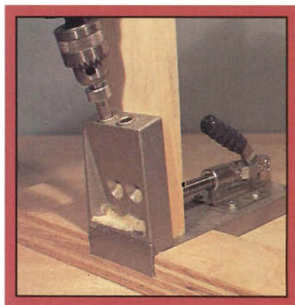
Relief holes on the backside of the jig prevent sawdust buildup inside the guides.
