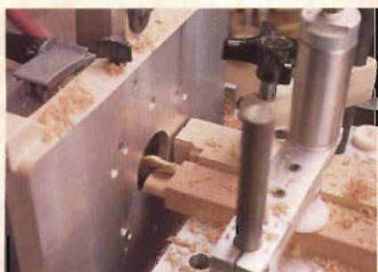
Tenons on the panel dividers are shorter than those on the bottom rails. Test fit the tenons in their mortises as you make them.
