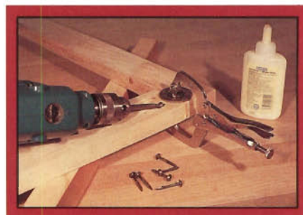
Step 3: Apply glue to the mating pieces and clamp together, making sure the pieces are flush. After driving screws, release the clamp.
