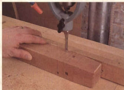
The author used a mortising attachment on his drill press to create the square mortise for the leg's decorative ebony plugs.
