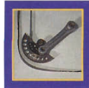
The toothed drive segment converts the rotary motion of the motor into the oscillating action of the drive belt.
