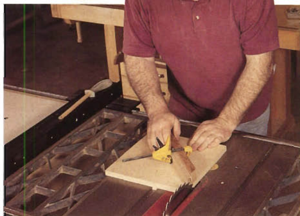
Figure 1: Create a sled to form the miters on the ends of these small pieces. It's safer, more stable and more accurate.
