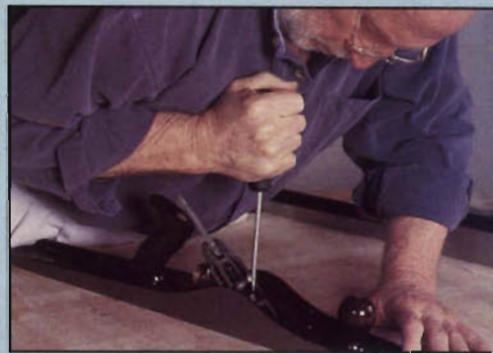
Adjust the frog to support the blade securely. The mouth opening should be set to 1/32".
