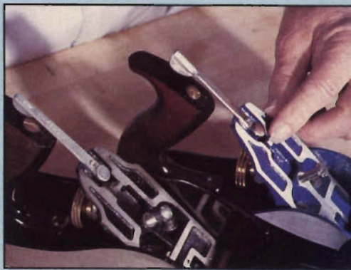
Old-style blade controls (left) are more robust than the stamped metal ones in recent planes.
