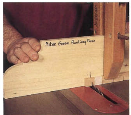
Figure 3: Tape the horizontal and vertical dividers together in groups with the notches plainly marked on the forward piece. Clamp the pieces to an auxiliary fence when cutting.
