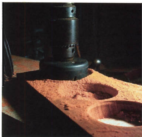
For perfectly matching scalloped rack pieces, chuck a hole saw in your drill press and bore holes down the center of a single piece of wood.
