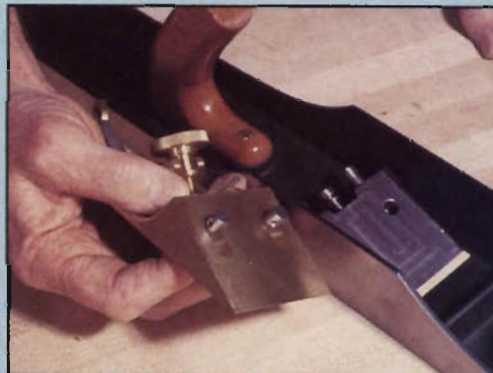
The bedrock style frog (above) firmly and ingeniously connects the blade assembly to the body. A regular frog is not as massive and does not seat as firmly.
