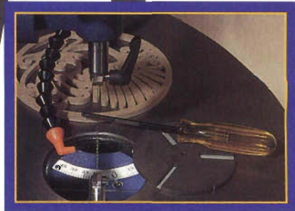
A precise table tilt scale (the table tilts 45° in either direction) is easily readable from above, through the inset opening.
