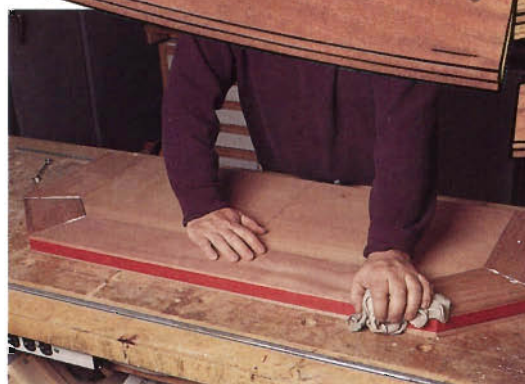
After slotting for biscuits, apply glue and then secure the five pieces of beaded trim around the top using a band clamp.
