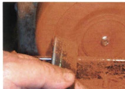
Turn the wheel true, then mark the points for its central depression. Use a sharp skew for this step, making fine cuts. When one side is right, reverse the wheel to turn the other side.
