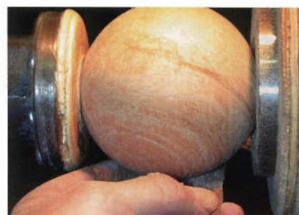
Make sure you keep moving the hole cutter through all three axes during the roughing process, then work your way through the grits.
