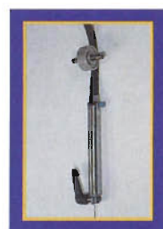
The upper blade clamp, connected to the toothed belt. Note the large, multi-positionable clamp lever.
