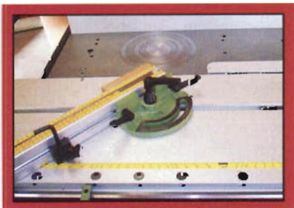
An extremely accurate miter/cutoff gauge. All of the elements of the sliding table saw system are engineered to exact tolerances.
