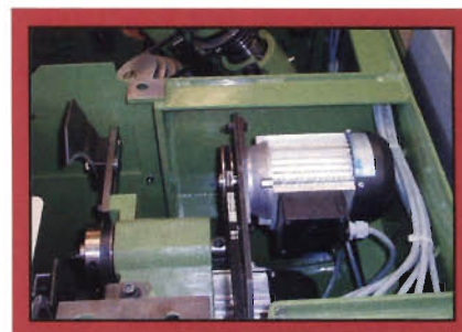
One of three 5.5 HP Siemens electric motors. Power is never a concern with Knapp's ultimate combination machine.
