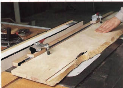
The hold down option on the jig will allow you to slice a straight edge on a rough piece of stock.
