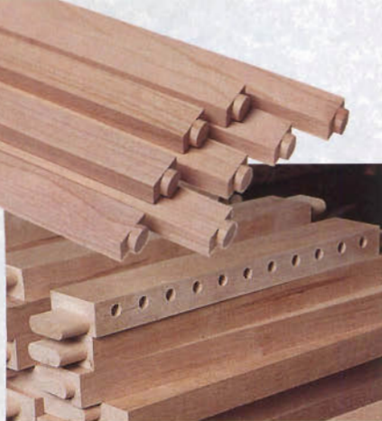
The author used his Multi-router to create tiny round tenons on the end of the slats. Our alternate method is "notched slat receivers."
