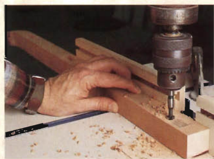
The mortises on the legs are the same size, but are asymmetrically placed. Use a sharp Forstner bit to rough them out.
