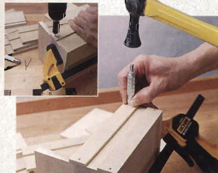
Attach the fronts and backs to the sides (after slipping the bottom in place) using glue and nails. A nail spinner and nail set make fast work of the multiple drawer assembly.
