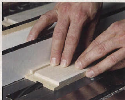
Plow grooves in the faces of the drawer sides (for the drawer runners) using a dado head and the saw's fence. Use your new dado sled for the rabbet cuts (see page 48).
