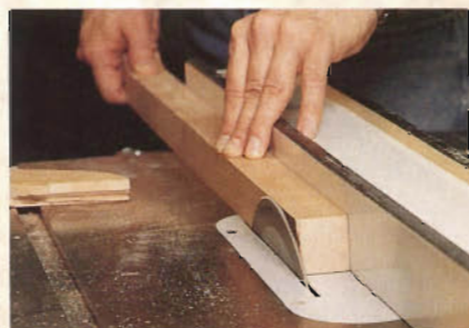
After the mortises are chopped, the front legs are sliced to match the angled shape of the chair's footprint.
