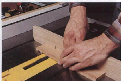
Lay out and notch the slat receivers in matched pairs on your table saw. In this operation, accuracy is critical.
