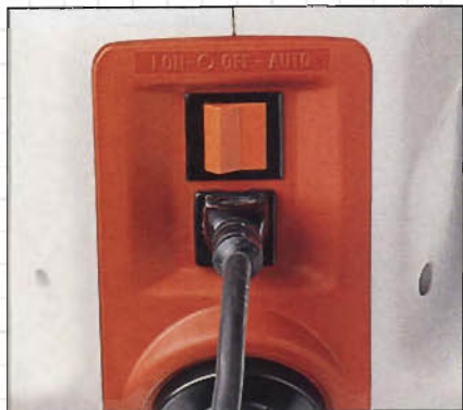
Rick used a shop vacuum with a special switch designed to be used with dust-creating power tools. When you plug your sander into the vacuum, each time you start the tool — the vacuum starts. When you turn your tool off, the vacuum continues for a short time.
