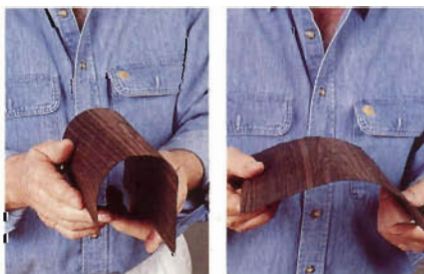
Tight side, loose side. The veneer curls more easily with the loose side out (left). When possible, glue the loose side down.
