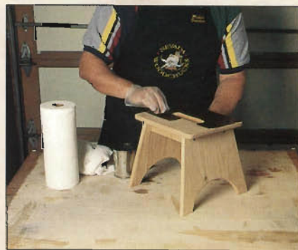
Flood the surface of your properly sanded project with the mixture. A generous application helps to insure uniform coverage.
