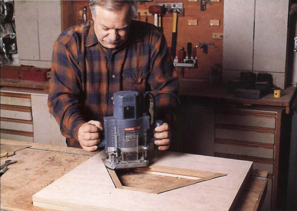
Figure 4: Use a rabbeting bit and a shop-made jig to safely and accurately rabbet the back of the shade frames. Homemade jigs are the key to success with this Prairie project.
