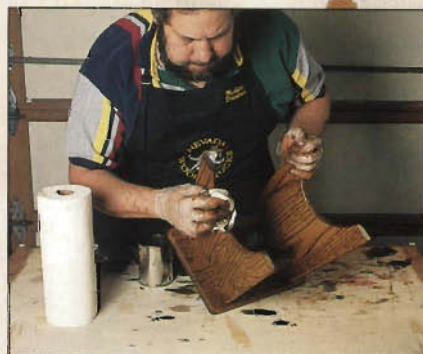
Wipe the stain off before it dries. Move quickly, but thoroughly rub the entire piece, working toward uniform coverage.
