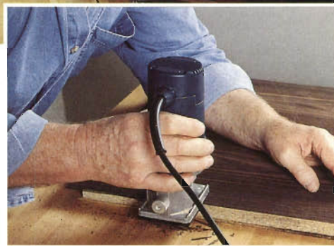
When the glue has dried, clean-up is easy: rout the excess veneer flush with the substrate and sand smooth.
