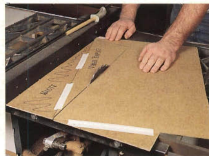
Create hardboard templates of the shapes which comprise the face veneer pieces. Find these shapes on the Full-size Pattern.
