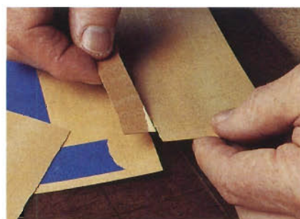
To repair a crack in your veneer, simply smear a little glue in it and tape until dry.
