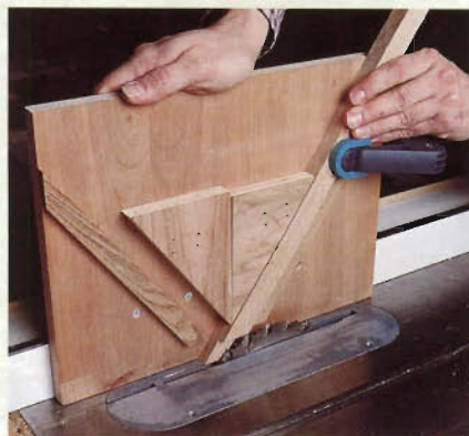
Figure 3: With the same dado blade in your table saw, use our jig to help chop the mortises and slice the tenons on the ends of the frame's stiles and rails.
