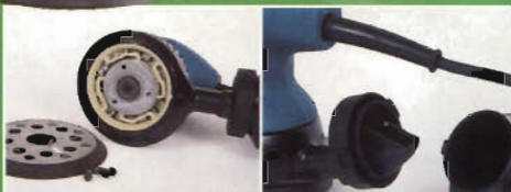
The Makita's dust bag has a locking rim, but leaks at the edges of the bag. Its molded plastic pad brake works effectively.
