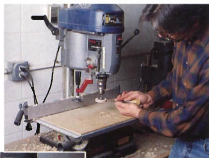
Figure 2: Make a wheel sanding jig from a 3/16" threaded rod, a nut, two rubber-backed washers and a wing nut. Use the jig to score the wheels for their O-rings, too.
