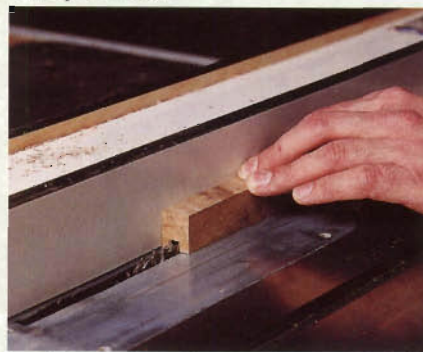
Figure 2: Before cutting the rails and stiles to length, use a dado blade to plow a groove. This will make it easier to create the rabbets for the glass after you assemble the frames.
