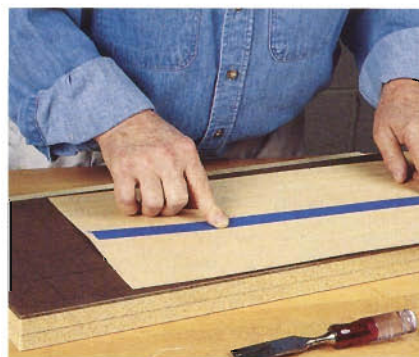
Glue veneers by stretching tape across the joint line, then tape along it and fold the seam open. Run a thread of glue on the edges, refold the joint, scrape off the excess glue, and tape the other side.
