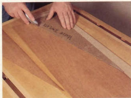
Using the appropriate templates and a sharp knife, slice the radiating face veneer pieces from contrasting hardwood veneer.
