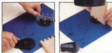
Each revolution of the knob adjusts your bit height .050". Remove knob for machining.
