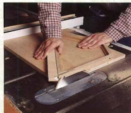
The first jig miters the left side of the frames.
