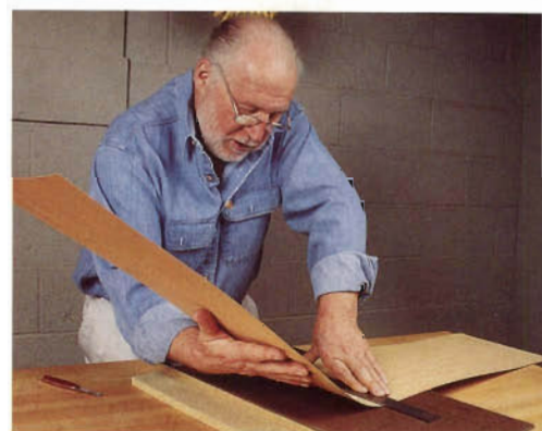
Cutting veneers: Use a sharp knife against a steel straightedge. To crosscut, press hard for one or two passes, then snap the veneer by lifting it against the straightedge. To cut with the grain, press lightly and make multiple passes.
