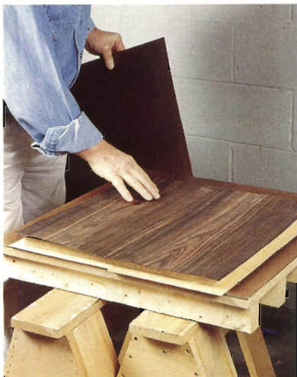
Assemble the press, platens and panel on a couple of sawhorses, so you'll have lots of room for clamps. Tighten the clamps in pairs, working from the center outward.
