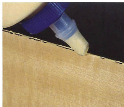
To repair a crack in your veneer, simply smear a little glue in it and tape until dry.
