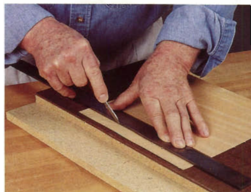
Cutting veneers: Use a sharp knife against a steel straightedge. To crosscut, press hard for one or two passes, then snap the veneer by lifting it against the straightedge. To cut with the grain, press lightly and make multiple passes.
