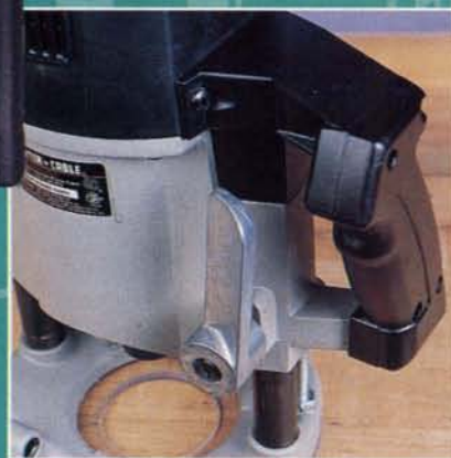
The spring-loaded plunge lock lever on the Porter Cable router locks the depth when you release it.
