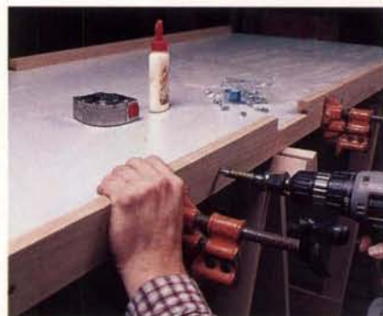
Figure 2: Attach the rails to the melamine deck with screws and glue. Cover the exposed screw holes with walnut plugs.
