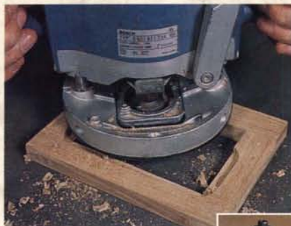
Figure 2: The size of the rabbeting bit and bearing is critical. The goal here is to fit a square cornered piece of glass into an opening with rounded corners.
