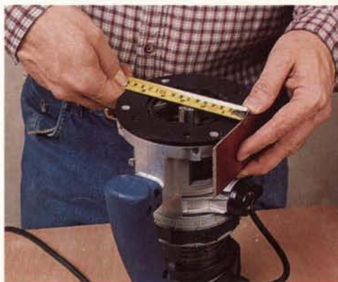
Figure 1: Determining the space required for your router is critical to the success of this jig. Measure your router and the two pieces of laminate to get the exact dimension.
