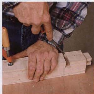
After you plow your stopped dovetail dado onto the apron, square up the end of the dado with a sharp chisel.
