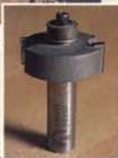
Figure 2: The size of the rabbeting bit and bearing is critical. The goal here is to fit a square cornered piece of glass into an opening with rounded corners.
