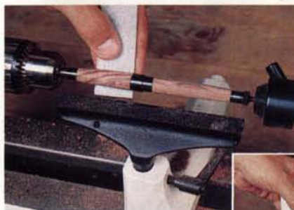
Figure 3: I sand and finish from the back on runs like this, so I don't have to keep moving the tool rest back and forth. Just be careful!
