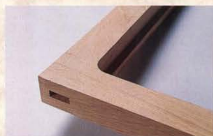
Figure 2: Assemble the desktop frame and cut a rabbet in its bottom edge with a bearing-guided bit. Square the corners with a chisel.
