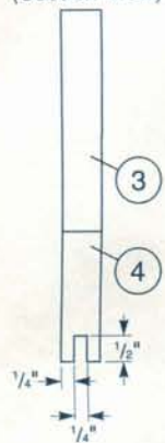
Top/ Middle Rail (Section View)
