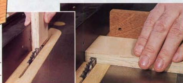
The drawer fronts and backs (left inset) are rabbeted on their ends. Drawer sides (above right), have 1/4" dados milled across their ends. Both steps can be done on the same set-up, as shown above. Also, the 1/4" drawer bottom grooves are formed on the same table saw set-up.
