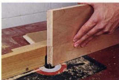
Figure 1: Plow grooves into the appropriate edges of the rails and glued-up rails. Take a few passes to achieve the proper depth.
