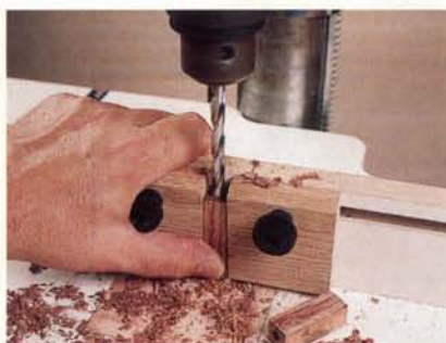
Figure 1: Equip your drill press with a good fence and stop system for this production project. Remember to continually back out the waste as you drill through the blank.
