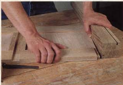
Figure 3: Before final assembly, test fit the joints between premade subassemblies, such as the back subassembly and the legs.
