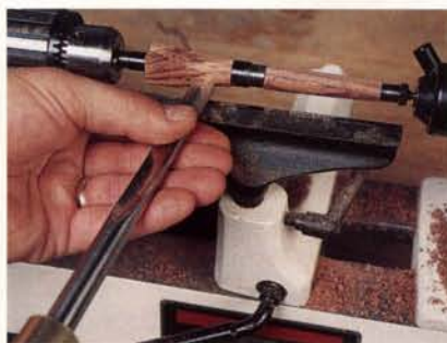
Figure 2: When turning the pen's elliptical shape, don't get aggressive and trim your bushings. It dulls turning tools and makes for very small pens toward the end of a run. Get close and switch to sandpaper.
