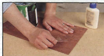
To book match the veneer, select successive flitches and join two pieces with packing tape, glue and a heavy weight.
