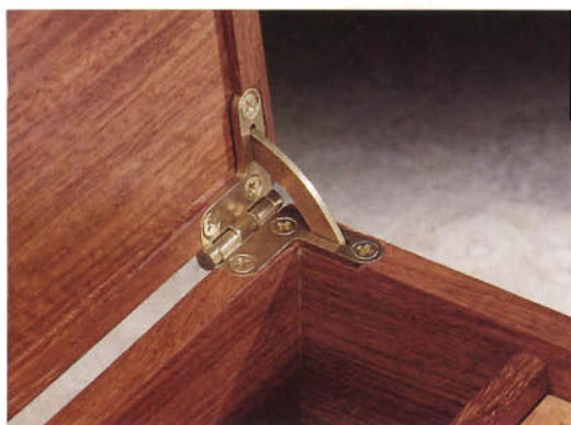
Quadrant hinges look simple, but require hidden mortises for the support arms to hide in. For this box, some of the screws provided needed to be cut down in length to fit properly.
