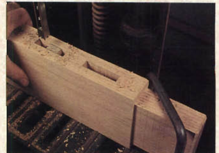
Figure 2: A mortising machine will make short work of the many mortises featured in this project's Stickley-inspired joinery.
