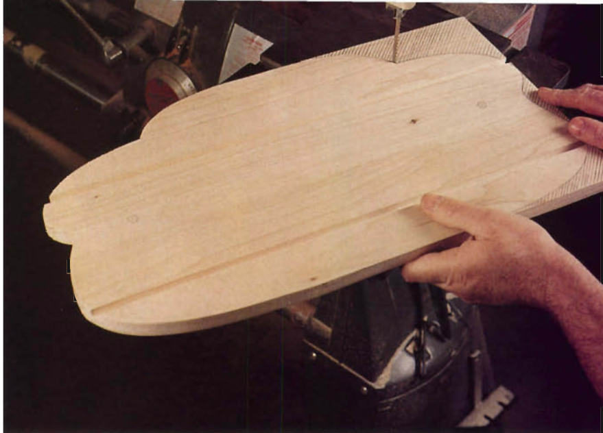
Once you've formed the grooves for the wings, use the Full-size Pattern to transfer the profile of the cloud onto the glued-up blank, then cut it to shape on the band saw.
