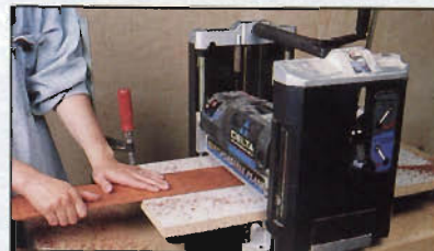
Use a slave board clamped in place to aid in planing your veneer pieces smooth. They must all be uniform in thickness.
