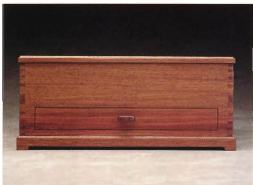
The front panel of the box was sliced into five separate pieces in order to achieve a tightly fitting drawer front.
