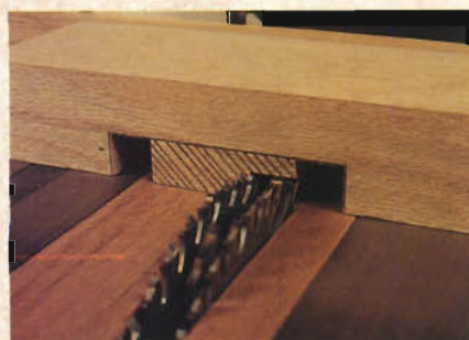
Figure 1: The leg mortises are formed before the legs are glued up. Simply slice wide dados to form one half of each mortise.
