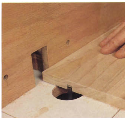
Figure 3: After gluing up a blank large enough to make the cloud, plow two shelf grooves before band sawing this piece to final shape.
