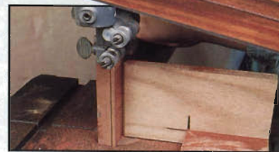
Resawing fat 1/8" veneer is the first step in creating handmade plywood. A point fence and a properly tuned band saw are essential.
