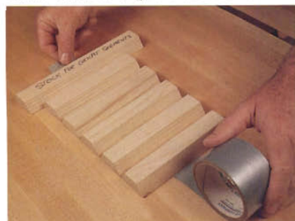
Figure 1: Duct tape, an airplane builder's secret weapon, comes in handy for testing the fit of the fuselage segments.
