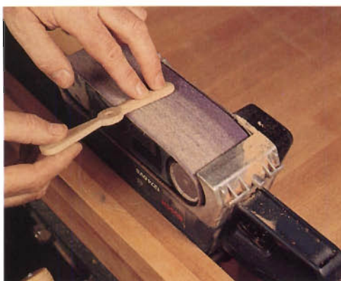
Figure 2: After cutting the propeller to shape on the band saw, clamp your belt sander upside down in the jaws of your workbench to carve the angled faces.
