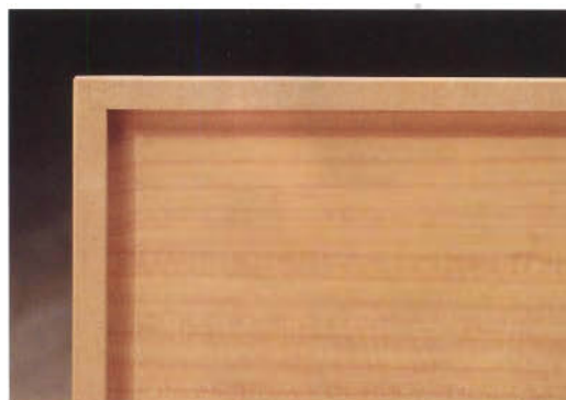
The tray bottom's edge is first shaped with a gentle cove and then captured by stopped grooves routed into the sides.
