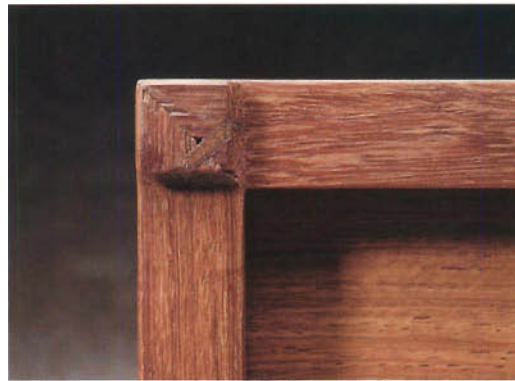
The mitered corners on the machiche base were reinforced with splines. The base is attached with dowels and glue.
