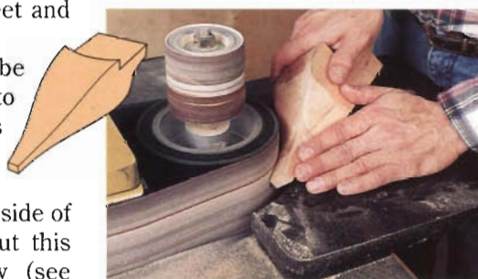
Figure 5: The distinctive and complex shape of the oval coffee table's feet is best completed on a belt sander.
