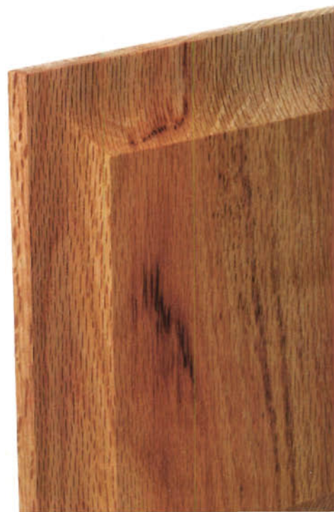
Figure 2: The rail ends are machined to fit into the grooves formed by the first cutter. Then use a raised panel bit (below) to shape both sides of the panels.
