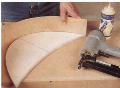
Figure 7: Use glue and staples (or brads) to attach two layers of bending plywood around the shape of the drawer bottom and top.
