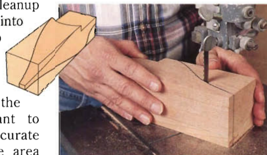
Figure 4: Make a template to transfer the shape of the feet to your blanks. Use your band saw to slice the curved shapes.
