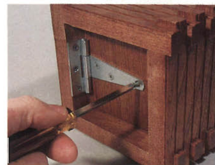
Figure 6: A T-shaped strap hinge automatically recesses the floor the correct distance from the bottom edges of the house.
