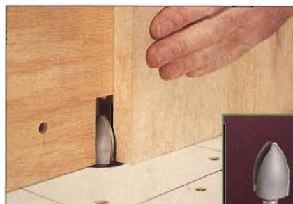
Figure 2: The rail ends are machined to fit into the grooves formed by the first cutter. Then use a raised panel bit (below) to shape both sides of the panels.
