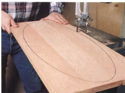
Figure 1: After tracing the oval shape onto your shelf blank, band saw the piece free. Then carefully sand to the traced line.
