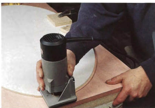
Figure 2: The offset collar is the key to this inlay template routing system. Rout one part with the collar on and the joining part without the collar ... you'll have two perfectly matching pieces.
