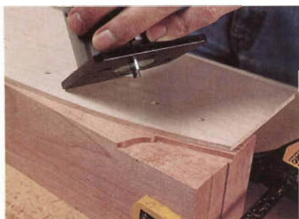
Figure 9: With a rub collar on your router, remove waste until a smooth drawer-lip is formed. Complete the corner notches on the band saw.
