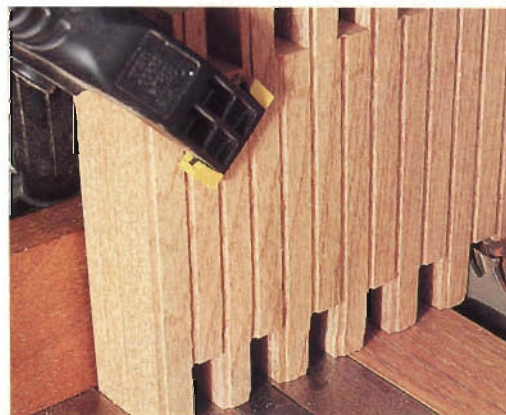
Figure 2: After crosscutting the scored sidewalls to size, form the corner joint notches, as shown at right. To reduce the number of passes, you can cut two walls at the same time.
