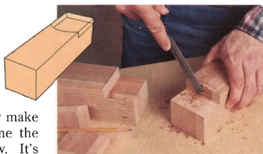
Figure 3: After cutting rabbets into the feet on your table saw, form their visible edge so they match the shape of the oval shelf.
