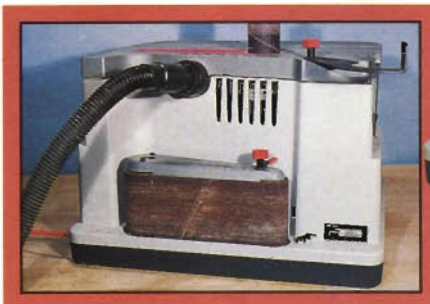
Storage for the large sanding plate and the drums is engineered into the body of the sander — a nice touch.
