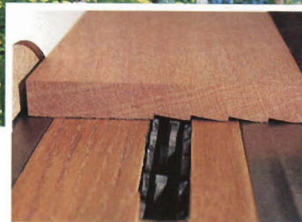
Figure 3: Rather than making many individual shingles, the author cleverly machines them into the roof sections with a dado head.
