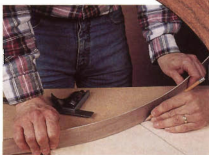
Figure 6: Strike a gentle curve for the drawer box top and bottom. A helper draws the line as you flex a strip to meet the three points.
