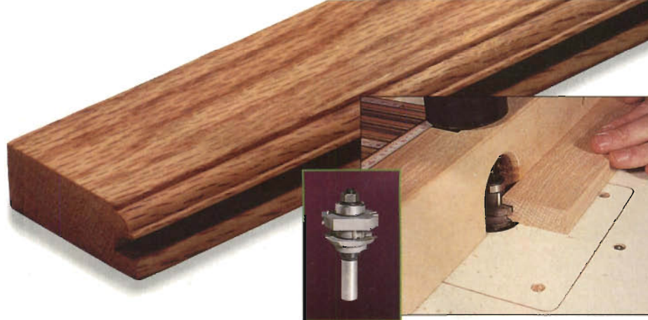
Figure 1: Stile and rail bits are the best way to create the mating joints characteristic of frame and panel construction. With your first pass you'll form a bead and groove.
