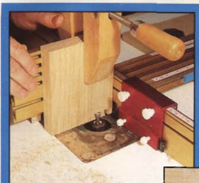
Milling through dovetails with the INCRA Jig Ultra system is a matter of aligning the jig with the correct template, then clamping two workpieces to a sliding right-angle fixture before making the cut.
