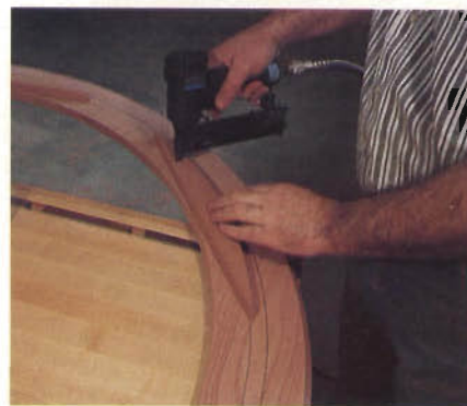
Figure 7: Glue blocks are used to help secure the top to the leg/apron subassembly. These blocks should be glued and nailed to the underside of the circular rim.
