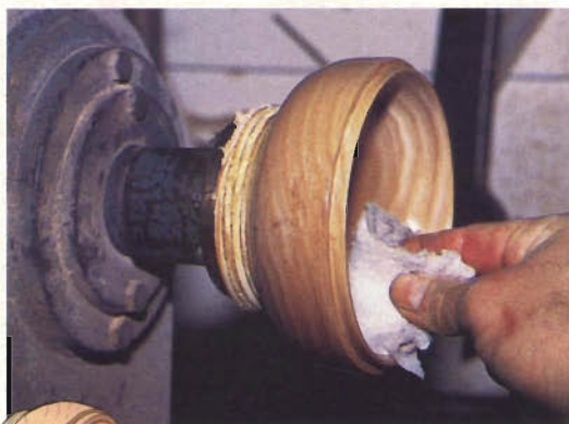
Figure 3: It's important to finish your project as you turn; it will minimize cracking and other moisture-related problems.
