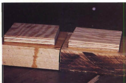
Figure 1: Glue 1/2" pieces of plywood to the hardwood blanks. They will be mounted to your faceplate with screws. The plywood will be removed later.
