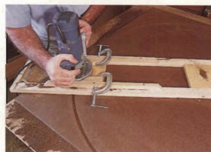
Figure 1: Use a circle cutting jig attached to your router to cut the hardboard top and bottom of the apron form at the same time.
