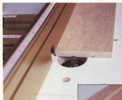
Figure 2: Rout the flutes in your stock before cutting it to length to ensure uniformity.
