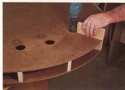
Figure 2: Using an extra spacer cleat as a guide, drill large clamp holes into the form to anchor your bar clamps during glue-up.
