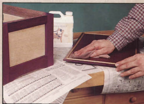
After the stain has dried and the box is assembled, an oil/wax wipe-on finish is applied. While not as durable as some final coats, its ability to bring out the warmth and richness of hardwood is unsurpassed.
