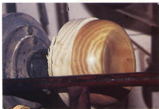
Figure 5: Use the lid blank as a ram chuck to reverse turn the concave bottom of the base. Then size the lid to the base's exact diameter. A very slick technique!
