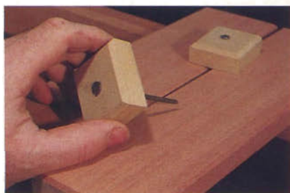
Figure 8: An 8d nail driven through a block of wood is useful as a spacer when attaching the table slats of the bench seat slats.
