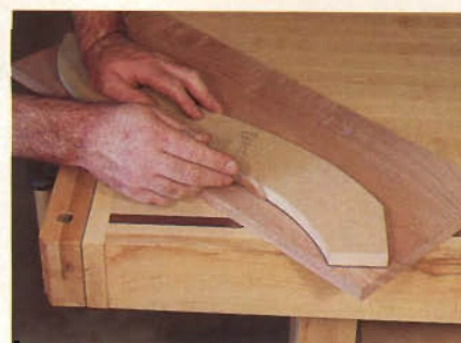
Figure 4: The stretchers of this table are curved to reflect the circular top. Create a template to ensure each piece is identical.
