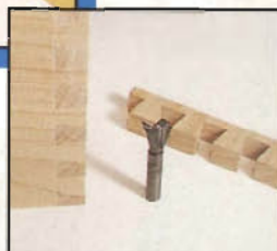
Milling through dovetails with the INCRA Jig Ultra system is a matter of aligning the jig with the correct template, then clamping two workpieces to a sliding right-angle fixture before making the cut.
