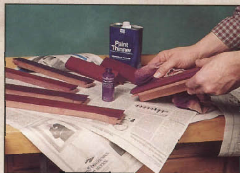
To preserve the vibrant color naturally found in purpleheart, the author applied a purple Woodburst™ stain. With this finishing approach, you stain the stiles and rails before assembly.
