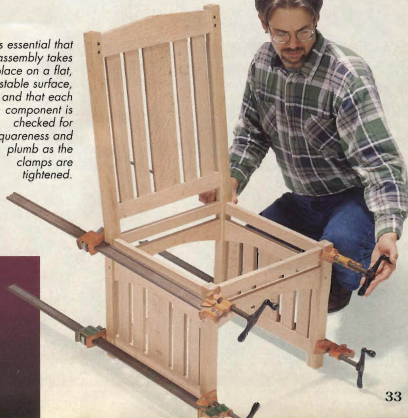
Figure 2: Glue up the subassemblies of the back and chair sides. Make sure they are flat and square. After the glue has cured, move on to the final assembly.
