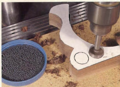
Figure 2: Use a Forstner bit to form the holes for the lead shot counterweight. After filling the holes with shot, pour a little epoxy over it to eliminate any trapped air.
