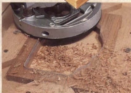
Figure 1: Remove most of the waste from the door opening with a scroll saw before routing with the first template: it makes for an easier cut with the top bearing pattern bit.
