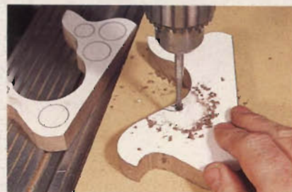
Instead of bullet catches, the smaller tape dispenser features a drilled and refined path for the tape core's axle pins.
