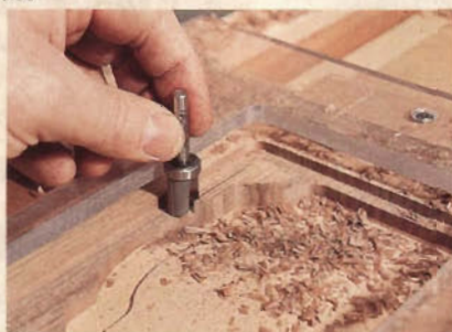
Figure 2: Using spacers with the second template keeps the bearing riding against the template while the cutter forms the rabbet for the glass and retainer strips.
