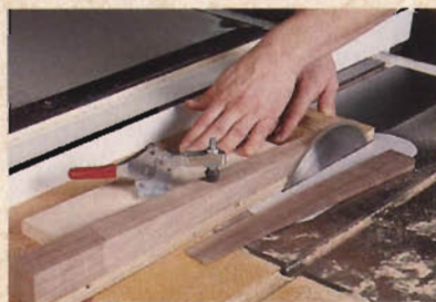
The nicely tapered legs on this classic design were produced using this simple jig.
