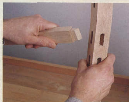
Figure 1: Mortise and tenon joinery is the key to this chair's durability. Different mortise locations create right and left chair parts. Some of the tenons are mitered to meet inside the uprights.
