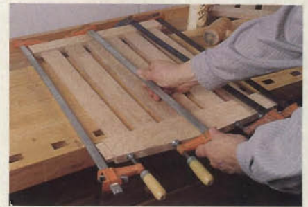
Figure 2: Glue up the subassemblies of the back and chair sides. Make sure they are flat and square. After the glue has cured, move on to the final assembly.
