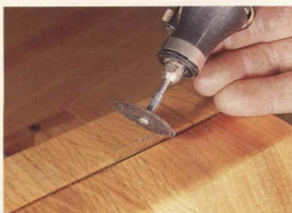
Figure 3: A rotary tool is perfect for forming the teeth on your brass tape cutter. Leave the protective plastic in place until you're done working the brass.
