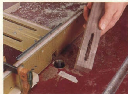
Figure 1: Floating tenons are a unique feature in this design. Use a stop block and masking tape to start and stop your mortises.
