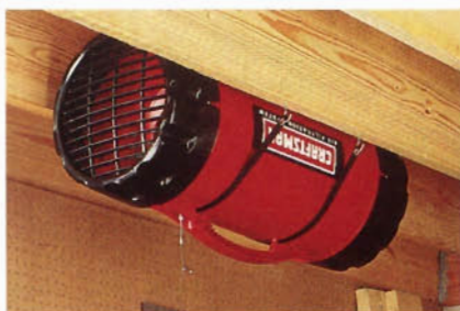
The Craftsman 16995 portable, two-stage filtration system comes with straps to mount it to the ceiling.
