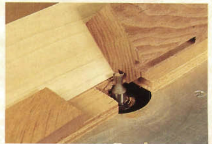
The leg joinery is formed in two passes. Use a straight bit to hog out the waste and then turn to a dovetail bit to complete the joint. A stop block limits the length of the cut.
