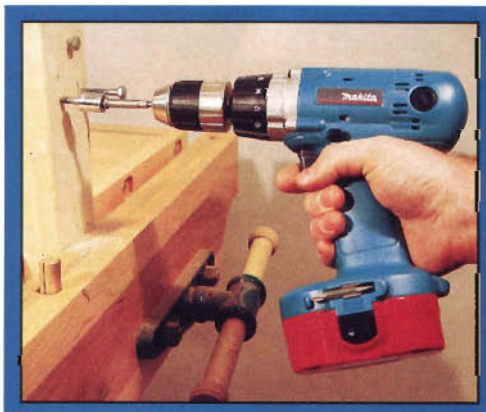
The 6343DWAE drill stood up to tests on several materials. Its 18 clutch settings allow the end-user to choose the amount of torque.
