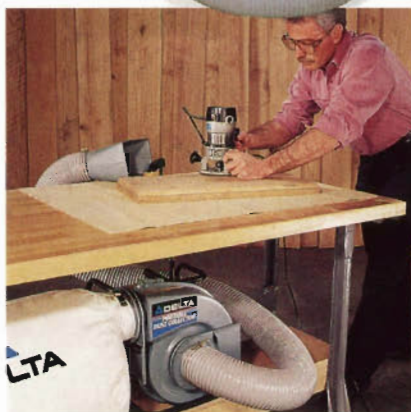
Portable collectors like Delta's 50-820 use a hood near the work area to gather dust from routing or sanding operations into a bag.
