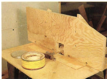
Figure 1: Use an 8" high fence on the router table when forming the dovetails. Be sure the fence is set at exactly 90°. A little wax helps keep the pieces moving smoothly as you cut.
