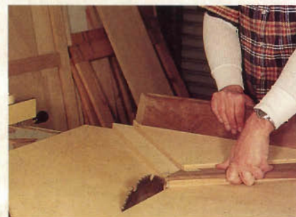
Figure 4: A sliding cutoff jig forms the miters at the ends of the table's frame components. Secure the miters with biscuits located in the remaining 3/8" thick stock.
