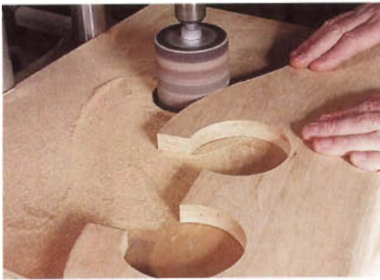
Figure 1: A broken pediment creates the crowning touch for this corner cabinet. Smooth its curves by using a drum sander.
