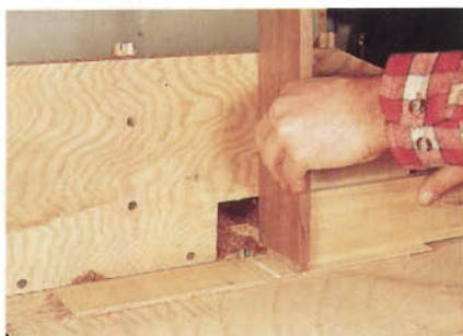
Figure 3: You'll have to switch to a straight bit to knock off the bottom of the apron's tails. Be sure to use a tall support block when trimming the bottom of the apron dovetails.
