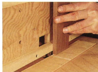
Figure 2: Slight bows could rock the aprons while the tails are being formed. I attached guide runners to my high fence to allow for any imperfection in the aprons.
