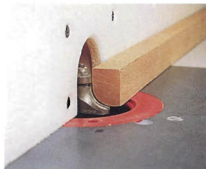
Figure 4: The outside edge of the large door molding is shaped on a router table with a 3/8" radius roundover bit.
