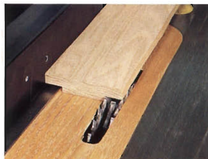
Figure 7: Use a dado head in your table saw to cut rabbets in the support bracket bases. Two support bracket sides will fit into the rabbets.
