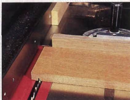
Figure 1: No need to set up a dado head: you can use a standard saw blade to make the small dados on the inside faces of the sides.
