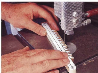
Figure 3: The full-size pattern on the center pullout makes machining the legs on the band saw a breeze. Follow up with a file.
