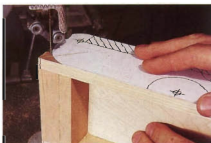
Figure 2: After gluing up the body parts, move to the Full-size Pattern to find the dimensions for shaping the cricket's end blocks.
