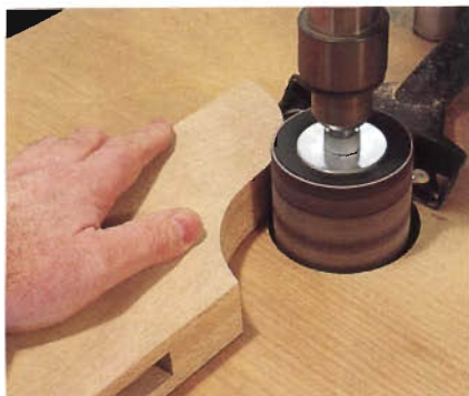
Figure 4: After cutting the glued-up tabletop supports to shape, drum sand the curved edges.
