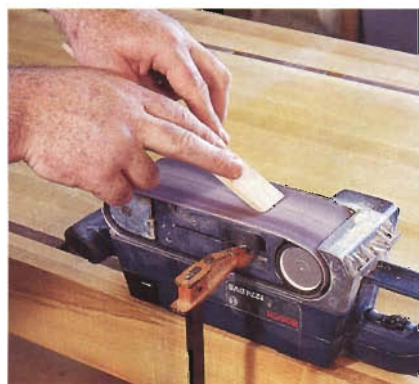
Figure 5: Give the solid cherry bumpers an authentic look by rounding over their ends on a belt sander before you glue them in place.
