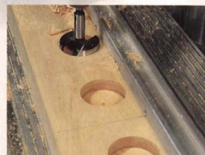
Step 1: Begin with a strip of 3/4" thick scrap, at least 3" wide. Use the Full-size Pattern at right to lay out and drill a series of 2" diameter holes in this stock.
