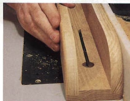
Figure 8: Create the screw slots in the cleat bases in several passes, raising the 1/4" bit 1/8" on each pass.
