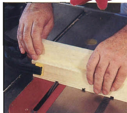
Figure 3: Clamp all four elements of the bus sides together to cut lined-up dadoes for the window dividers.
