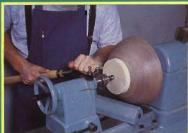
Turn the exterior to rough shape before mounting a face plate.
