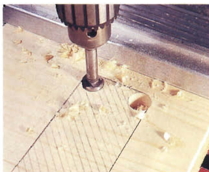
Figure 2: Use a Forstner bit to create smooth radii on the window and windshield corners, then complete the cutouts on a scroll saw.
