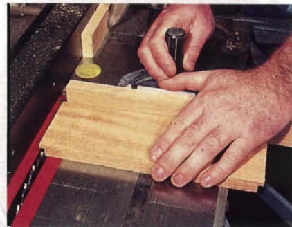
Figure 2: Tongues on the top and bottom fit into dado slots in the sides. Create them by milling rabbets on the opposing edges.
