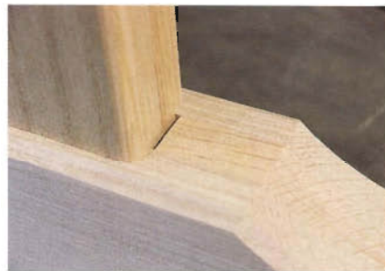
Figure 5: Leave 1/16" play on either side of the legs when you glue them into their mortises, to allow for wood movement. Leg moldings will eventually cover these gaps.
