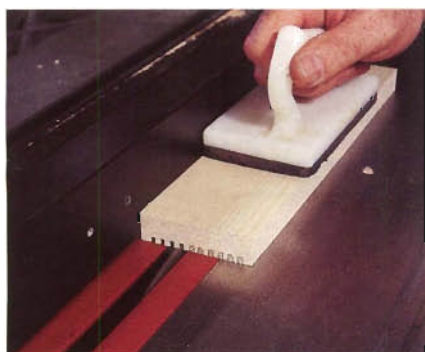
Figure 4: Use a zero clearance insert and a push stick to mill a long piece of stock for the grill, then trim it to size later.
