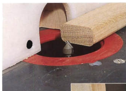
Figure 3: After rounding over all four long edges of the leg moldings, create two V-shaped glue control grooves in each back face.
