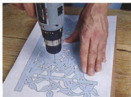
Figure 2: Use the smallest drill bit possible when drilling your fret blade insertion holes. This helps you to make the delicate vein-cuts.
