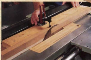
Use this safe, simple jig to cut accurate tapers on your table saw.
