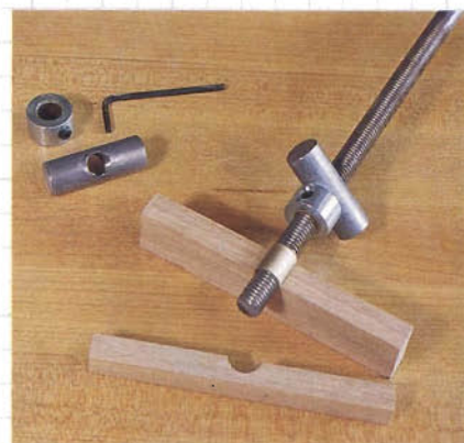
The operating hardware for this drill press vise is a double threaded spindle (allowing both jaws to be driven by a single handle) teamed up with spindle nuts and collars.
