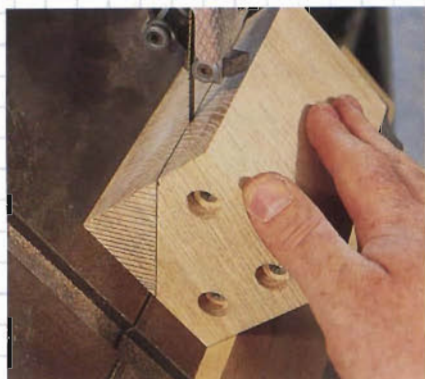
Figure 2: Use your hand saw to complete the laminated jaw's shape. See the Pinup Shop Drawings for all the dimension details.
