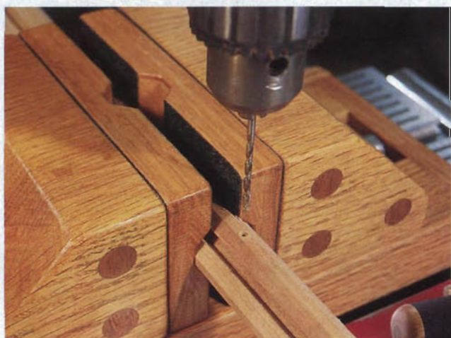
Use a single liner or both at once to effectively grip and secure a wide variety of moldings or other shaped pieces. Even difficult end grain drilling is made easy with the author's fixture.
