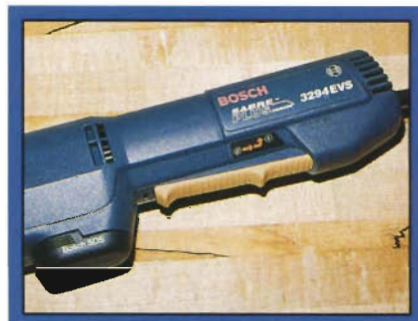
The paddle switch must be pressed backward and down 1/4" to reach full on. Built-in tabs help keep your fingers from sliding over the surface while operating the switch.
