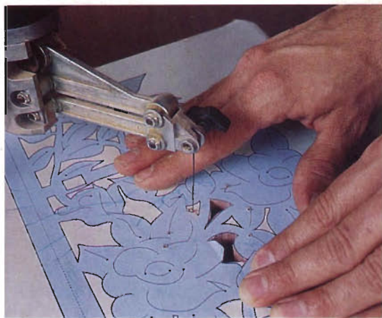
Figure 3: Stacking the two 3/8" pieces together reduces overall cutting time, but can present problems when waste pieces are freed up. Be sure to keep a steady hand as you reach the end of each cut.
