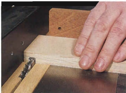
Step 2: Without moving the rip fence, switch to the miter fence to form matching dados in the drawer sides.
