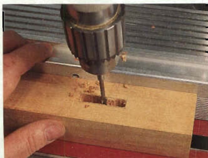
A Forstner bit chucked in your drill press will remove most of the waste, and the bit's design leaves a nice, flat-bottomed cavity.
