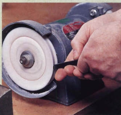
Polish the Ebon-X plugs and splines to their final luster with a polishing wheel mounted in a bench top grinder.
