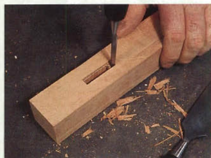
Clean up with a sharp chisel, cutting across the grain on the top and bottom first, then with the grain along the sides.
