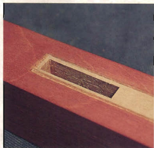
Figure 1: The author recommends tiny v channels around the perimeter of the joint area to help prevent glue squeeze out.
