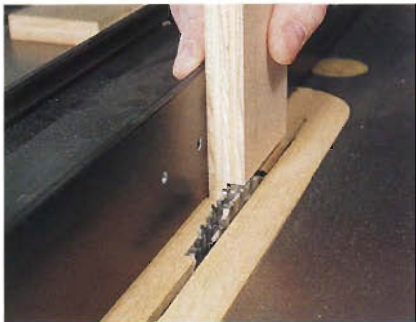
Step 1: Install a 3/8" dado head and a zero-clearance insert in the saw and cut a rabbet at the end of each drawer front and back.
