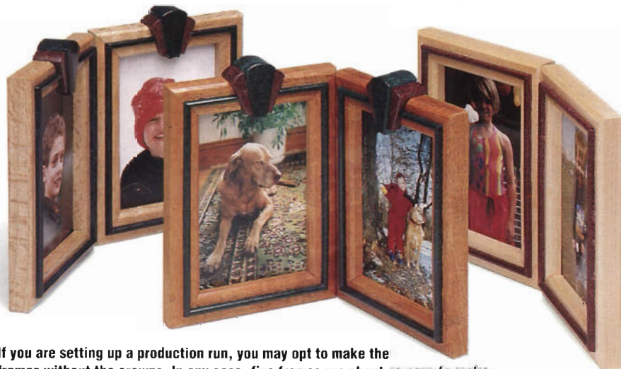
Figure 3: To add a little drama, a dovetail shape is formed at the top of each frame to accept the accents. These cuts can be made on the table saw with your miter gauge set first at 22½° to the left and then to the right.
