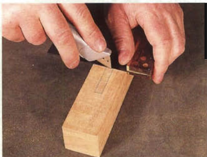
After laying out the matching mortises in the legs, score them with a sharp utility knife to avoid tearout as you drill.
