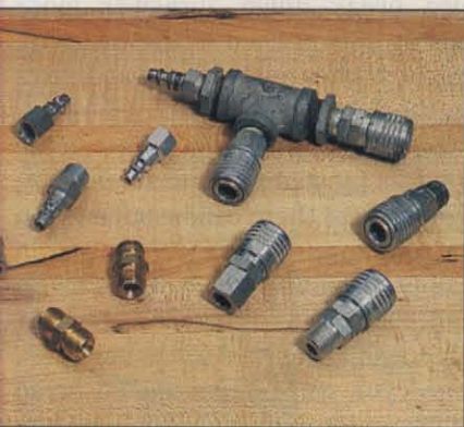
Photo E: Quick couplers and connectors make it easy to connect and disconnect tools and hoses. Several types are available, so make sure yours match.
