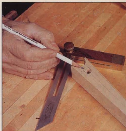
Photo H: Lay out a flat in the \frac{7}{16} " hole, then square-cut it to hold a \frac{1}{4} " hex nut securely.
