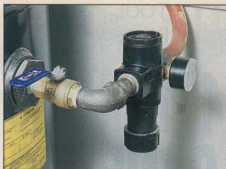
Photo F: Pressure regulators help maintain constant air pressure and also let you set the optimum operating pressure for the particular tool in use.
