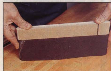
Photo E: Compress the springs to start the belt on the block, then simply slide it on the rest of the way.
