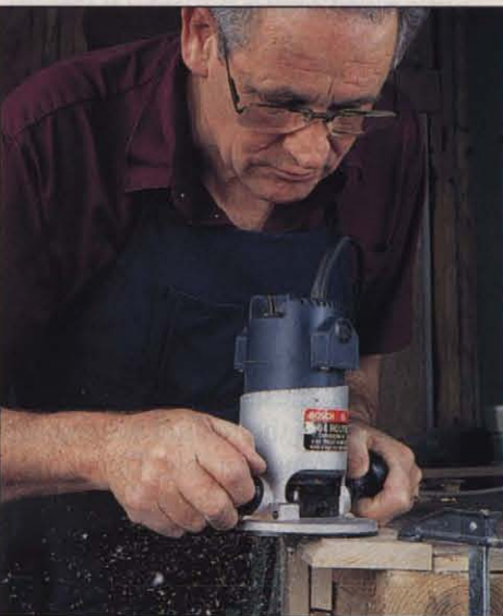
Photo B: Rout edge of top molded layer with 1/2"-radius beading bit (or a round-over bit with an undersized bearing).
