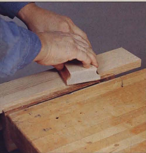
Photo A: The coved edges on this quarter-sheet sanding block help keep the abrasive tight.
