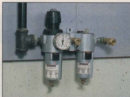
Photo G: Campbell Hausfeld's in-line control incorporates a filter, regulator, and lubricator kit. Filters protect air-powered tools by removing water and other contaminants.
