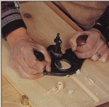
Photo L: The router plane excels at cleaning up the bottom of a machine-cut groove or dado. Cutter depth is adjusted by screw feed and can be placed on either side of the post.
