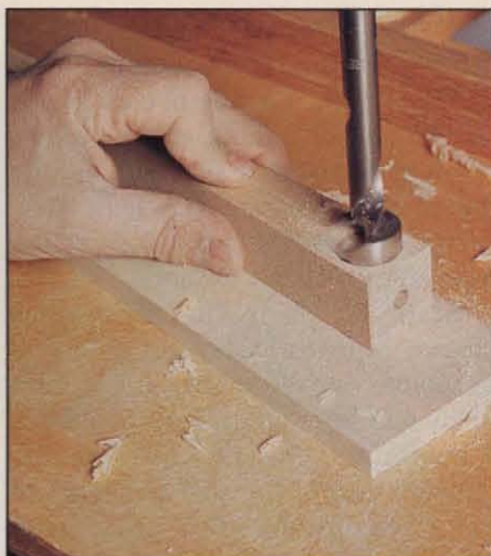
Photo G: To prevent tearout when drilling the 1" hole, use a backing block.
