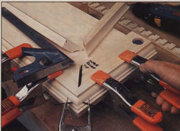
Photo C: Assembled first molded layer shows relief cut at miter and expansion screw at back end of side piece.
