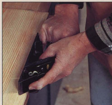
Photo D: To complete the rabbet, lay the plane (a filister shown here) on its cheek on the rabbet bottom and trim the shoulder until you shave off the layout line.
