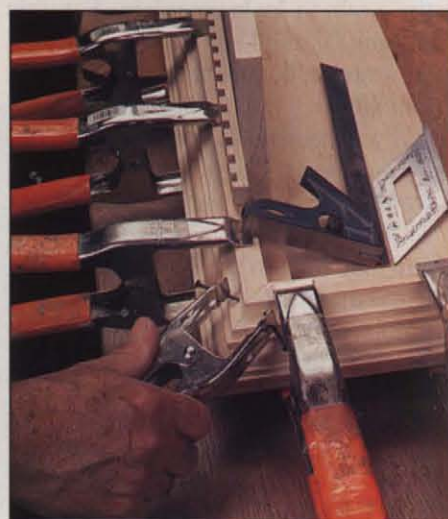
Photo D: The grain lies parallel on coved and beaded layers, so coved layer assembly does not require expansion joints.
