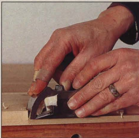
Photo F: Use a bullnose plane to finish a stopped rabbet right up to the stop. To produce a straight cut, author uses two hands, applying firm pressure behind the blade.
