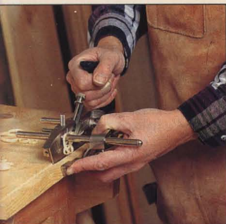
Photo N: To avoid alignment problems with the plow plane, apply firm pressure to the fence with the forward hand and start the groove carefully with a shallow, full-length cut.
