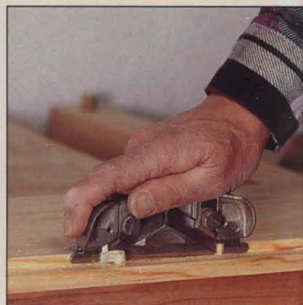
Photo G: Because of its short body and tricky setup, author generally uses the side rabbet plane only to trim limited areas along the shoulder line.
