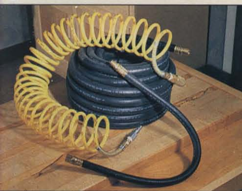
Photo D: Buy the largest-diameter air hose you can afford. The black coil is Sears' new 1/2"-i.d. high-performance rubber with 3/8" male/female connectors (catalog no. 16205). The yellow, self-coiling nylon air tube (catalog no. 16220) carries a 200-psi working pressure, an 800-psi burst-strength rating. The 2'-long 3/8"-i.d. leader (catalog no. 16207) has a 300-psi working pressure and 1200-psi burst-strength rating.
