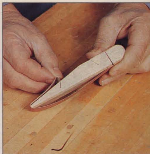
Photo N: While depressing the spring-loaded head with one hand, insert the free end of the abrasive strip into the second slot.
