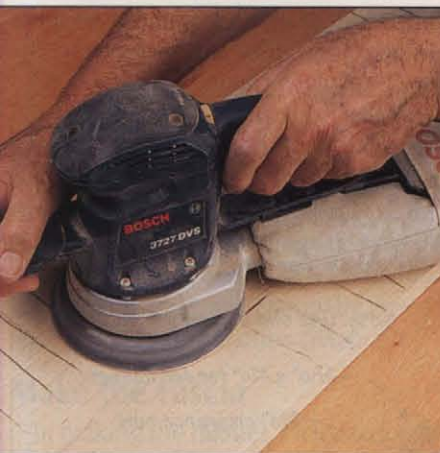
Photo A: To minimize blotchy finish, "deep-sand" the stock after planing to remove about .01" of material. This removes mill marks, torn and compressed grain.
