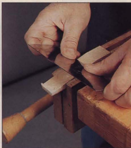
Photo M: Hand-plane or scrape the taper's face to smooth it.
