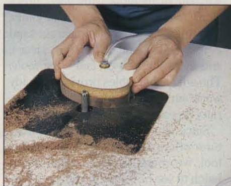
Photo H: Compressed air passing through a venturi generates enough suction to clamp the workpiece to this router template.
