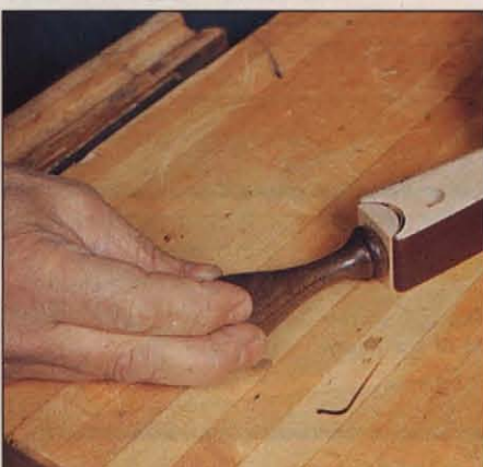
Photo J: Tightening the handle secures the abrasive strip to the sanding file.
