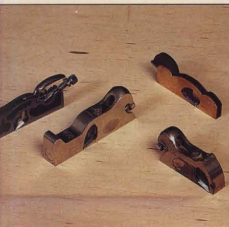
Photo H: Group portrait of shoulder planes: low-body (left) conventional (center), thin-body (back right), bullnose (front right).
