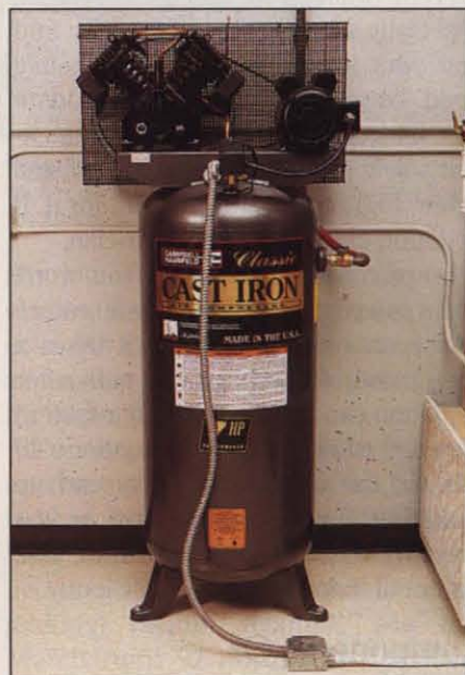
Photo A: The Campbell Hausfeld stationary compressor we installed in our shop is an oil bath-lubricated, piston-type unit.
