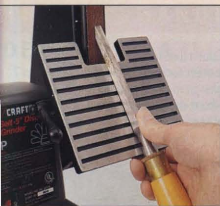
Photo A: For sharpening, the belt table must tilt to at least 65°, or you can use a wooden block machined to the proper angle.
