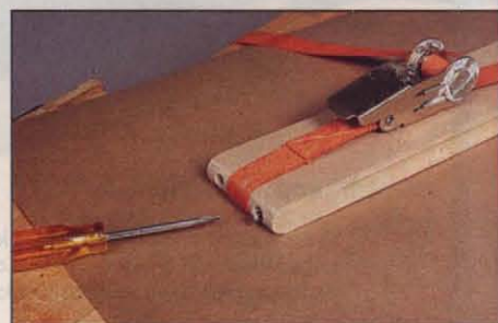
Photo D: Use a band clamp to compress the springs and hold the parts together while you drive the screws.
