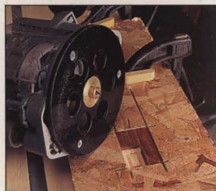
Photo A: To rout the window-frame openings, make an insert for your window-routing template.
