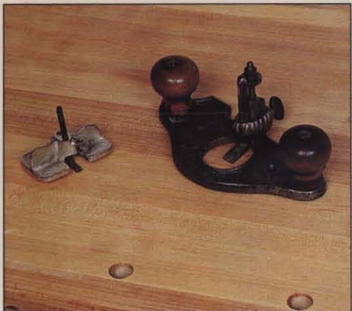
Photo K: A full-sized and a miniature router plane. Throat of the miniature can be used either open or closed so it's ideal for fine work and cabinetry.
