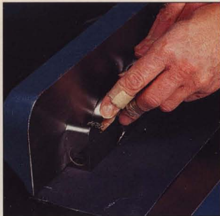
Photo I: Lap the sole of an out-of-square shoulder plane using a trued jointer or table saw fence and silicon-carbide sandpaper. Work from coarse through medium to fine grit.
