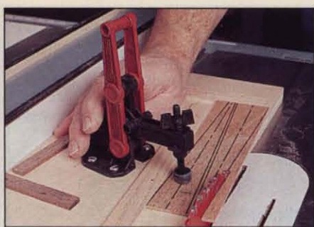
Photo C: Taper one edge of roofing blanks using two fixtures (one for each size), then turn blanks end for end, and (without the fixture) rip the second edge parallel to the tapered edge.
