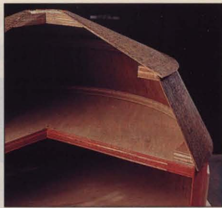
Photo G: Assembled barn and roof (without cupola) shows careful alignment of roofing and siding with cutaway rings, crown disc. Note slight overhang of roofing at eaves and hip.
