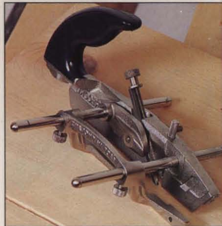
Photo M: The complex-looking plow plane, with its integrated fence, depth stop, and assortment of blade widths, was designed to replace a battery of wooden planes.
