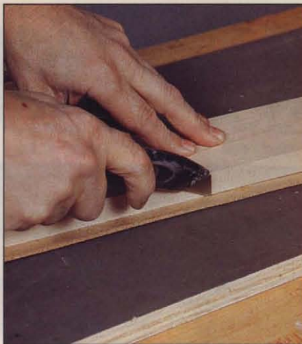
Photo B: Use a backing board and sharp knife to trim the excess cork from the blank.
