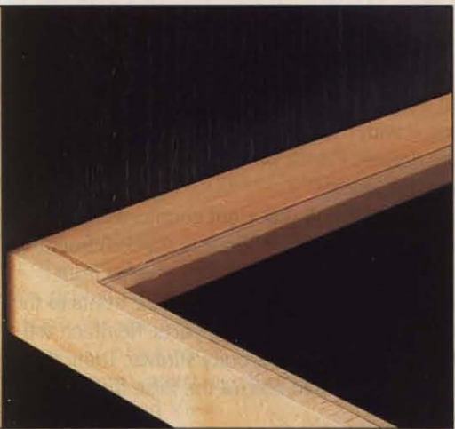
Photo A: Shelf frames are pocket-screwed and glued together, then rabbetted along the top inside edge to accept the plate glass. A small bead of silicone caulk holds the glass in place.
