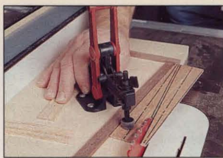
Photo D: After tapering both edges of the roofing blanks, make a third and fourth fixture to cut each blank size into identical halves.
