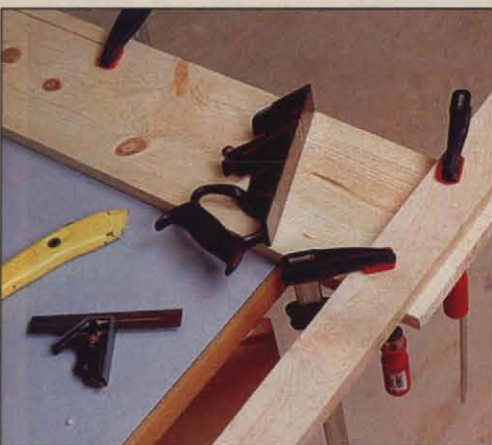
Photo E: Guide rail for cross-grain rabbeting extends well past the board's edges to give better control of the plane. Align guide edge exactly over (not beside) the scribed shoulder line.
