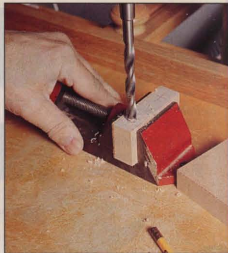
Photo C: To ensure a perpendicular hole, clamp the parts firmly to the drill-press table.
