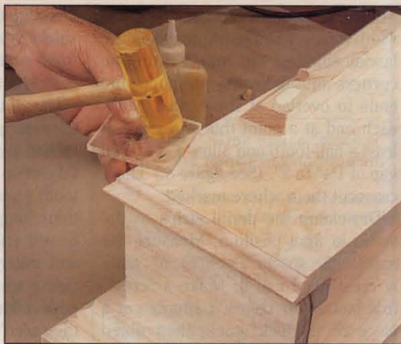
Photo J: To protect parts from the mallet and prevent plugs from going in too deep, author uses a scrap of ¼" sheet acrylic.
