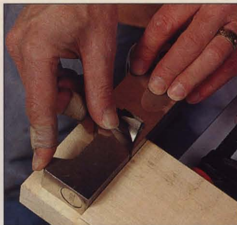
Photo J: To trim a tenon shoulder with a shoulder plane, clamp a backing board to the exit side and make very fine, full-length cuts along the sawn shoulder line.
