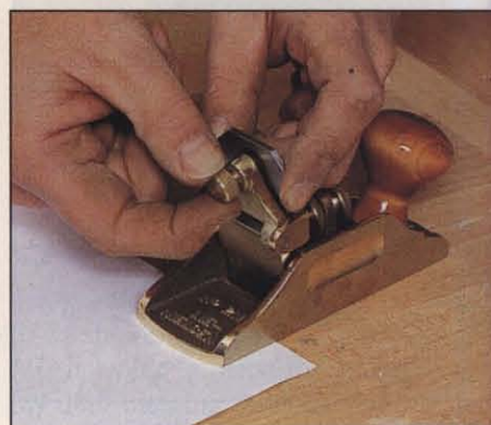
Photo N: Use a piece of paper to set the depth of the blade on a scraper plane.
