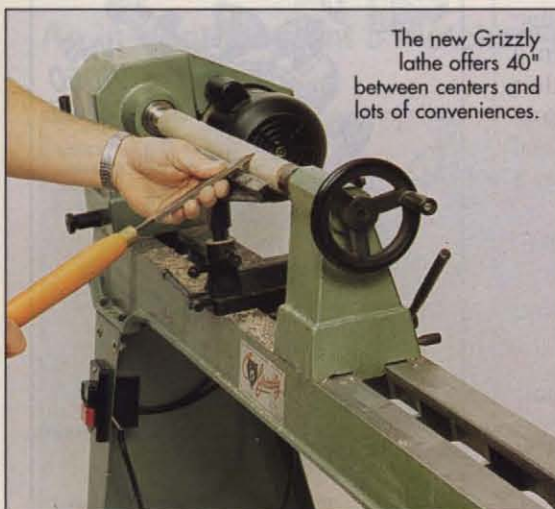
For outboard turning, the headstock swivels 180° and can be positioned at any point along the length of the bed.
