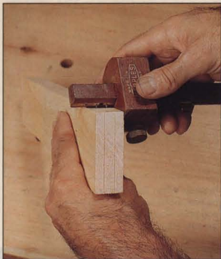
Photo D: Set the mortise gauge's double pins to desired tenon thickness, then set the fence to center tenon on rail edge. Starting at the shoulder line, scribe the cheeks up one edge, across the end, and down opposite edge.
