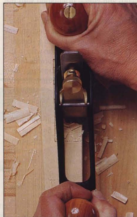
Photo J: The butt mortise plane can shape up hinge mortises faster than a router in many cases.
