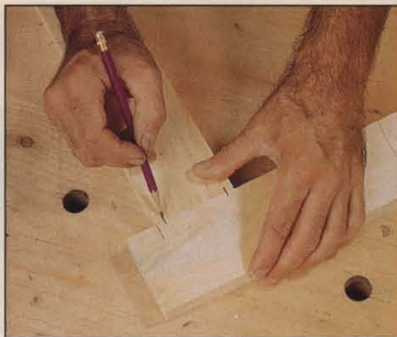
Photo E: Position the rail where it will join the stile, then mark mortise/tenon width onto stile directly from rail about \frac{1}{4} " in from rail edges.
