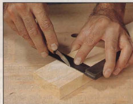
Photo C: Scribe the tenon's shoulder lines using a sharp knife and a square held against the rail's working edge. Make tenons \frac{1}{16} " shorter than the mortise depth.
