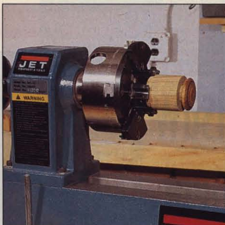
Photo B: The headstock has 1"x8 threads which accommodates a standard 3" faceplate and similar full-sized lathe accessories.
