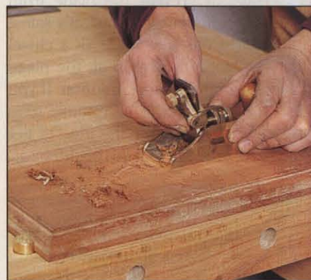
Photo M: When faced with wild or unruly grain, the scraper plane is the tool of choice to prevent tearout.
