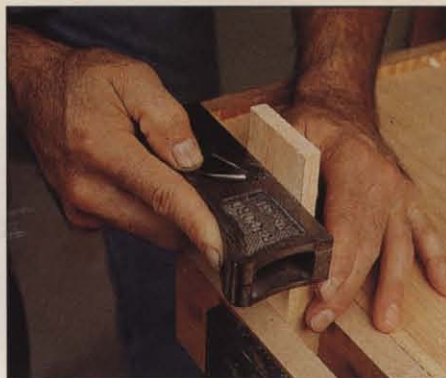
Photo T: A shoulder plane works great for final-fitting the tenon cheeks and shoulders.
