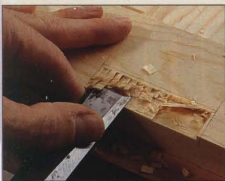
Photo O: Pare away scored waste, working down to depth line scribed on rail edge. Carefully extend mortise to its full length and width.
