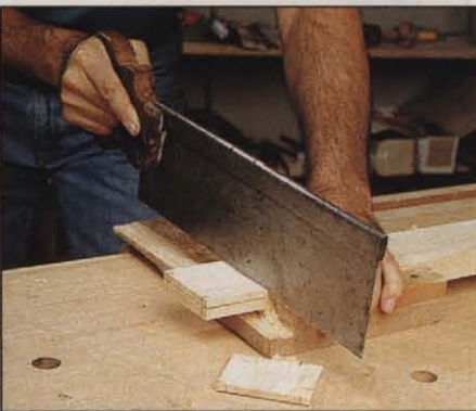
Photo N: Cut the shoulder to the knife line, starting at an angle on the far edge and gradually lowering the saw across the rail's full width. A bench hook steadies the rail.
