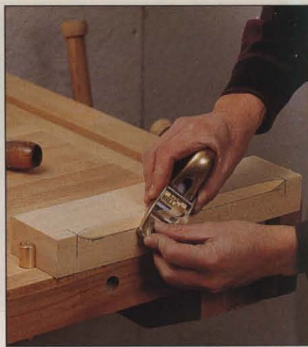
Photo F: Final paring on the chamfer is done with the block plane.
