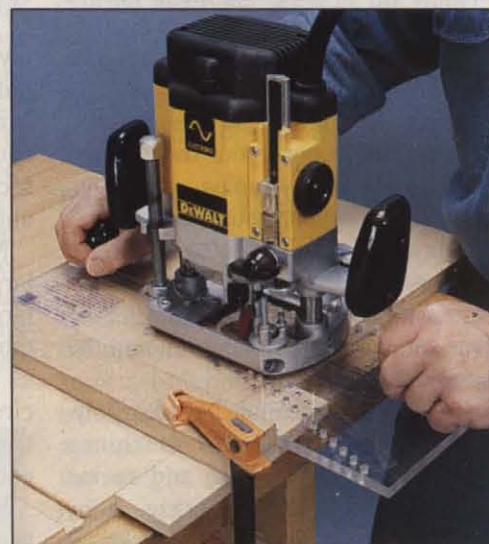
Photo C: The PowerPlate, used here as an extended base, enables a router to perform eight different routing tasks.
