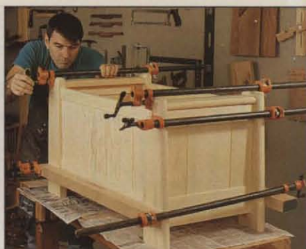
Photo K: Clamp up chest, then check for square. If necessary, adjust clamp positions slightly to help square chest.
