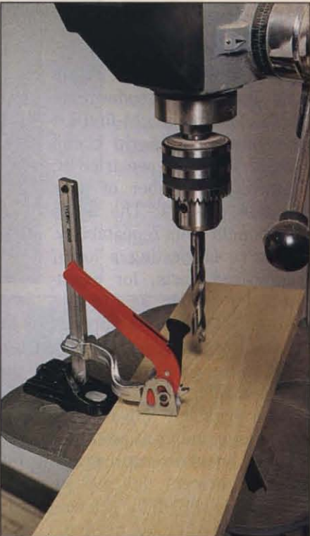
Photo D: Wilton's T-slot speed clamp with its off-set ratcheting lever (catalog no. 6906) adapts to tools with slotted tables or drilled bases.
