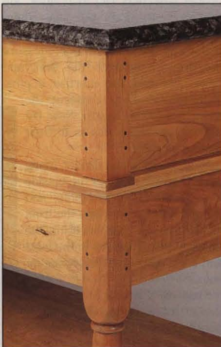
Photo D: Walnut dowels pin the side-panel tenons in the leg mortises.
