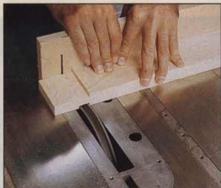
Photo S: If you don't own a bandsaw, you can cut the tenon cheeks with a dado head, although this is less accurate because it prevents you from indexing the tenon from the working face.
