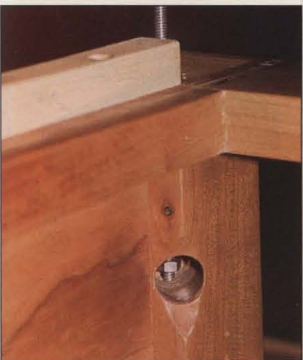
Photo A: Threaded rods hold the four case corners together. Each rod passes through the upper leg and divider frame and fastens to a nut and washer recessed in the lower leg.
