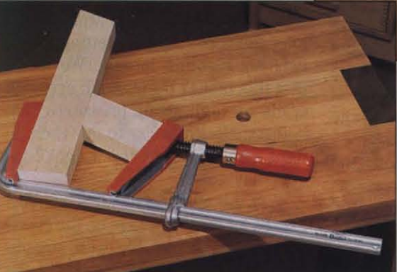
Photo B: Both jaws on the Bessey Flex K (catalog no. FJ4.016) angle up to 10° in two directions—ideal for holding miters and irregular-shaped parts.
