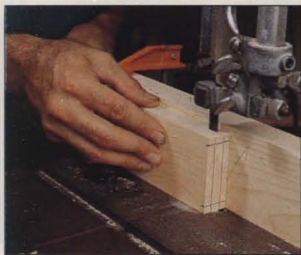
Photo P: Bandsaw the far cheek first, then the one closer to the fence. Reset the fence for each cut so the working face always bears against the fence.
