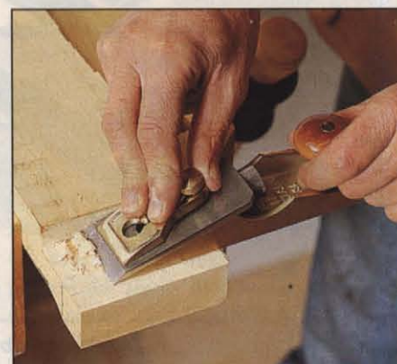
Photo H: Nothing can get you closer than a chisel plane, shown here trimming the cheek of a large lap joint.
