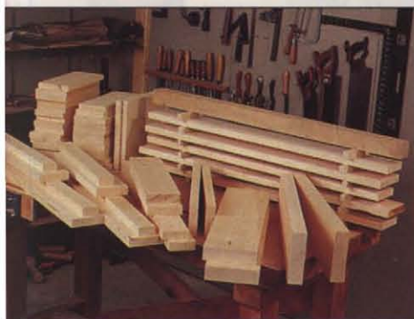
Photo A: Group the legs, rails, and stiles, and keep them together throughout the construction process to reduce confusion.
