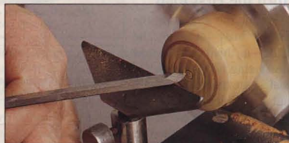
Photo J: Scratch shallow decorative grooves into the face.
