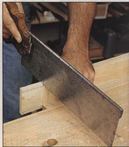
Photo O: With the cheek waste cut away, mark the tenon width using a pencil marking gauge. Make the long-grain cuts, then cut along the knife lines on the edges to form the short shoulders.
