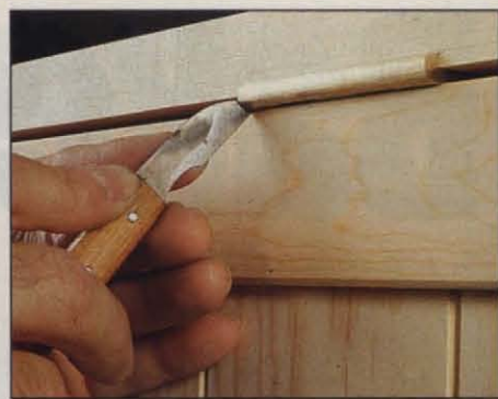
Photo Q: With lid sized to fit snugly in its opening, use a knife to transfer hinge locations from lid to chest rail, then lay out and cut chest mortises. Resize the lid for easy opening after installing hinges.
