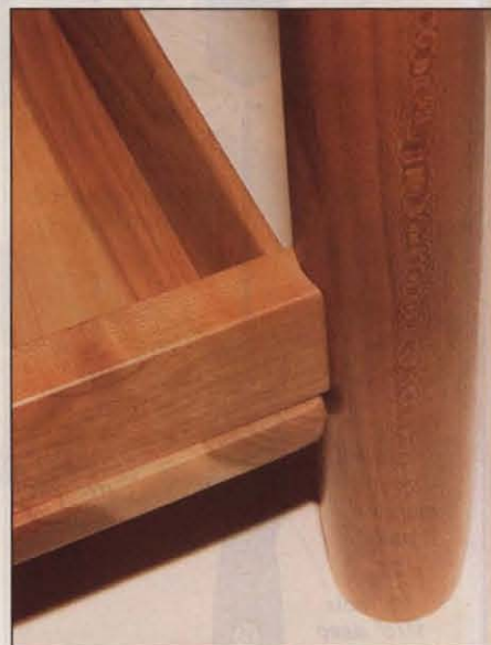
Photo B: Author sanded the ends of the shelf stretchers with a drum sander to fit them to the turned-leg profile.
