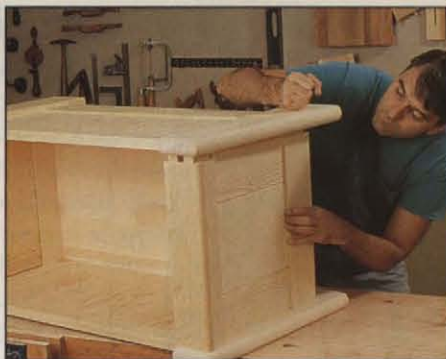
Photo J: After gluing side rails to the back assembly, insert bottom panel and side slats in their grooves without glue. Then, glue and assemble front to side rails.
