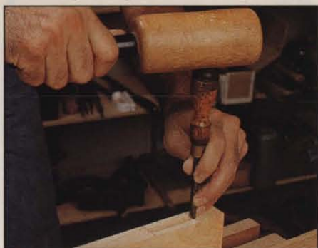
Photo J: Use a narrow chisel to square the mortise ends. When end grain offers resistance, author uses a mallet.
