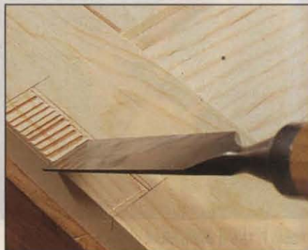
Photo N: Score the waste to within \frac{1}{16} " of mortise ends and edge, holding chisel at an angle so depth decreases toward inner edge. The leaf should align flush with rail face at this edge.
