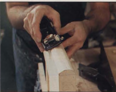
Photo F: Use a sharp block plane to round the top end and outside edge of each leg, taking care to keep a crisp arris where the round meets the face. Round the leg edge after assembling the front and back so you'll have a square edge for clamping.
