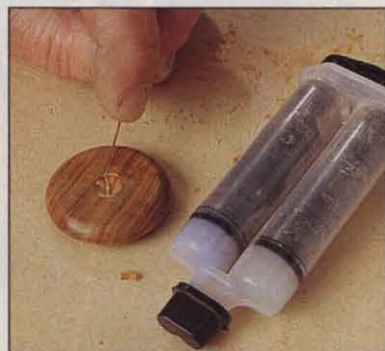
Photo R: Epoxy the hardware in place.
