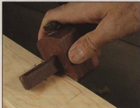
Photo L: To lay out hinge mortises, use two marking gauges if you have them—one for width (on face), one for depth (on edge).
