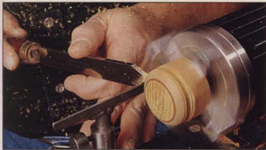
▲ Photo K: Turn a 1/2"-deep groove at the point where you'll later part the piece from the stock.
