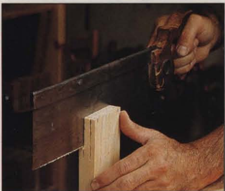
Photo M: Using the angled saw kerfs as guides, cut both tenon cheeks to the shoulder line holding the saw perpendicular to the rail.
