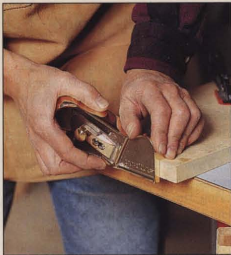
Photo D: The edge trimmer's fence guarantees a square edge.
