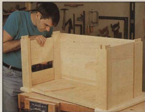
Photo I: Dry-assemble all parts to verify that joints fit properly. Do a "dry run" to make sure you have clamps, pads, and other supplies arranged where you'll need them.
