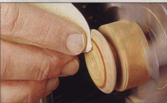
Photo M: Sand all surfaces to 320-grit with the lathe spinning.
