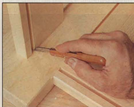
Photo G: To lay out bottom groove on leg, first dry-assemble the side bottom rail to the front/back assembly, then use a knife and straightedge.
