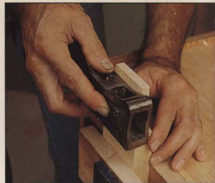
Photo U: To square tenon shoulders, work from both edges inward to avoid splintering the rail edges.
