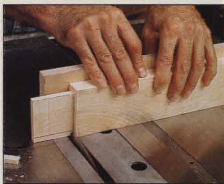
Photo R: After laying out and bandsawing the tenon to desired width, remove waste by cutting the short shoulders on the tablesaw.
