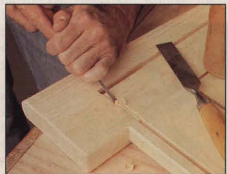
Photo H: Author uses sharp chisels to cut cross-grain bottom groove on leg.
