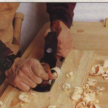
Photo I: The scrub plane looks like a narrow-bodied Jack plane with a large mouth opening but without a cap iron.
