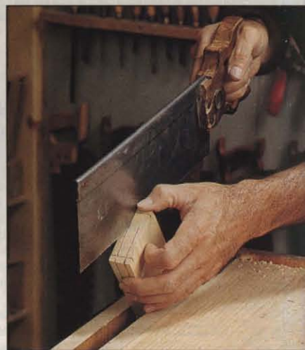
Photo L: Start each tenon cheek by making angled cuts from both corners. When completed, each cut should extend from the shoulder line to the midpoint of the rail end.
