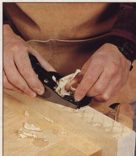
Photo C: Author demonstrates the proper block plane technique: two hands in control and the plane at a slight skew.
