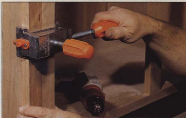
Photo G: The two-way Pony Cabinet Claw draws cabinet face frames together and aligns them for accurate shank-and pilot-hole drilling.
