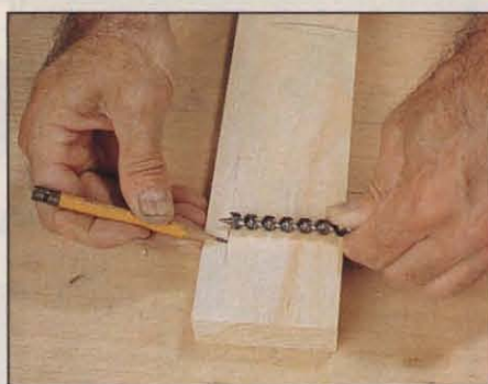
Photo B: When establishing mortise depth on the stile, make sure the waste-clearing bit's lead point won't penetrate the workpiece's opposite edge.
