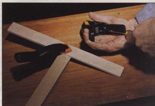
Photo A: To adjust clamping pressure from 1 to 50 lbs. on a Pony Adjust-a-Clamp, simply turn the screw located inside the clamp.
