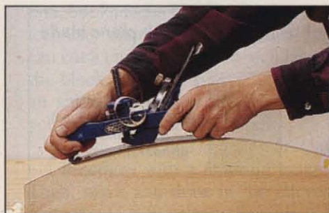
Photo L: A compass plane has an adjustable sole that enables it to cut a true radius. For good results, make long, shallow cuts.
