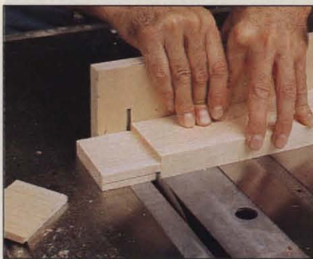
Photo Q: Cut the shoulders on the tablesaw using a miter gauge with a wooden extension. The extension provides extra support for accuracy and also backs the cut.
