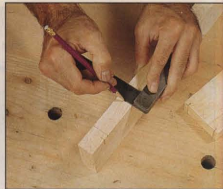
Photo F: Square the mortise lines across stile edge to establish mortise ends. Sharp pencil lines are accurate enough for these marks.
