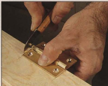
Photo M: Since hinge leaves often are not cut perfectly square, use actual hinge to mark ends of mortise. Mark hinges and mortises to pair them.
