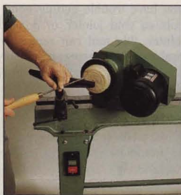
For outboard turning, the headstock swivels 180° and can be positioned at any point along the length of the bed.
