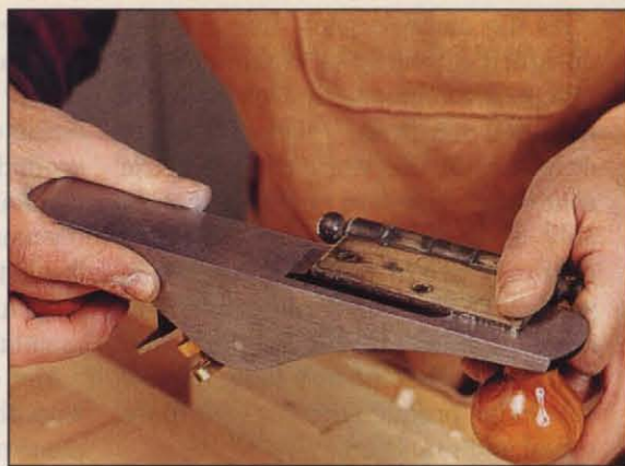
Photo K: Set the depth of the blade on a butt mortise plane by gauging it against a leaf of the hinge.
