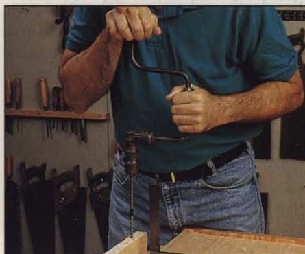
Photo H: To clear waste, use a bit slightly smaller in diameter than the mortise's width, boring at the mortise ends first. Note the square used to help the author keep the bit vertical.
