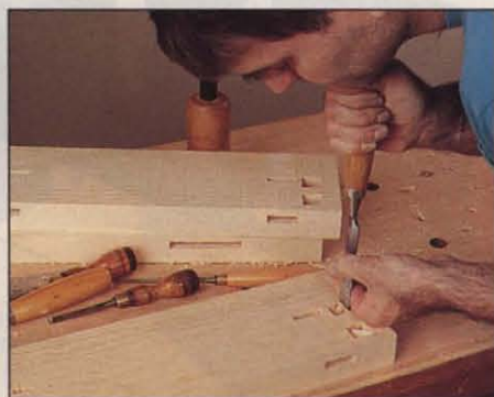
Photo B: For accuracy, index all mortises from the "working" face and edge of the leg. Lay out the mortises on one leg, then transfer the layouts to each of the remaining legs.
