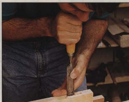
Photo K: For the final paring, place the chisel edge in the scribed lines you deepened earlier and clear the last traces of the auger-bit holes.
