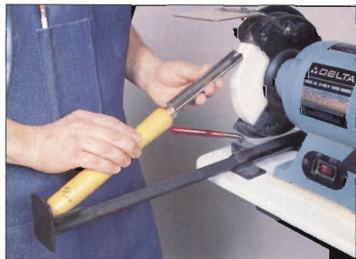
Photo A: To sharpen gouges, use the Vee-arm to support the tool at the proper angle to the wheel.
