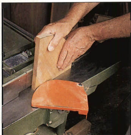
Photo C: Set jointer to remove only \frac{1}{64} " of stock, then joint straight edges to the line.
