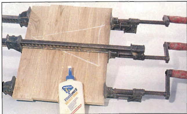
Photo A: Edge-glue clear, straight-grained pieces to form the blank, arranging the pieces for best grain and color match. Note the clamp placement and ideal amount of glue squeeze-out.
