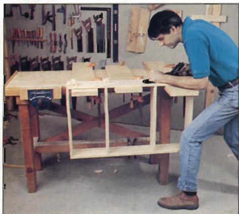
Photo L: Plane the joints flush with the exterior faces. To support the case for planing, author cantilevers three boards from his bench.
