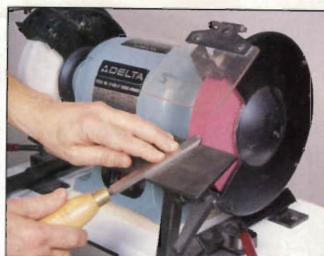
Photo C: The large surface on the adjustable-angle platform provides plenty of support for sharpening scrapers, chisels, or plane irons.
