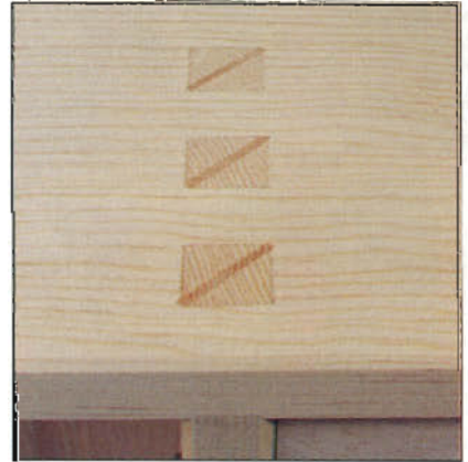
Photo H: This detail of the completed cabinet shows the through-wedged tenons (planed flush) and \frac{1}{8} " chamfers on both the inside and outside front edges.
