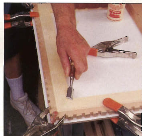
Photo I: Glue and pinch-clamp dentil layer, then scrape off squeeze-out and sand or plane joints level if necessary.
