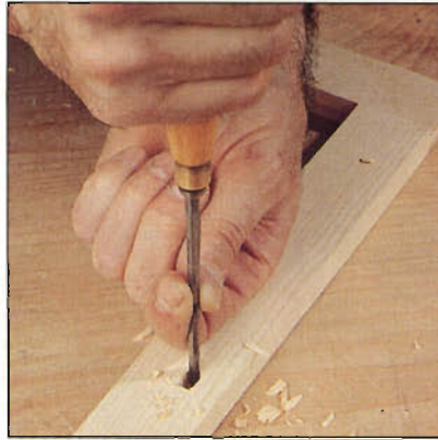
Photo V: Mortise the door stile to accept the knob tenon. This joint ensures a much more permanent attachment than fixing the knob with a screw.
