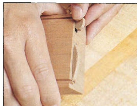
Photo B: The box miters take a #0 biscuit. The lid miters require a miniature version.
