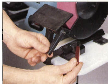
Photo E: Lever-actuated cam clamps lock the Vee-arm and the adjustable-angle platform to their bases.
