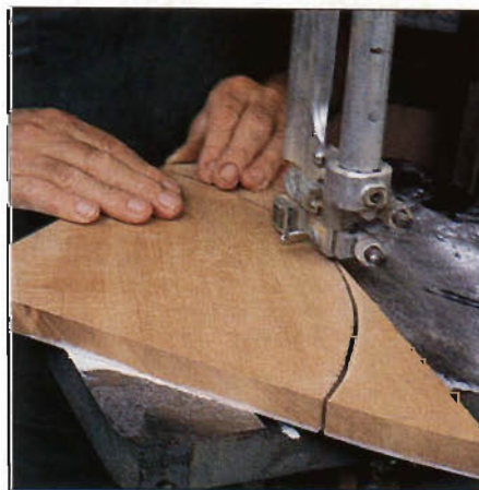
Photo B: Bandsaw shelves to shape. Depending on your jointer's performance, you may want to joint the straight edges before bandsawing the curved front edge.
