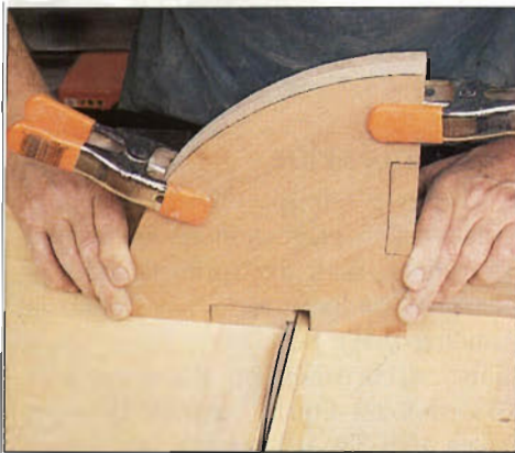
Photo F: Use a sliding crosscut saw table or miter gauge with extension to cut shelf notches. Size notches to fit support width and depth, sneaking up on final dimensions. Cut both shelves at the same time.
