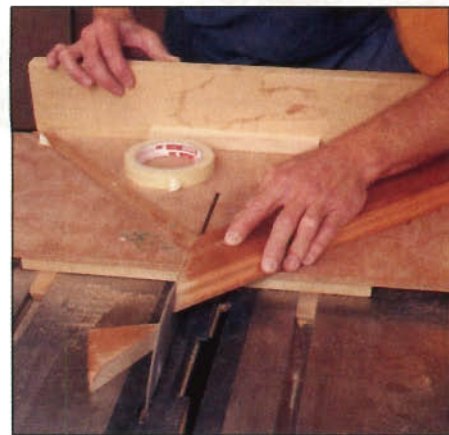
Photo F: To miter stock, author uses shop-built jig that cuts opposing miters and handles long workpieces. Note use of masking tape to fine-tune the fence angle.
