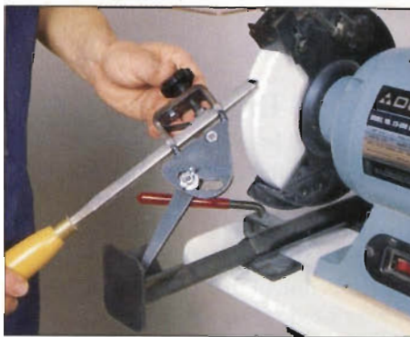
Photo B: The Vari-Grind attachment used with the Vee-arm makes it easy to grind a sharp, even profile on deep-fluted bowl gouges.
