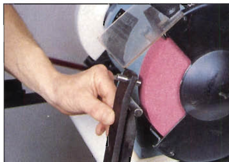
Photo D: Dressing either grinding wheel is quick and accurate using the diamond wheel-dressing attachment.
