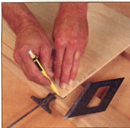
Photo E: To lay out miters on bottom (Roman ogee) layer, align template on stock for \frac{1}{4} " offset, mark template corners, then use an accurate 45^\circ instrument to extend cut lines to front edge of stock.
