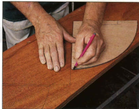
Photo A: Lay out triangular shelves so the grain runs across them, flip-flopping the template to conserve stock.
