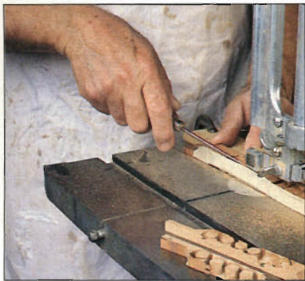
Photo H: Cut plugs in over-thick blank, then resaw the blank to make plugs \frac{1}{8} " longer than counterbore depth. Author applies masking tape before resawing to keep plugs together.
