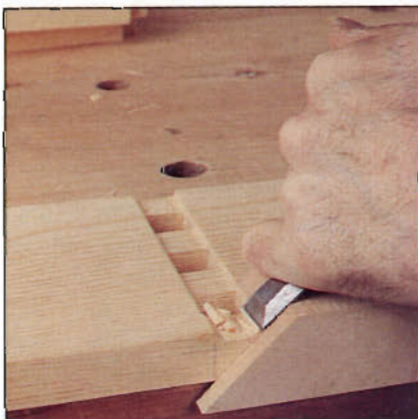
Photo F: Miter the shoulders in the front section of each dado using a chisel and 45° template. Clamp the template in place and take thin cuts until the chisel rests flat on the template.
