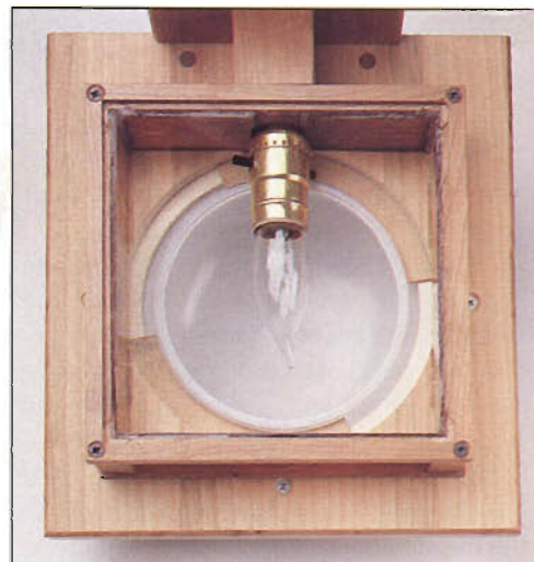
Photo A: Top view of the assembled scone without the glass cover. Note placement of the globe retainers, stained-glass panes, and light socket.
