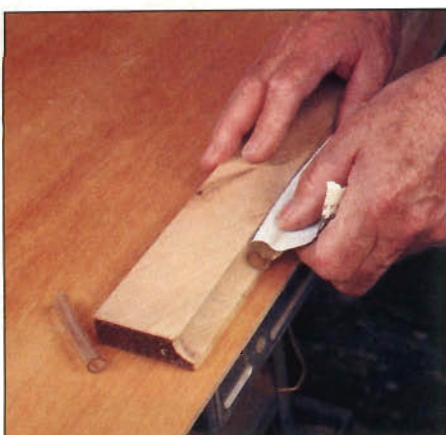
Photo D: Sand the routed profiles to 180-grit before mitering the stock to length. Here, author wraps abrasive around vinyl tubing to sand covered profile on top (fourth) layer.
