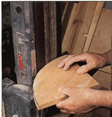
Photo D: Using a stationary belt or disc sander, sand curved shelf edge to the line.
