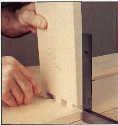
Photo C: Cut tenons on the dividers, then align the front faces of the parts and carefully knife the mortises on the dadoed (inside) face of the top/bottom directly from the tenons.
