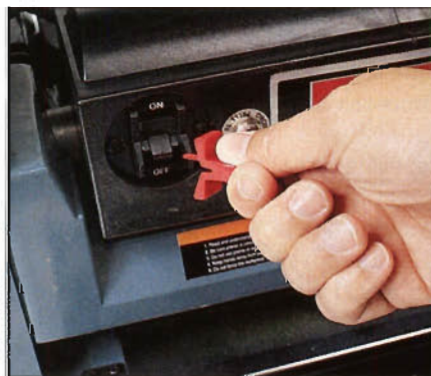
Photo H: Removable lock-out switches on the Jet and Sears planers prevent use by unauthorized individuals.
