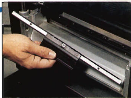
Photo A: Delta's magnet-backed lifter makes it easy to handle the knives and protects fingers from nicks and cuts.
