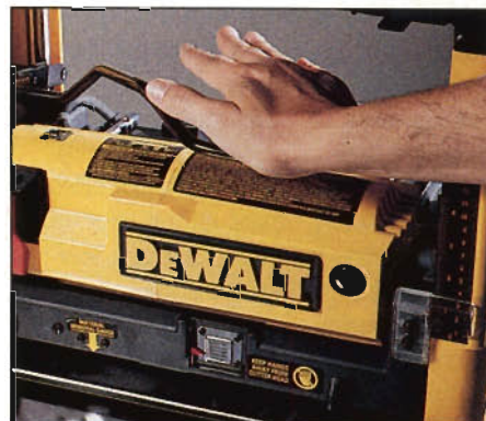
Photo C: To lock the head on the DeWalt planer, simply push down on the bar.
