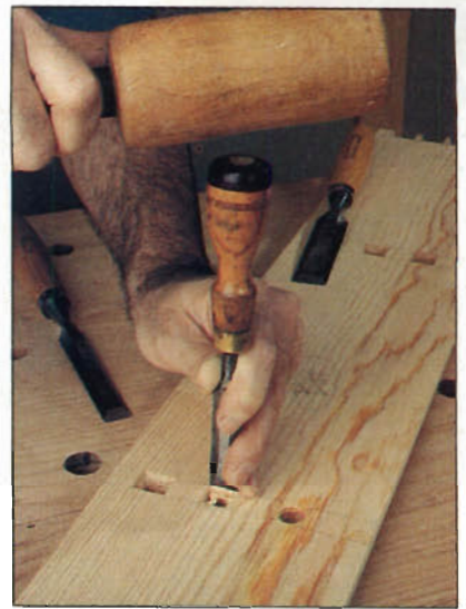
Photo E: After boring holes to clear most of the waste, square up the mortises by chiseling from both faces of the top/bottom.
