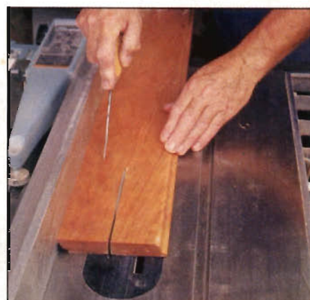
Photo C: As an alternative, start with double-wide stock and rout two of your profiles on opposite edges. Then, rip the piece in half to provide two layers' worth of stock.
