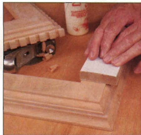
Photo L: Before gluing up the two-layer sub-assemblies, level the mating surfaces with a hand plane and sanding block.
