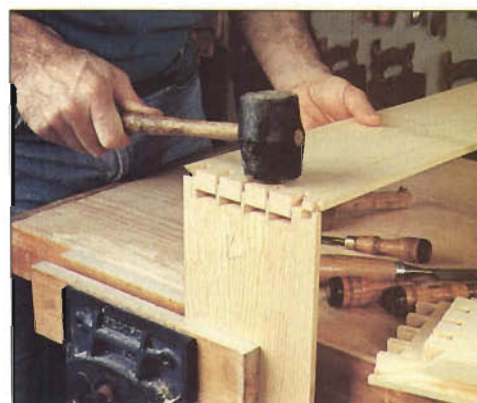
Photo A: To fit the mitered front edge of the dovetailed case parts, drive the joint home without glue. Note the small dovetail that secures the rabbeted back edge.
