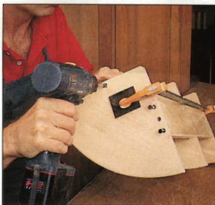
Photo G: After aligning and attaching supports to middle shelf, clamp top/bottom shelves to this assembly and bump them into position before drilling screw holes. When square, drill and counterbore the shank holes.
