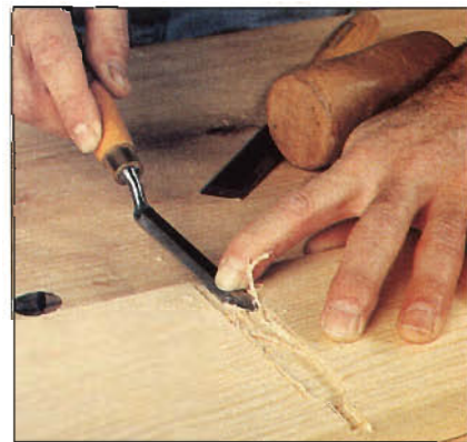
Photo B: Cut 1/8"-deep dados to seat the dividers. Square the shoulders of the full-width rear dado. Later, miter the shoulders of the narrow extension at the front to full width.
