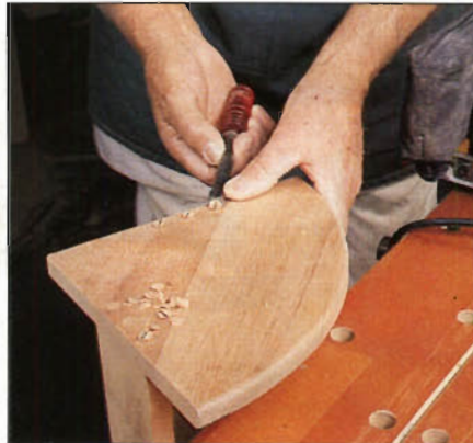
Photo I: Glue in plugs, then pare them almost flush with a chisel, taking a thin shaving in first one direction, then the other. Note pencil marks help align grain.
