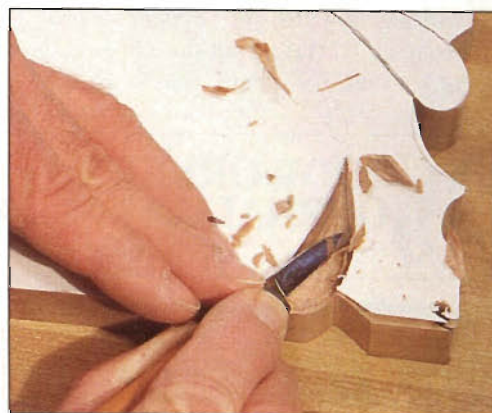
Photo D: Practice your carving strokes on the large waste piece from the frame opening, making cuts both with and across the grain to shape the teardrops. Note author's use of the left hand to steady and guide the knife.
