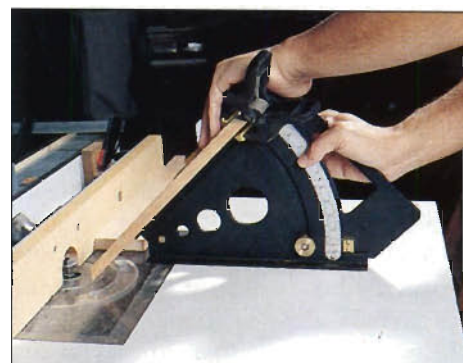
Photo A: Cut the itty bitty biscuit using an AngleWright or other 45^\circ -angled jig and a stop.
