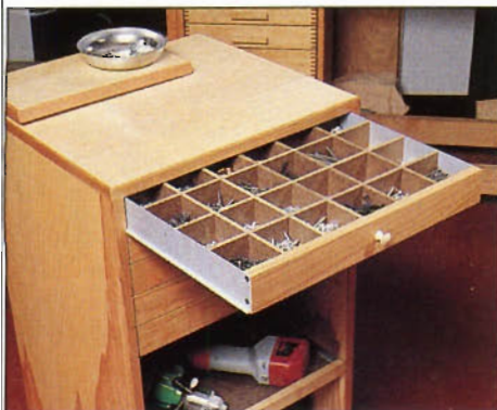
Photo A: The magnetic parts dish holds ferrous metals securely and the drawers can be divided into 30 or more compartments.
