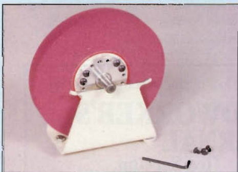
The grinding wheel rests on the balancing fixture. The flange and balancing screws help distribute the weight of the wheel evenly around the arbor.
