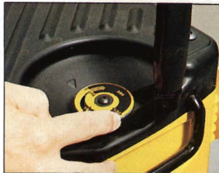
Photo E: A gauge on the DeWalt's elevation mechanism permits zeroing the existing setting before turning the handle.
