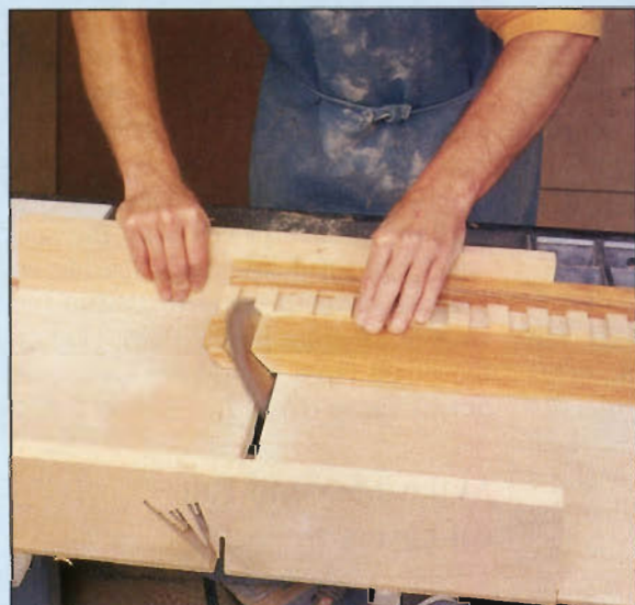
◀ Miter valance stock using a sliding table. As with crown molding, try to finish each corner with a full-width dentil.
