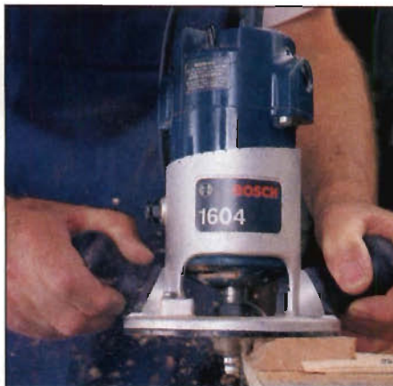
Photo B: Start with a simple Roman ogee for the bottom layer. Use wide ( 2\frac{3}{4} " stock for this layer to provide width for door overhang and also for firm attachment to cabinet top.
