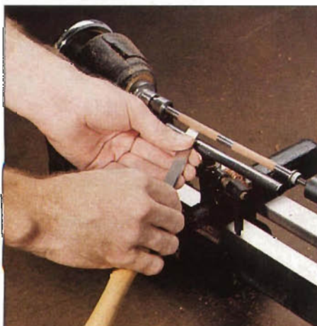
Photo H: Use a skew chisel to bring the barrel to within a few thousandths of an inch of its final diameter.
