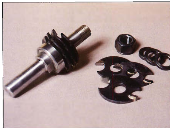
Photo A: To match your stock thickness, arrange the bit's individual cutters and spacers in different configurations on the \frac{1}{2} "-diameter arbor.
