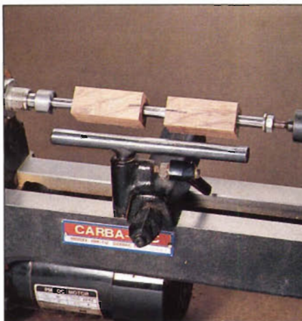
Photo F: The bushings space the blanks on the mandrel and also establish the diameters to which you turn the ends of the pen.
