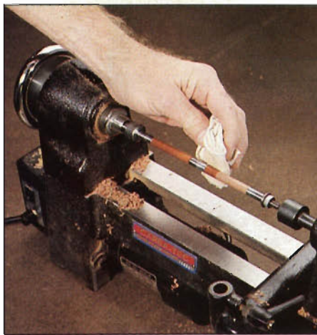
Photo L: Apply the finish with a soft cloth while the lathe is spinning slowly.
