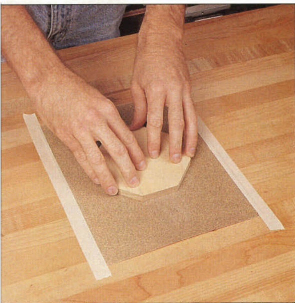
Sandpaper taped to a flat surface enables you to flatten parts and remove saw marks without rounding over the edges of the workpieces.
