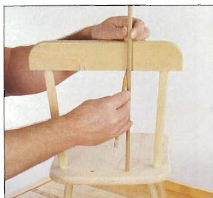
Photo B: Center the backrest between the rear posts, then mark the hole locations for the posts and back spindles.
