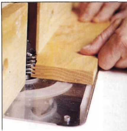
Photo B: The bit must be used in a table-mounted router equipped with a fence. On long stock use feather boards or other hold-downs.
