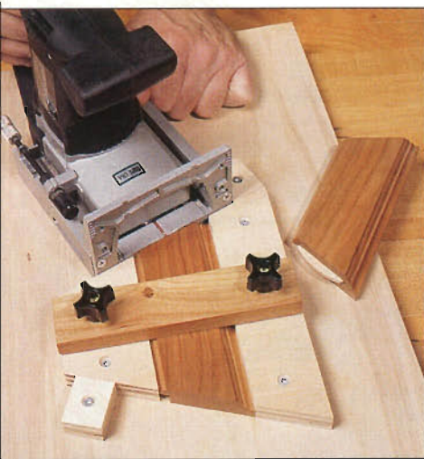
Photo A: Make a simple jig like this to hold the cap rails when cutting biscuit slots into their mitered ends.
