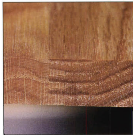
Photo C: Set up properly, the bit cuts perfectly matched finger joints in all species of wood.
