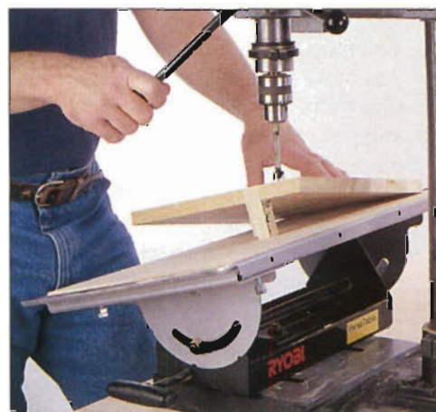
Photo A: To drill compound angles, tilt your drill-press table and tape an angle block to the underside of the workpiece.
