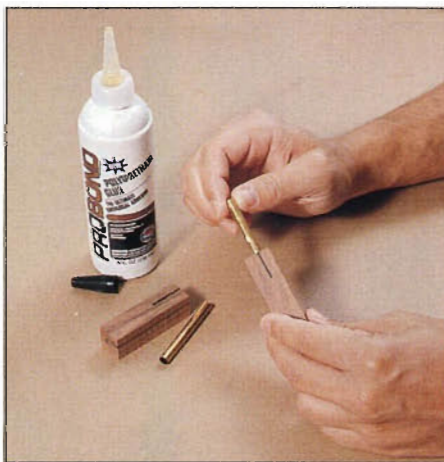
Photo C: Coat the brass tube with glue and rotate it in the hole before full insertion. We used polyurethane glue and allowed it to cure for 24 hours.
