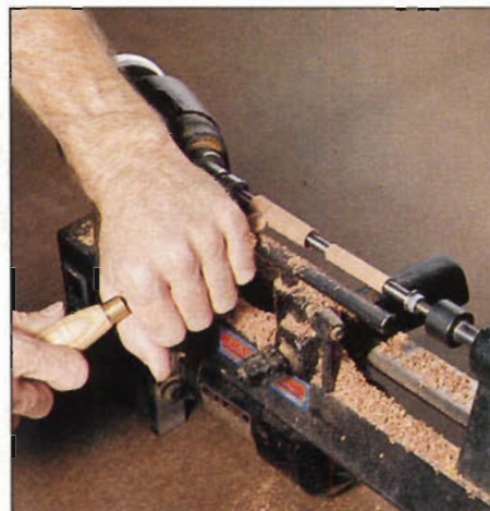
Photo G: A gouge brings the blank down to its rough shape. Work from the middle of the blanks towards their ends to avoid a concave barrel.
