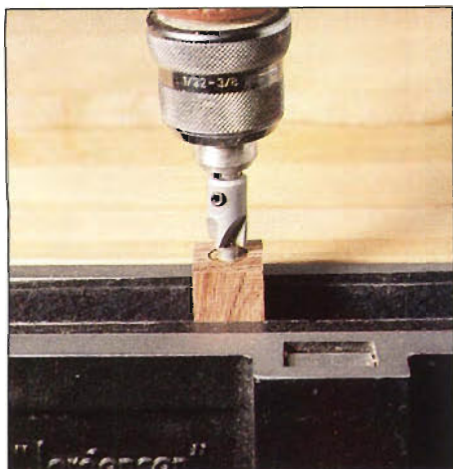
Photo E: Use the pen mill chucked into a portable hand drill to square and dress the ends of the blanks.
