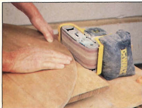
Photo D: To sand a tabletop edge square with its face, author clamps belt sander to the bench, partially burying the bottom edge of the sander in a scrap base piece.
