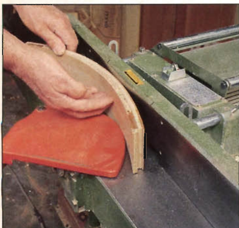
Photo K: Joint apron edges to 2\frac{1}{8} " final width. Hold the workpiece firmly against fence over cutter head to ensure uniform jointing over its entire length.
