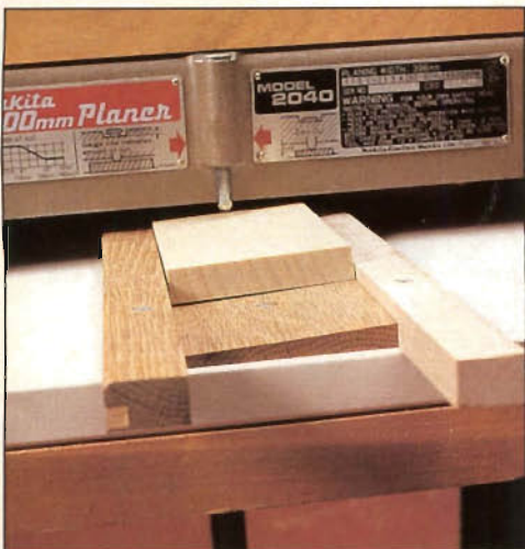
Photo A: Fixture used to bevel the four faces on each louver. Note the 4° bevel on the bottom slide strip attached to the auxiliary base.
