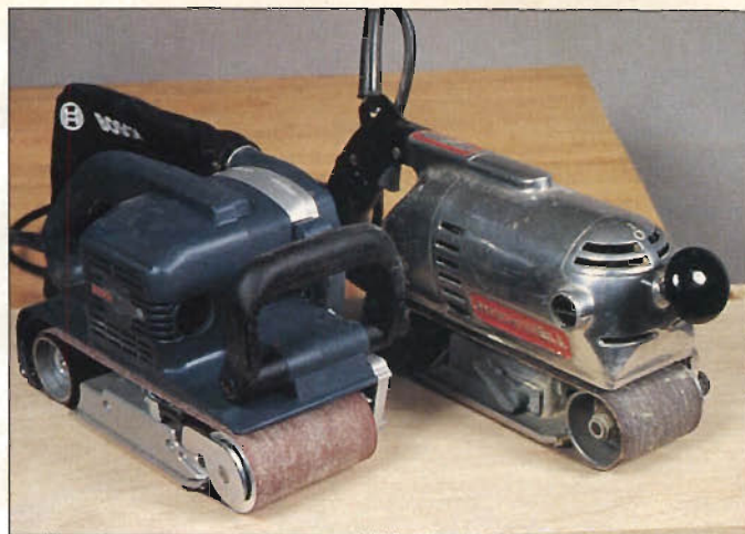
Photo B: The motor-mounting configuration determines the shape, size, and feel of a belt sander. On the Bosch, the motor is mounted crosswise. The Rockwell worm-drive model has its motor mounted in line with the belt.
