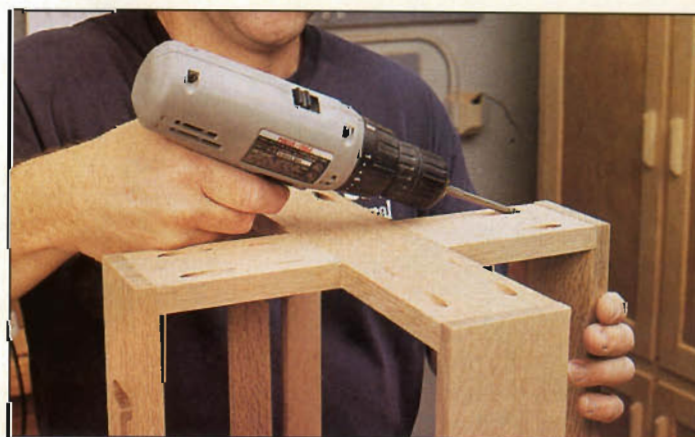
Photo B: Using a pocket-hole jig to predrill the screw holes makes assembling the legs and frame easy. Note half-lap top supports and rabbeted legs.
