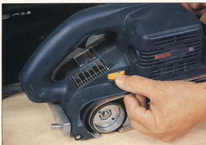
Photo C: With variable speed control, you set the belt speed. On this unit, you can select belt speeds from 1150 to 1550 SFPM.
