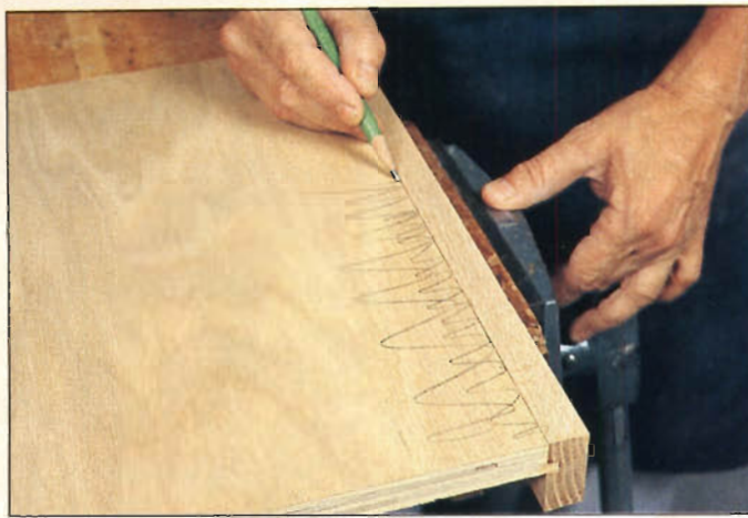
Photo K: To sand a hardwood edging flush with the surface of a plywood panel, scribble pencil lines on the plywood against the edging. Sand the edging, then attach the frame and sand both plywood and edging.
