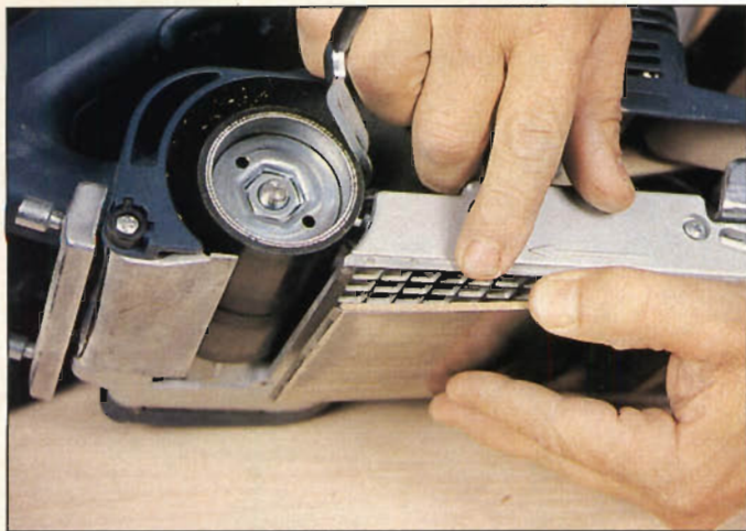
Photo E: Inspect the platen, pad, and wear plate when you change belts. Replace any damaged or worn parts.
