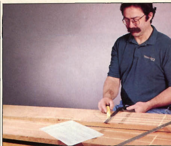
Photo B: Laying out rough-dimensioned parts lets you work around defects and select the best grain. It also ensures that you won't run out of stock in the middle of the project.
