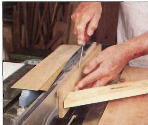
Photo F: Author resaws \frac{3}{32} "-thick cherry veneer strips from \frac{1}{4} "-thick stock. For safety, he cuts only one thickness from each piece and inserts scrap in the kerf to prevent binding during the second cut.
