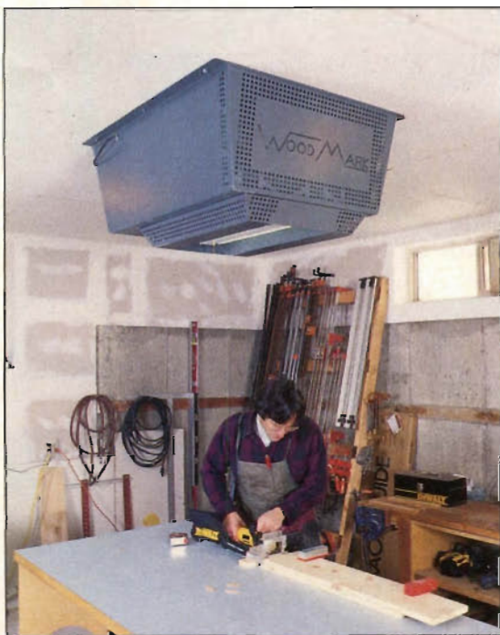
Photo A: WoodMark's ceiling unit filters 1100 CFM and draws air from all four sides, making it one of the most powerful and efficient machines in its class. Note the two-bulb fluorescent light on the underside.
