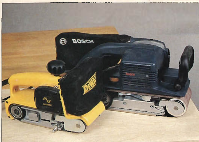
Photo A: Today's belt sanders come in different sizes. The DeWalt 3x21" unit has variable speed control and a dust-collection bag. The 4x24" Bosch has the same features. Both offer accessory sanding frames.
