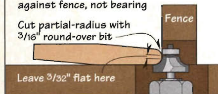
Figure 3 Routing round-over on louver edges
