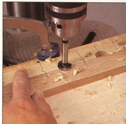
Photo D: Boring the partial holes in the openers. Note fence along back edge to position workpiece. Front cleat ensures a clean-cut hole every time.
