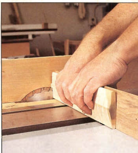
Photo B: Forming the tenon on the ends of the louvers on the tablesaw. Note dado head partially buried in the auxiliary wooden rip fence.
