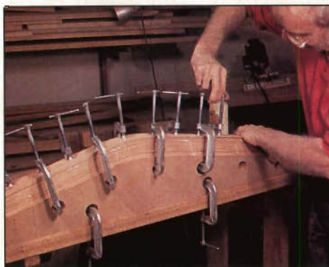
Photo A: To laminate the back legs, author placed one dry strip underneath and three on top of the bundle. He taped the bundle at the bottom end to minimize side-to-side slippage, then started clamping, tightening down each C-clamp before moving on to the next one.
