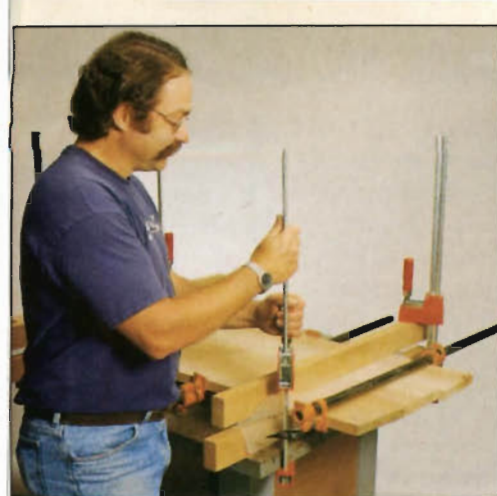
Photo D: Lightly clamped cauls keep edges of boards aligned when clamping.
