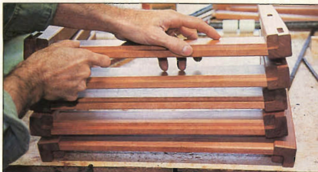
Photo B: A stack of front leg assemblies with the top edge of the frame rabbeted to accept the cushion frame. Front legs have a matching notch, which the author routs using a simple shop-made template.
