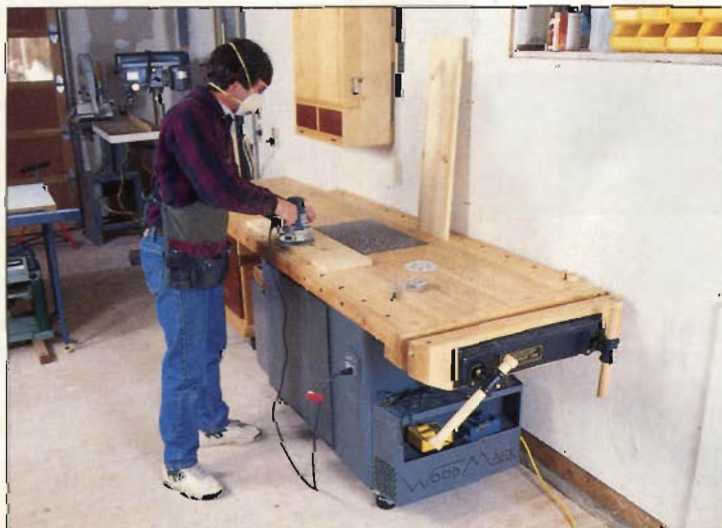
Photo B: The WoodMark downdraft bench draws 930 CFM and provides the mass and durability of a serious, professional-quality work surface.
