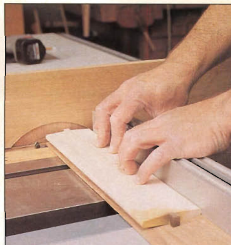
Photo C: Tablesaw set up to square-cut the \frac{5}{16} " tenons. Note 4° bevel strip again being used to support the beveled louver.
