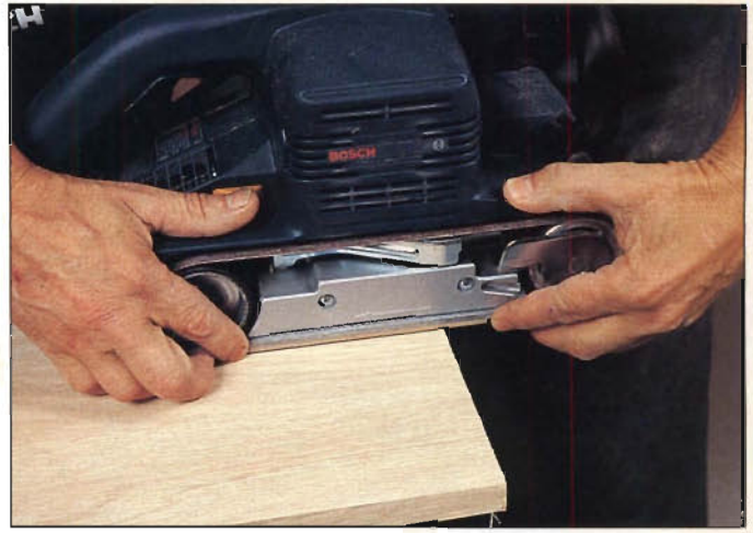
Photo J: Author points out front and back edges of platen which should extend about one fourth of its length over the edge of the stock.
