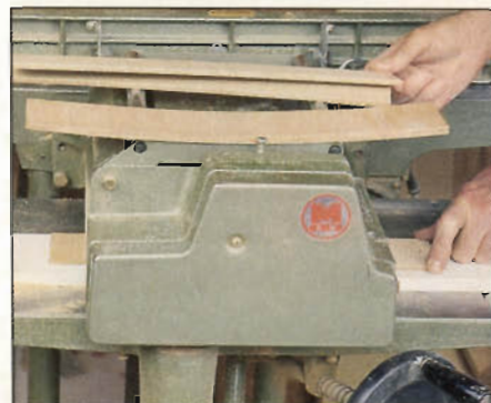
Photo G: To make "bender board" for laminating core layers, plane veneer off one face of 1/4" three-ply birch plywood. Use auxiliary table as shown if your planer won't cut material that thin.
