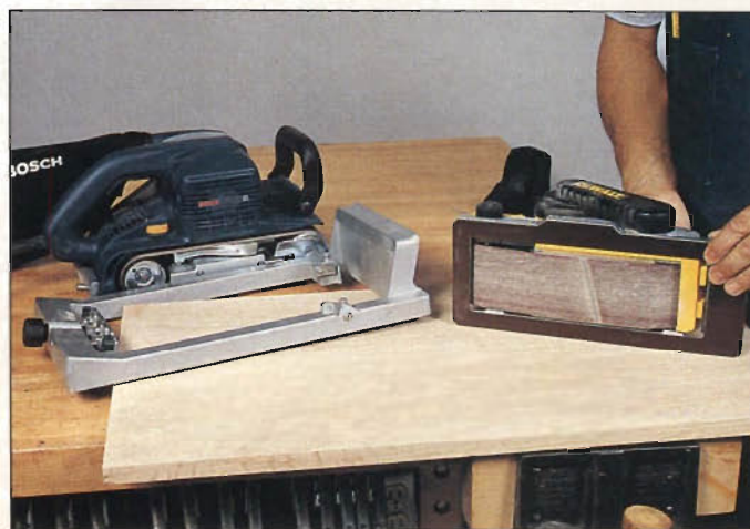
Photo D: A sanding frame attached to the bottom broadens the sander's base to improve its stability and controls abrasive contact with the workpiece.
