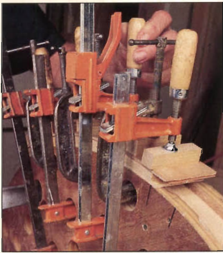
Photo H: For error-free laminating, author dry-stacks and clamps laminates before gluing, then and trims layers to rough length.
