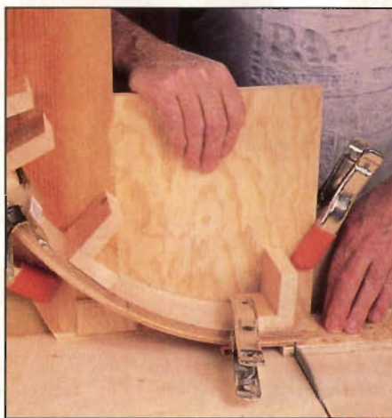
Photo N: To trim apron for back leg, stand jig on end on crosscut table, then cut apron square to 90° jig end.
