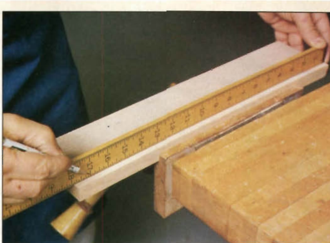
Photo E: When dimensioning parts for a project, use the same rule for all critical measurements.
