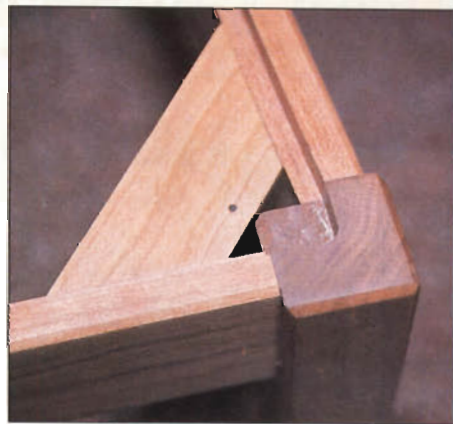
Photo C: Miter-cut corner blocks to fit the odd-angled joints. The shank hole drilled through block is used to attach the cushion frame after upholstery. Also note the \frac{1}{4} " chamfer on exposed ends and edges of parts.
