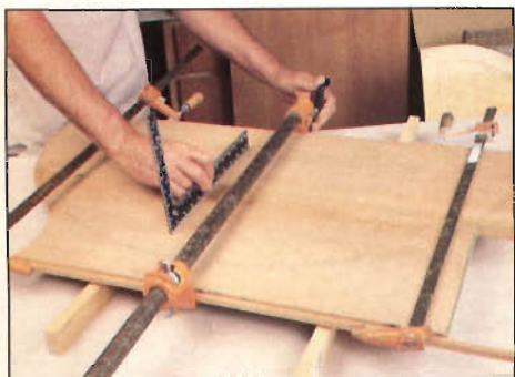
Photo C: Author cuts boards for tabletop to rough shape before edge-joining, then clamps using outside offcut as a clamping caul.
