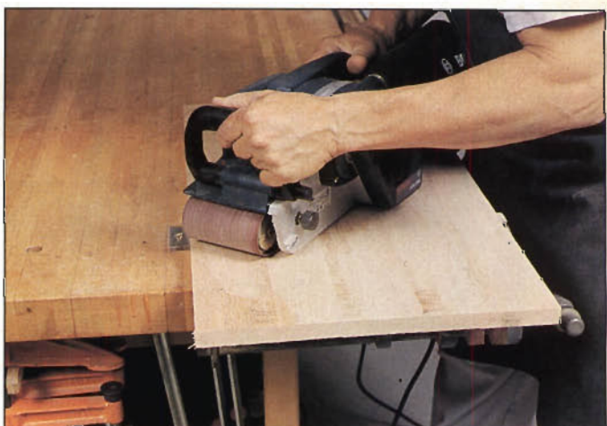
Photo H: Sand high spots down quickly by moving the sander across the grain at a slight (30°) angle.
