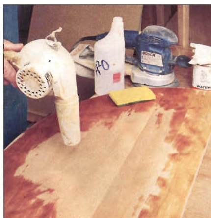
Photo P: To remove sanding "fuzz" that causes water rings to form beneath finish surface, dampen sanded tabletop with sponge. Blow-dry to raise fibers, then resand lightly.
