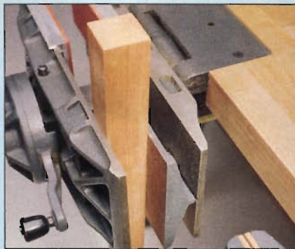
Photo F: These auxiliary tapered jaws fit inside the main jaws of the AMT enabling it to clamp tapered objects vertically.
