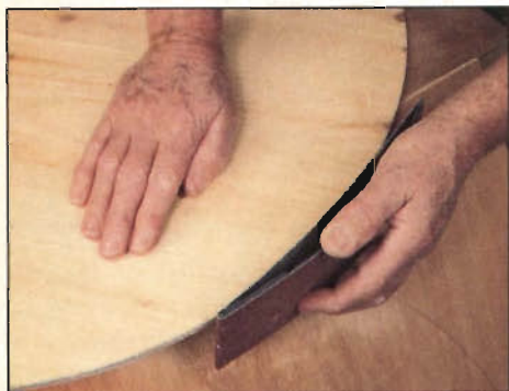
Photo B: To sand a near-perfect curve on the template and tabletop, author uses a simple bow sander made from a scrap piece of \frac{1}{8} " Lexan that is slightly longer than a flattened sanding belt.
