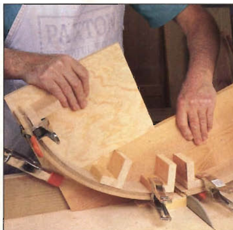
Photo L: To trim aprons square to tangent line for middle legs, use a shopmade jig and sliding crosscut table. Note backing board beneath workpiece used to minimize veneer tearout.
