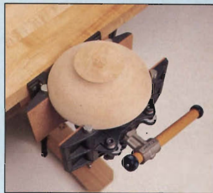
Photo D: Two dogs on each jaw face easily clamp round or irregular objects.
