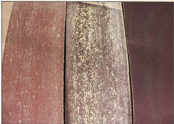
Photo F: A used but properly dressed (cleaned) belt left; a loaded and worn belt center; a new, unused belt right.
