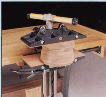
Photo C: Rotate a patternmaker's vise upward to clamp objects on top and bottom.
