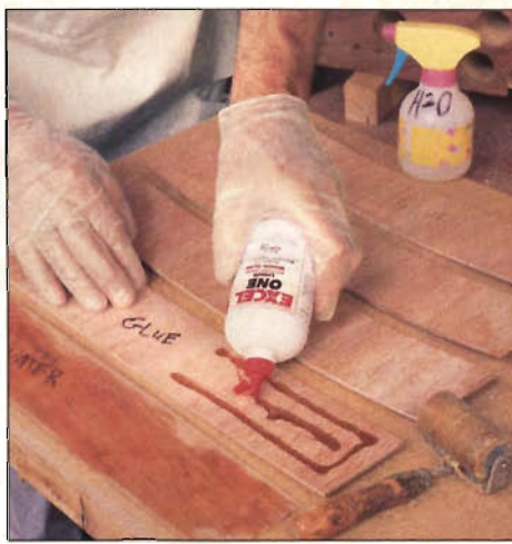
Photo I: Author dampens face of laminates with mist (to activate adhesive), then applies polyurethane glue to laminate faces, spreading it evenly using an artist's roller.
