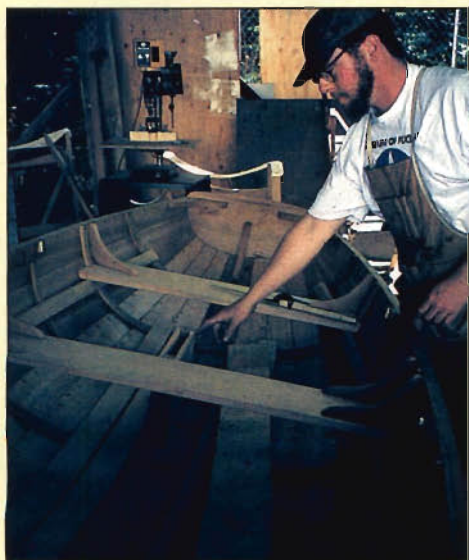
▲ Staff instructor Joe Crecca explains centerboard construction on a 10-foot lapstrake sailing dinghy built by students during a six-day workshop, one of the school's short courses.
