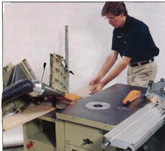
Photo C: To reach the thickness planer, flip up the two jointer tables. Then, crank up the bed and reposition the dust collector.
