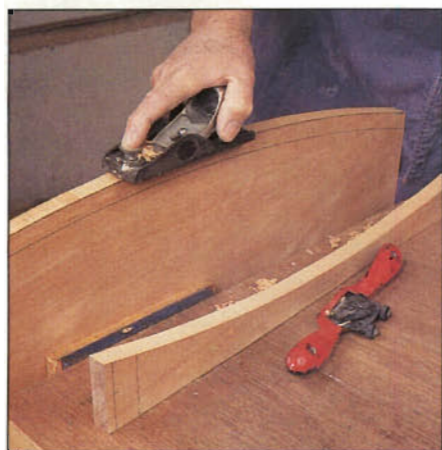
Photo E: After bandsawing outside radius of curved molding stock, use block plane to fair radius to the line.
