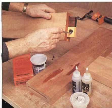
Photo B: Paint the surfaces to be joined with a coat of epoxy to wet them thoroughly. Author used a multi-piece tenon, which doesn't weaken the joint provided you use adequate adhesive.
