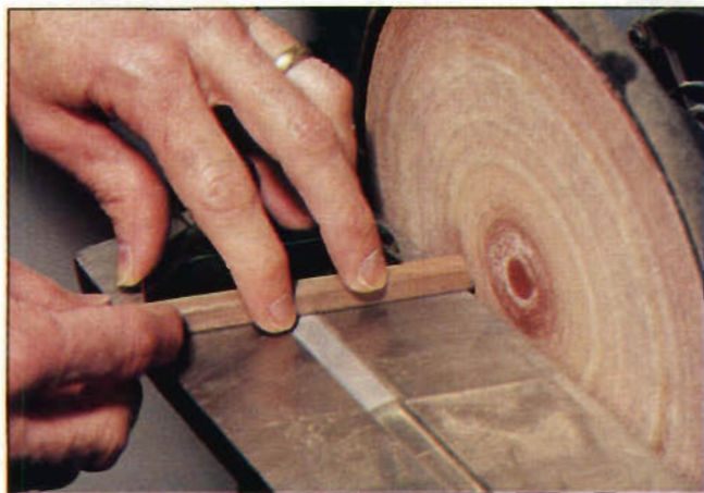
Photo D: Using the miter gauge as a guide, touch the ends of the plugs lightly to the sanding disc to create four triangular facets.
