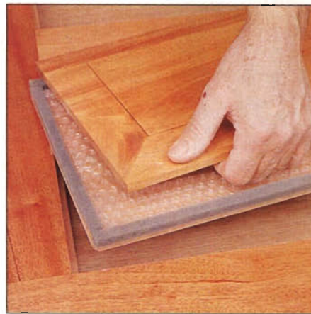
Photo J: Adhere foam insulation tape around edge of panel back, then cut insulation sheet to fit inside tape. (Author used bubble wrap.) Adhere sheet to bottom panel, then add top panel.
