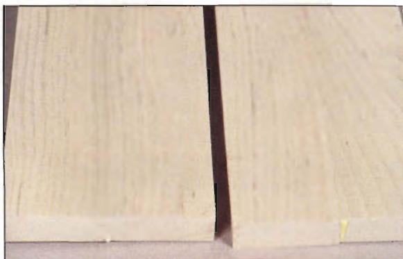
Photo B: Once squeeze-out was scraped away, glue lines of all products were undetectable on both light and dark woods.
