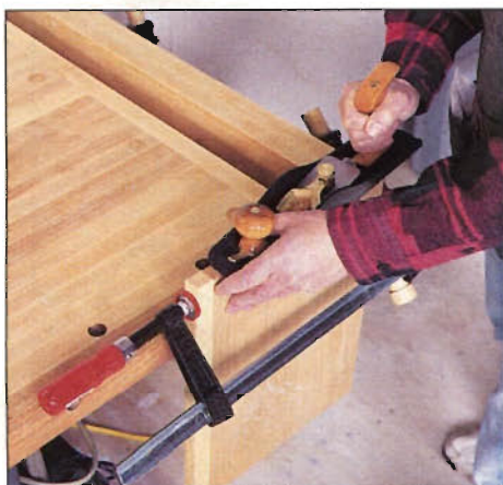
Photo 1: Low-angle jack plane cuts end grain best. Its top-beveled blade, set at a low incline with no cap iron, slices cleanly. Backing block clamped to workpiece edge prevents tearout.
