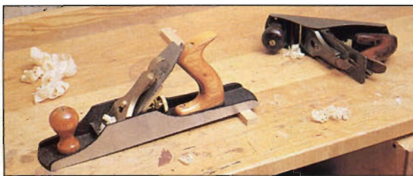
Photo C: Place a shim under the sole to protect the blade when not using the plane. Also, lay plane on its cheek whenever you put it down, facing the blade away from you for safety.
