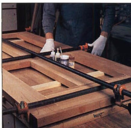
Photo C: Assemble frame on a flat, wax-papered surface, using light to moderate clamp pressure and pads that direct pressure to joint centers. Allow the epoxy to cure completely.
