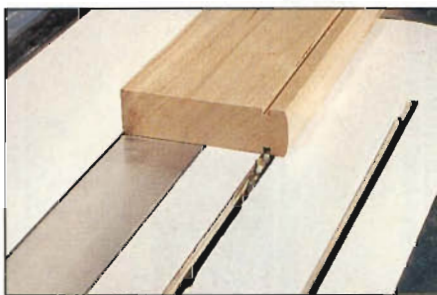
Photo F: The clear plastic teething rail provided in the hardware kit snaps snugly into a \frac{1}{8} " kerf you cut on the tablesaw.
