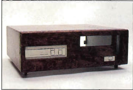
Photo F: Assembled CPU case. Test-fit all switches before gluing in the plastic plates. Make sure you don't get glue in any of the controls.
