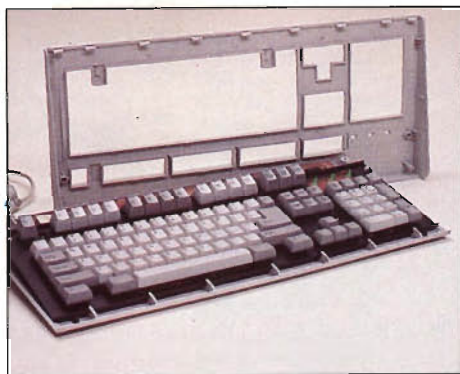
Photo A: If the keys are permanently attached to the cover, the keyboard can't be refaced. To determine this, remove the cover.
