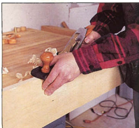
Photo F: To keep the plane's sole square to the workpiece edge, let your fingers slide lightly against the board's face. This helps keep you "in touch" with the plane's angle as you work.
