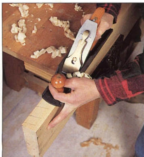
Photo G: To plane an out-of-square edge, hold plane level and start on the board's higher corner. As work progresses, shavings will gradually increase to full width of edge.
