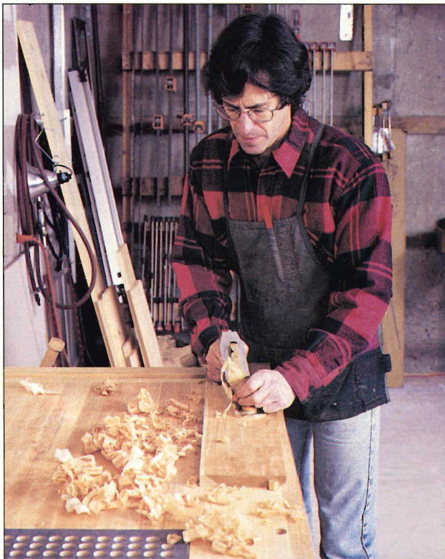
Author surfaces a board with 9" smooth plane. Because thickness planers leave milling marks, hand-surfacing still has a viable place in the woodshop, producing a mirror-like smoothness you can't get with sanding.
