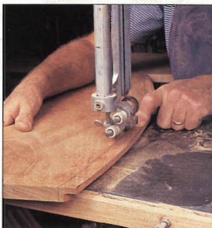
Photo F: Bandsaw inside radius of curved molding, then fair to the line using a spokeshave.
