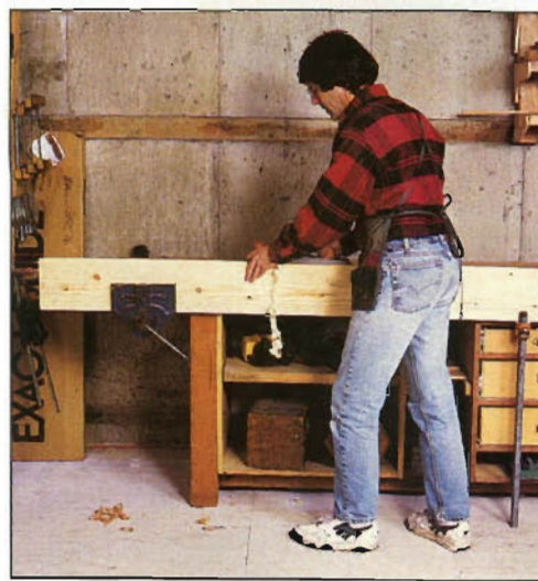
Photo E: To edge long workpieces, secure one end in a bench vise and prop the other end with a pipe clamp adjusted to correct height.
