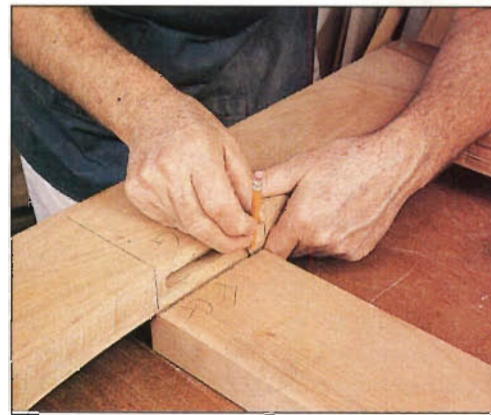
Photo A: To cut dividers accurately, dry-clamp the stiles and rails, then trace radius directly onto top divider blank.
