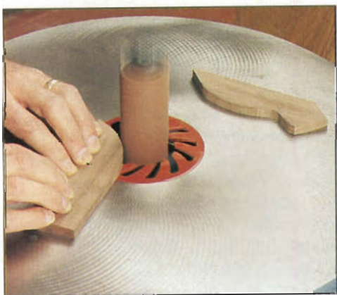
Photo D: An oscillating spindle sander, shown here cleaning up the bandsaw marks on the walnut splines, comes in handy for several operations in this project.
