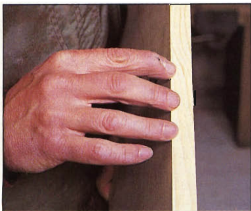
Photo B: To check for emerging grain, run a finger lightly along corner of workpiece. In this board, grain direction is clearly visible, but reading grain with a finger may be essential with roughsawn stock.
