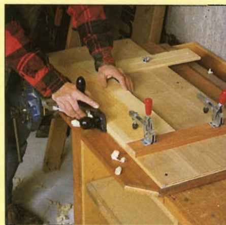
Author's shooting board has toggle clamps and a ramped work support. Here he uses a Record "technical" plane, which has high cheeks and a side handle designed for use with this fixture.
