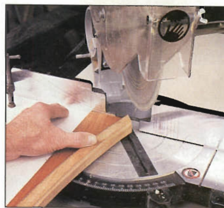
Photo G: Make template to orient curved molding properly, then miter each end to match template angle. Author's miter saw won't cut an angle greater than 45^\circ , so he turns template 90^\circ to fence to compensate.
