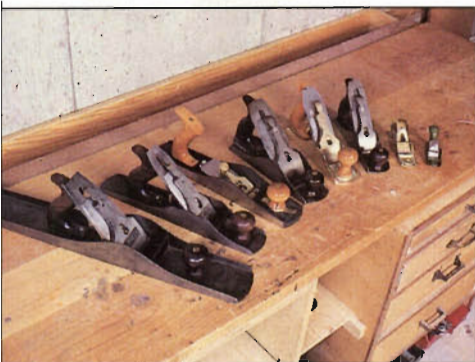
Photo A: Select the right plane for the job. Shown here (front to back): 24" jointer (#8), 14" jack (#5), 14" low-angle jack (#62), 10½" wide-body smooth (#4½), 9½" standard smooth (#4), 9" narrow-body smooth (#3), 5" block, and 3" Kunz palm plane.
