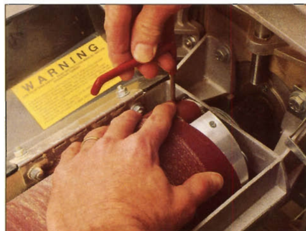
Photo B: Performax's "TufTool" takes some of the strain out of securing the adhesive strip.
