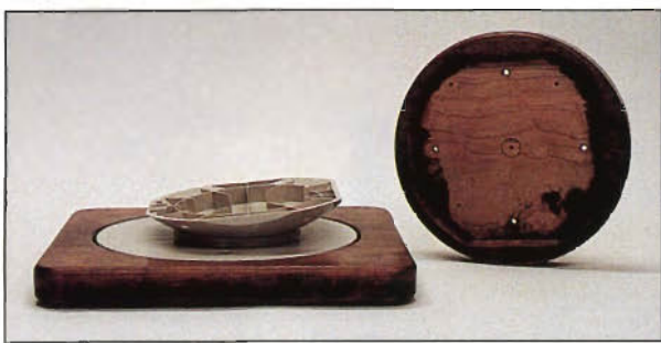
Photo J: To make the pedestal base, author first cut hole in top piece to accept the lower base plate, then glued the two \frac{3}{4} "-thick pieces together. The standing piece is routed to fit the upper pedestal section.
