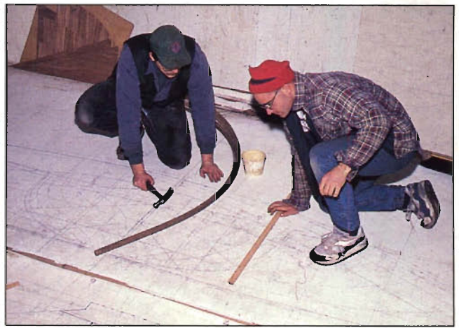
▶ Scott Whitesides (left) and Scott Chichura plot hull lines on the school's lofting floor.
