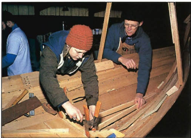
◀ Amy Sandidge fits a bilge panel in a 15' faering with help from instructor Ray Speck.
