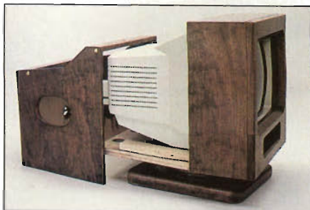
Photo G: Author's two-piece monitor cover. The front frame glues to the base, and the monitor sits on a flat spacer. The back attaches with screws.
