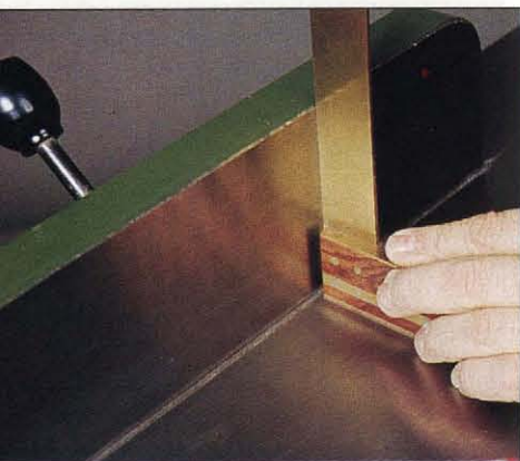
Photo B: Checking the 90° setting on the jointer fence and table with a try square.
