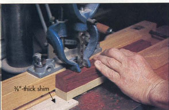
Photo B: To cut the through mortises in the head blank, make a carrier board to support the workpiece. Place a 3/8"-thick shim under the end of the carrier to angle-cut the inside end of each mortise.
