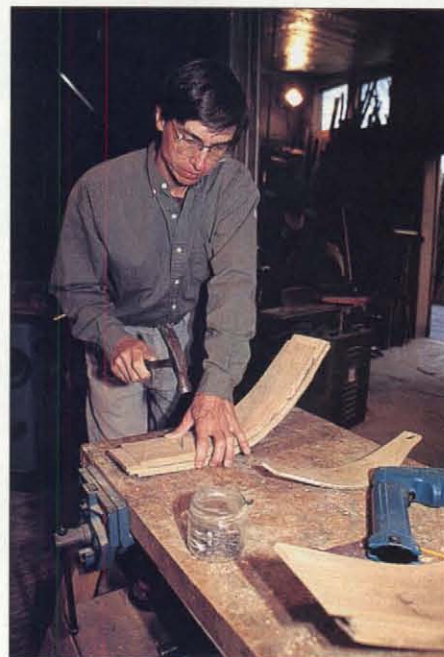
Photo K: I match a set of bent slat blanks for color and grain, then stack, pilot-drill, and nail them together in the waste areas.
