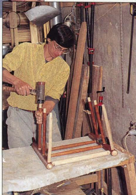
Photo T: I assemble the side rungs to the chair front and back using a shot-filled mallet and softwood block. I size the rung tenons slightly larger than the mortises (about .003") for a snug fit that won't crush wood fibers.
