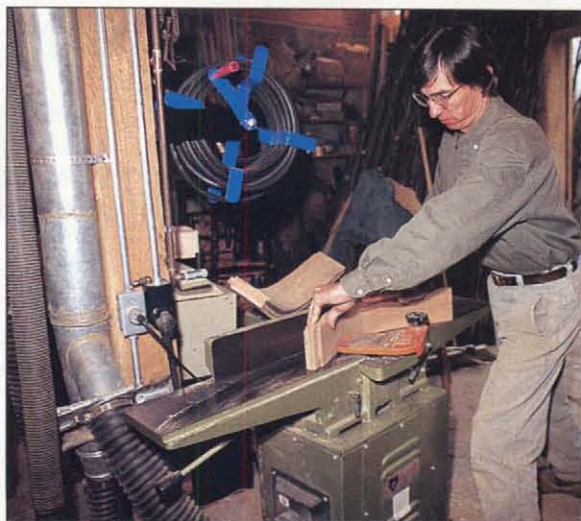
Photo L: I straighten the bottom edge of the stacked slats on the jointer, then crosscut the ends. Because of the curvature, each slat is a bit shorter than the next one down in the stack.
