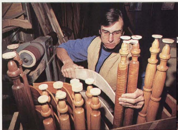
Photo O: I also use the drum sander to thickness the slats, checking the ends for fit in the back-leg mortises as I work. Note the yet-to-be-parted finials on the back legs.
