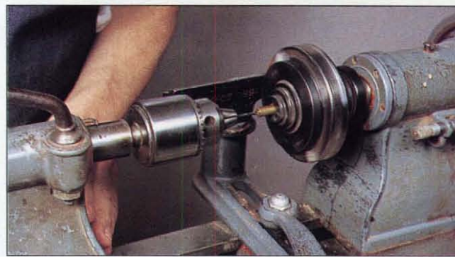
Photo G: To center a \frac{1}{8} "-deep hole in the end of the \frac{3}{16} " brass rod, chuck a length of rod into the lathe, then install a no. 39 bit in the tailstock to drill the hole.
