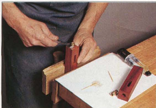
Photo C: After applying epoxy, thread the compression fittings into the holes, but don't over-tighten them.
