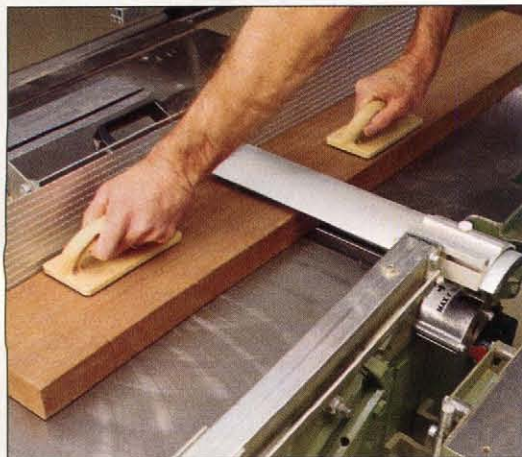
Photo C: On the jointer, the guard prevents you from getting your hands near the cutter head.
