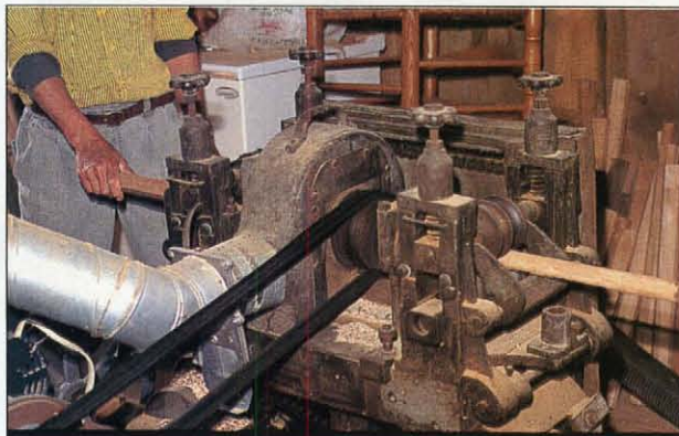
Photo B: To rough-out the chair rungs, I use a 1920s-vintage dowel cutter that I salvaged from a broom factory.
