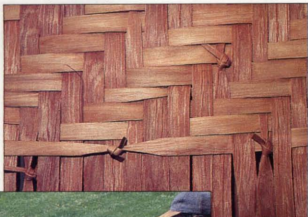
◀ Photo U: This close-up of the underside of a woven seat shows the staggered weave and carefully knotted hickory bark strips.
