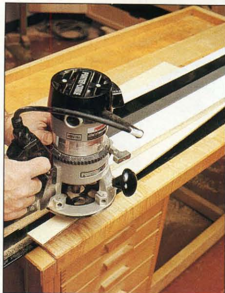
Photo D: To cut the tapered plywood panels, rout to the line using a straightedge or jig to guide the router.
