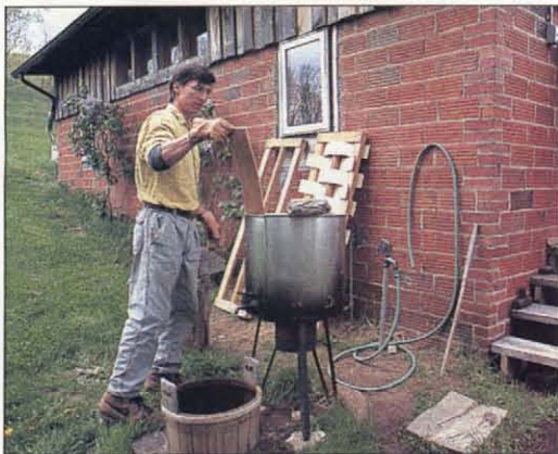
Photo I: To bend the slat blanks, I boil them for 15 minutes in a stainless-steel kettle. Unlike cast iron, stainless steel doesn't react with the wood's tannic acid.
