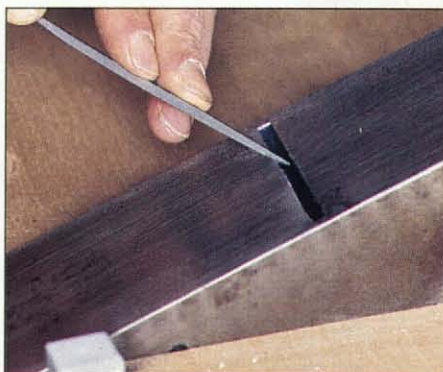
Photo F: Using a second-cut or mill-bastard file, form a \frac{1}{16} " bevel on the back and side edges of the mouth opening.
