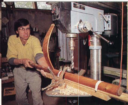
Photo N: After tracing the profile from a pattern, I bandsaw the top edge of the stacked slats with a single cut, then drum-sand them to final shape.
