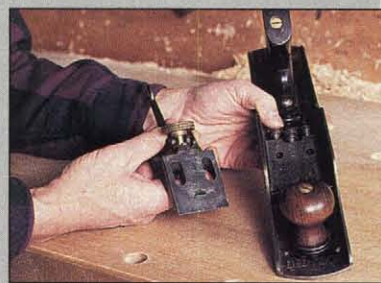
Pre-WWII Stanley Bedrock planes feature machined frog bed (shown here on a #5), which offers superior performance to more common cast beds.
