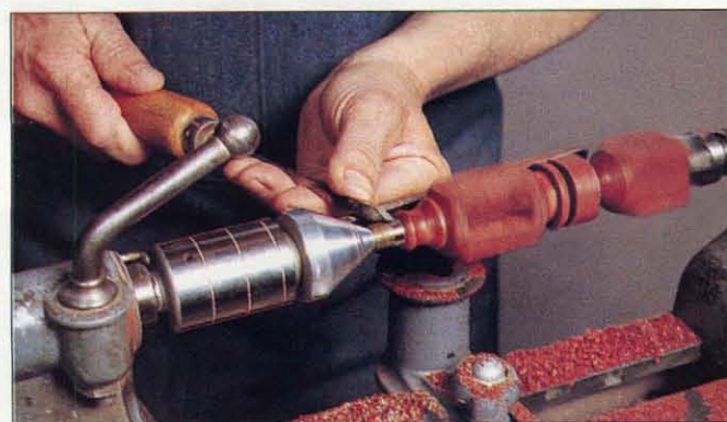
Photo F: Author uses the heel of a high-speed steel skew chisel to round the hex section of the brass compression union.
