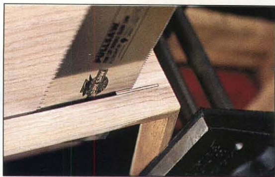
Photo E: Finish the glass slot after assembling the box by carefully cutting along groove lines using a Japanese ryoba or other backless, thin-kerf saw.
