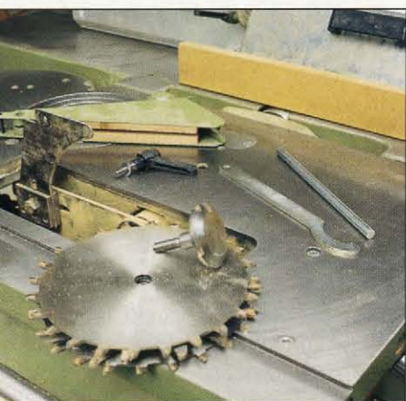
Photo A: The arbor bolt with the large head enables you to use a dado set.
