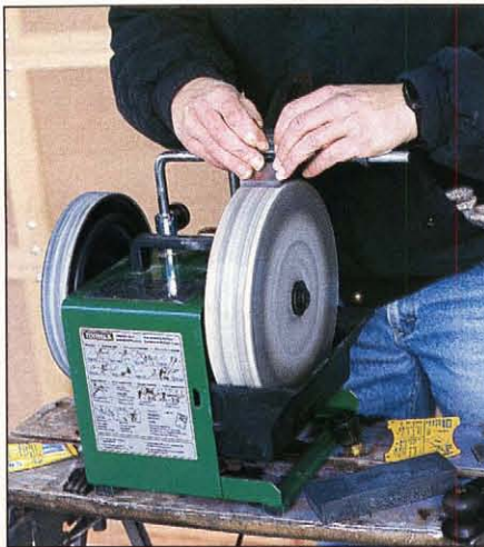
Photo D: If blade bevel is not ground to the time-tested 25° angle, regrind it using a slow-turning, large-diameter water-cooled wheel. The water keeps the blade cool, preserving its temper, and a large diameter reduces hollowing, which weakens the cutting edge.
