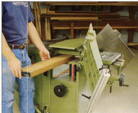
Photo D: Tilting back the jointer tables gives you access to the planer bed.
