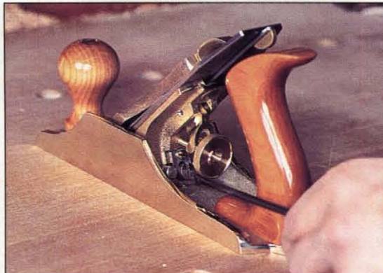
Photo 1: Adjust frog position relative to mouth opening to fit the job: \frac{1}{8} " for coarse shavings, \frac{1}{16} " or less for fine. Lie-Nielsen (shown) and Stanley Bedrock planes provide frog screws accessible at rear of frog, which allow removal of frog without having to remove the blade/cap iron assembly.
