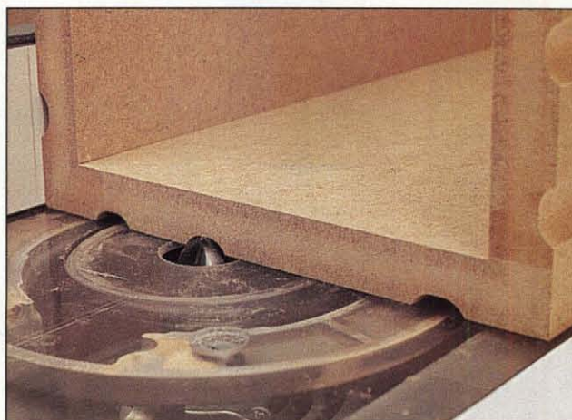
Photo C: You need just two fence settings to rout the four flutes in the column sides. After routing the first flute at each setting, turn the piece end for end, then rout the second flute starting at the opposite end. Move fence to cut the second set of flutes into each side.
