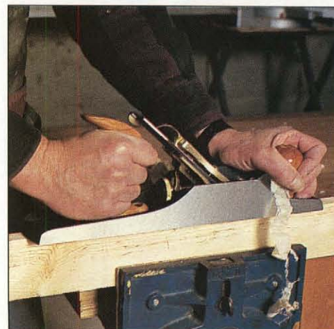
Photo B: If he could own only one plane, the author would choose a jack. This versatile 14-15" tool will smooth surfaces, joint edges, and plane end grain.
