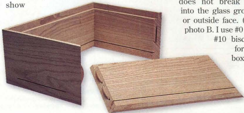
Photo B: Rabbet the back edge of the case parts to accept a \frac{1}{2} "- or \frac{3}{4} "-thick plywood back. Cut a thin groove near the front edge for the single-strength glass pane.
