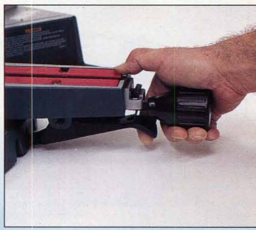
Photo H: The Bosch turntable uses notches and a detent trigger. It also has a detent override clip that lets you swing the turntable freely to any position on the miter scale.
