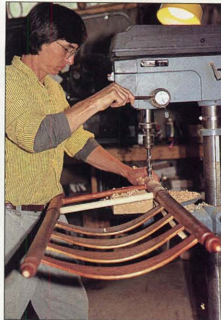
Photo R: After gluing up the back and front as separate subassemblies, I drill angled mortises for the side rungs. To do this, I use a V-block jig with a beveled block that supports the unit at the correct angle.
