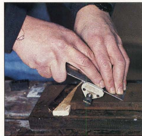
Photo E: To hand-sharpen, use water stones and a blade holder that holds the 25° bevel flat on the stone. Author starts with 1000-grit stone, then proceeds to 1500-, and finishes on 6000-grit. He deburrs back of blade by rubbing firmly once or twice on 6000-grit stone.
