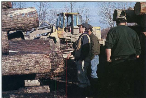
Photo A: At the Rosewood Lumber Co., mill operators let me select my own logs and then saw them to my specifications. I sticker the lumber in a breezy but covered location and allow it to air-dry for about a year.
