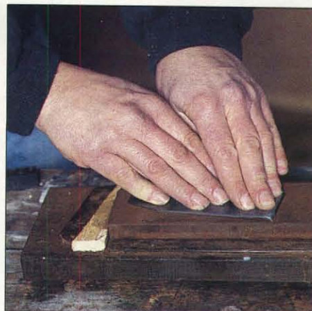
Photo G: Cap iron must sit flat on blade. To eliminate any gaps, flatten cap iron's bearing surface on lapping plate or coarse honing stone.
