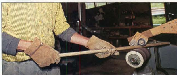
Photo C: To smooth the rung blanks, I devised a fixture for the stationary drum sander that uses skateboard wheels.
