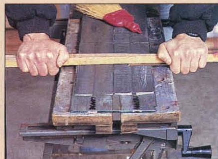
A flat piece of wood enables author to apply firm, even pressure to the plane blade during the lapping process.
