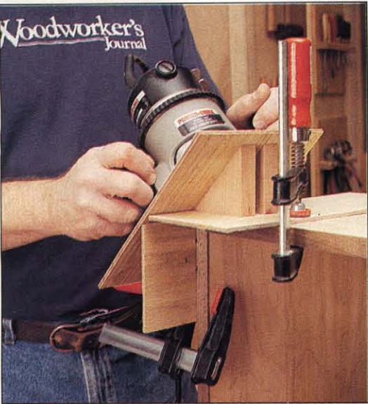
Photo A: With this jig you can rout the key slots on the chest corners easily and accurately.
