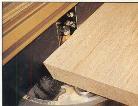
Photo A: Routing a profile with an offset fence reduces the risk of splintering.
