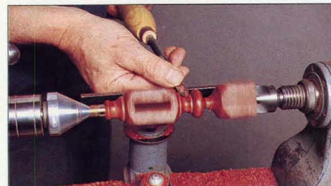
Photo E: Lay out each turning section, then turn and sand both blanks to identical finished profiles.
