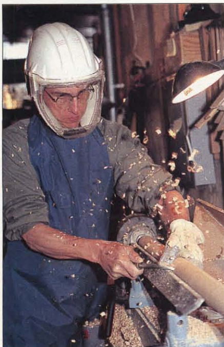
Photo D: I rip the square leg blanks to hexagonal shape, then do the roughing-out work with a \frac{3}{8} " spindle gouge modified with an "Irish grind."
