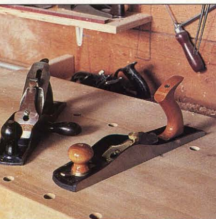
Photo C: Two jack plane variants. Low-angle jack (right) has blade incline of only 12° for cleaner, easier end-grain planing. The "technical plane" (left) features wider side cheeks and removable side handle which makes it easier to use with a shooting board.
