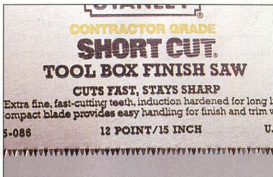
Photo A: The darkened teeth indicate that they have been heat-tempered, which keeps them sharper longer.
