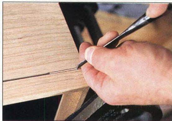
Photo F: After sawing to the groove limits, square the ends of the glass slot using a small chisel. Make sure slot ends align with the glass grooves in the sides.
