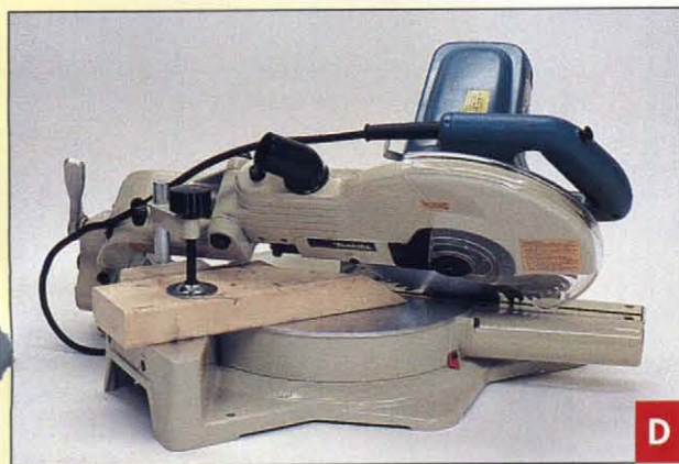
Sliding compound-miter saws cut stock four different ways: a square crosscut ( photo A ); a flat miter ( photo B ); a bevel cut ( photo C ); and a compound miter or mitered bevel ( photo D ).
