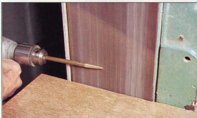
Photo H: Author shaped the brass rod to profile using a portable electric drill and belt sander.
