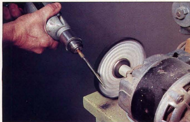
Photo J: Buff and polish the brass scribe to a scratch-free high gloss.
