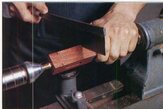
Photo D: Before turning each head to profile, cut kerfs to help prevent chipping at the points where the blank makes transition from square to round.
