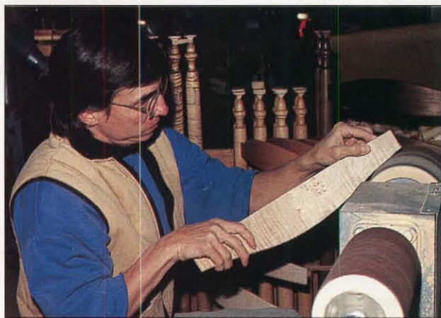
Photo N: After tracing the profile from a pattern, I bandsaw the top edge of the stacked slats with a single cut, then drum-sand them to final shape.
