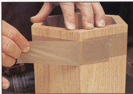
Photo B: For effective, low-cost clamping of multi-sided projects, strap the pieces with brown packaging tape.
