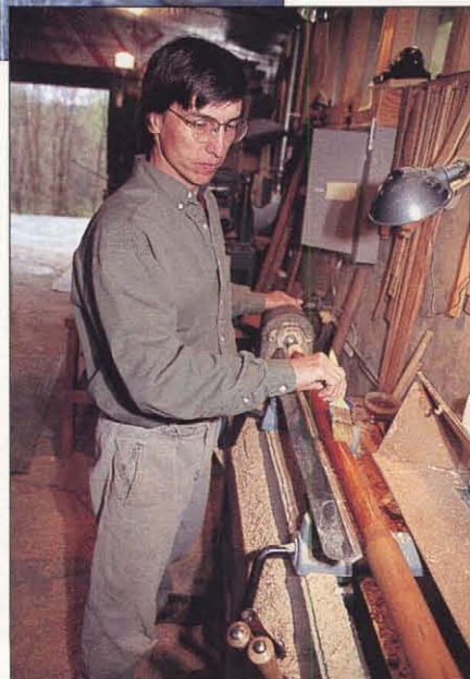
Photo H: Pre-finishing ▶ legs on the lathe makes for easy buffing and a lot less finishing work after assembly. Since I cut all mortises and tenons after this initial oiling, I don't mask these areas.
