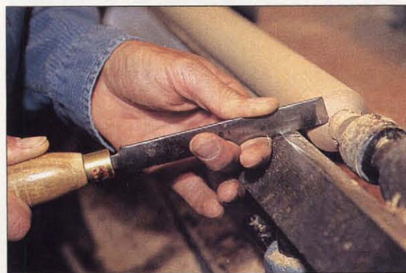
Photo E: After laying out the leg using a "story stick," and pencil, I use a parting tool to score the grooves that mark mortise locations, then size the coves and beads to their proper diameter.
