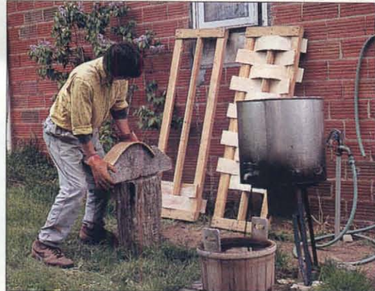
Photo J: After bending the slat blanks on a form, I dry them under tension on a rack for one to two weeks. The slats are ready to work when they've dried enough to slip out of the rack.
