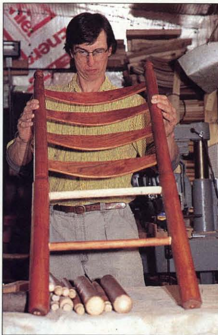
Photo Q: After drilling the back rung mortises, I assemble the back legs, slats, and back rungs. I use glue on the rungs but not on the slats, which I'll peg later. The woven seat will cover the unfinished seat rung.
