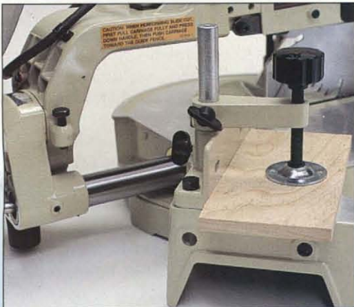
Photo I: Makita's workpiece clamp simply screws down onto the workpiece.
