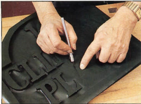
Photo G: Apply the masking film to the plaque face, then cut around the letters and borders. Leave the film intact to mask areas you do not want painted.
