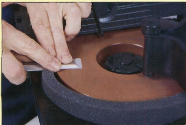
Horizontal wet wheels quickly and accurately flatten the backs of chisels and plane irons.
