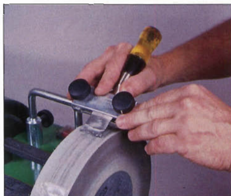
Photo B: Tormek's universal support arm accommodates all of the company's sharpening jigs.
