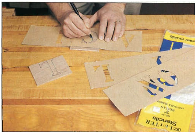
Photo B: By using full-sized stencils, we were able to trace the letters directly to the letter stock for cutting.
