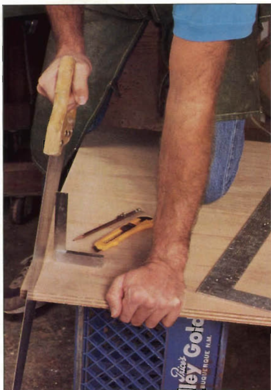
Photo A: For larger-scale work such as panel-sawing, an 18"- to 20"-high sawhorse (or milk crate, shown here) supports the workpiece at just the right height: low enough to let you get a knee and plenty of body weight on it, but high enough that you don't stab the floor with the saw tip.
