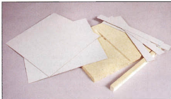
Photo E: The base for any fixture can be built from particleboard and surfaced with melamine or plastic laminate.
