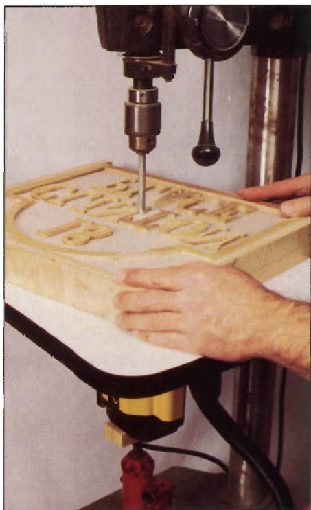
Photo A: To use the inverted-pin router, place the plaque blank in the carrier box, lower the guide pin to the carrier, and elevate the router bit. Then, maneuver the carrier and templates around the guide pin.
