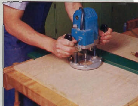
Vacuum T-square works without metal clamps that would interfere with the router's operation.
