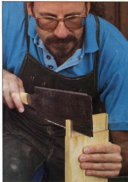
Photo F: Japanese saws, made of thin steel and given less set than Western saws, cut a very narrow kerf. Because they cut on the pull stroke, tension virtually eliminates binding. This backless ryoba saw has fine crosscut teeth on one edge, rip teeth on the other.
