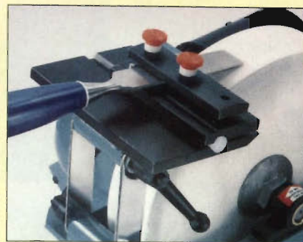
The tool holder rides in the groove in the table, providing complete control of the tool on the wet wheel.
