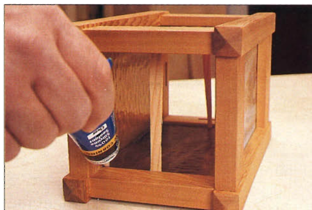
Photo B: Two thin, springy sticks hold each glass pane in place while you apply silicone caulk.
