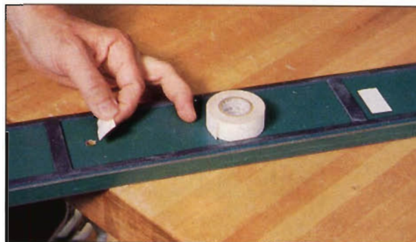
Photo F: Seal unused vacuum ports with plastic tape.
