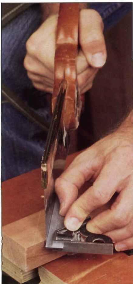
Photo D: A combination square makes an expedient guide for a 90° or 45° cut. Author has found that this method neither notches the guide nor dulls the saw.
