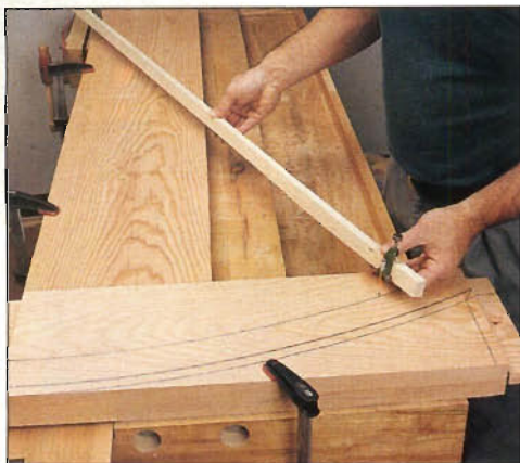
Photo A: Using trammel points and a beam, lay out the radii of the top rail and curved molding on the 2x10 blank. Note: We pre-cut the tenons to show how they square to the rail ends.
