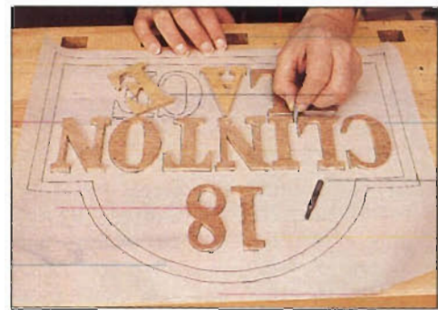
Photo D: Space letters for optimum readability. Remember—diameter of guide pin and router bit determines minimum spacing.
