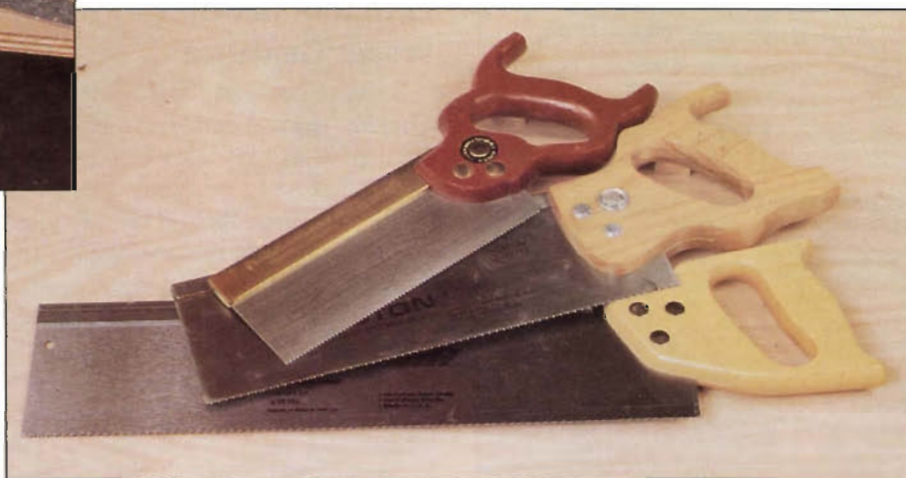
Photo C: Conventional backsaws come in three size ranges, represented here (top to bottom) by an 8" saw with 20 points (a tenon saw); a 12" model with 15 points; and an 18" saw with 10 points (a miter saw).
