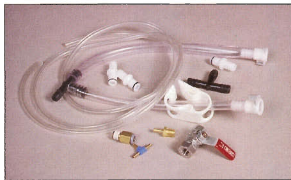
Photo D: Quick-connect fittings make it easier to move from one fixture to the next.
