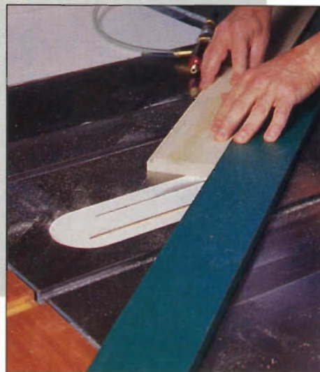
Vacuum straightedge being used as a tablesaw fence to cut a cove.
