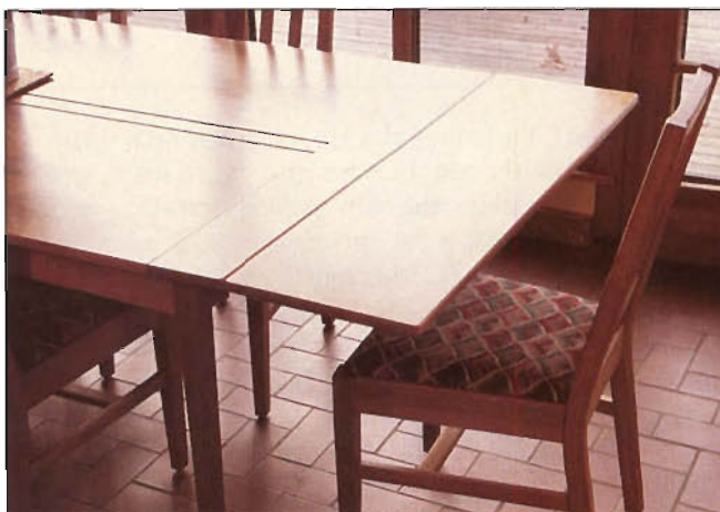
Photo A: The tabletop's lengthwise center divider with its two expansion gaps adds visual interest and gives the two large panels room to shrink or swell as environmental conditions change.
