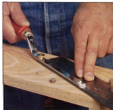
Photo G: A flush-trim saw's teeth have no set or are set only on one face, which lets you trim dowels, plugs, and projecting parts nearly flush without marring the surrounding surface. The saw's back protrudes only on the off-face, and the handle rotates 180° for left-handed use.
