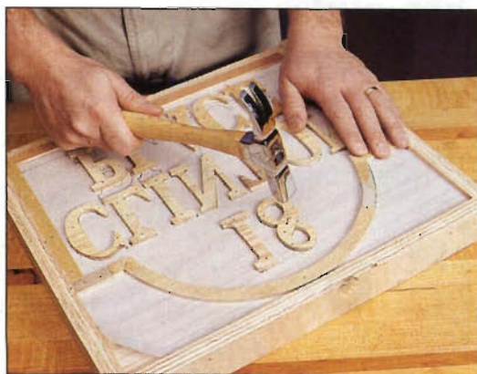
Photo F: Position layout paper upside down on carrier, then tack nail templates to it. Layout should appear backwards.
