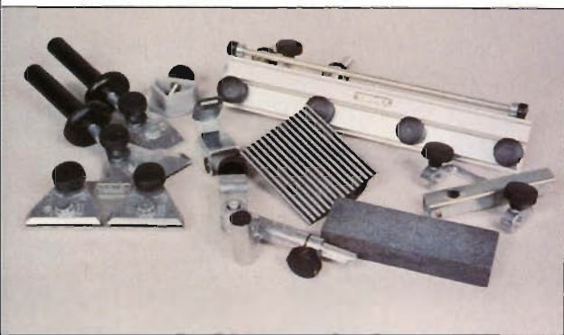
Photo C: A sampling of the many Tormek sharpening jigs currently available for the grinder.
