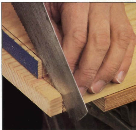
Photo B: To make a straight start on a small trim cut, clamp a slightly wider scrap board with the kerf already started underneath the workpiece, and use this kerf as a guide. The scrap board also minimizes tearout.
