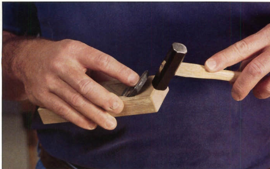
Photo B: To remove the blade, tap gently on the chamfered edge along the back end of the block, alternating from one corner to the other. As you tap, hold the blade and chip breaker with a finger to keep them from flying out.
