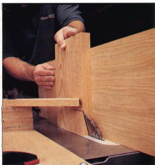
Photo A: Use an auxiliary fence and a feather board elevated above the blade to stabilize the piece when you cut the chamfers on the lantern roof.
