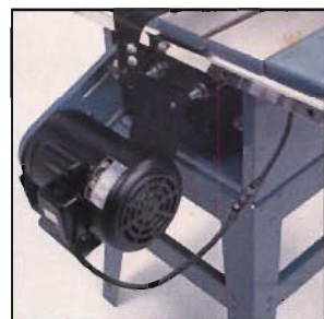
Totally enclosed, fan-cooled motor. Quick-connect plug requires no wiring; just plug in male and female connectors.
