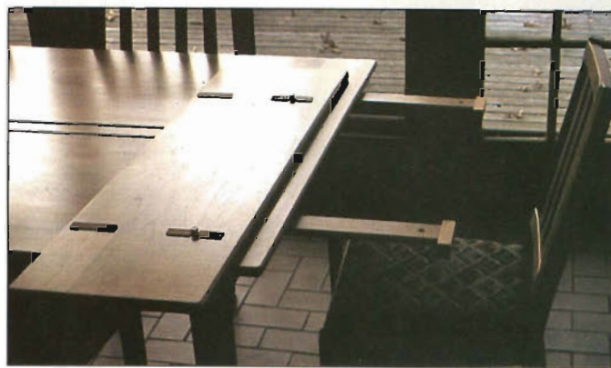
Photo C: The two leaves rest on simple, slide-out supports. Note alignment pins and felt strips on leaf underside. Supports have stop pins underneath, finger pulls on ends.
