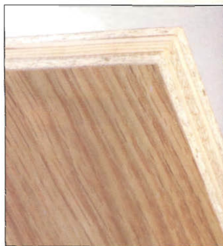
Photo B: As a veneer substrate, Classic Core plywood combines the strength of plywood with the flatness of particleboard.
