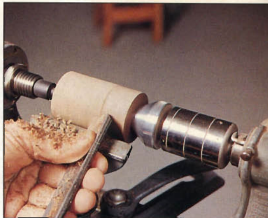
Photo A: Using a roughing-out gouge, form the turning square into a cylinder.
