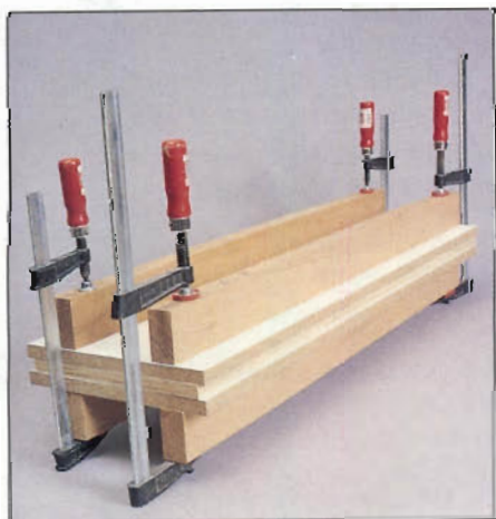
Photo G: For larger sheets of veneer, apply pressure using clamps, cauls, and equally spaced rows of beams. The ends of the beams should be tapered like those on the router jig shown in figure 4.
