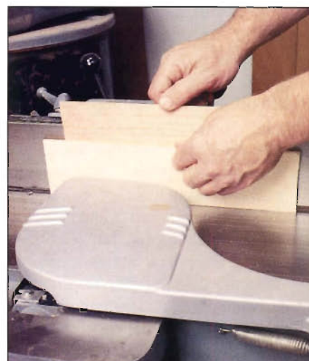
Photo C: Straighten short pieces of veneer on the jointer by sandwiching them between pieces of scrap block.
