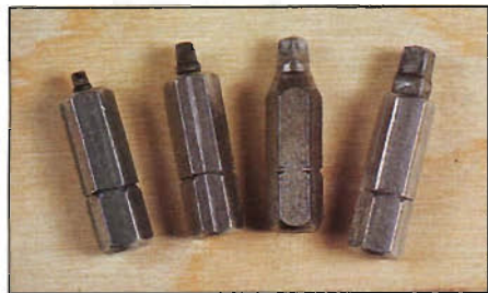
Photo B: Square-drive bit sizes (l to r): #0, #1, #2, and #3.
