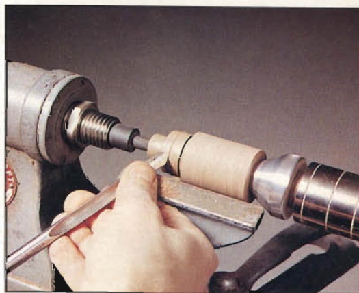
Photo C: Mark, then turn the 1\frac{1}{2} "-diameter cylinder to form sections 1, 2, and 3.
