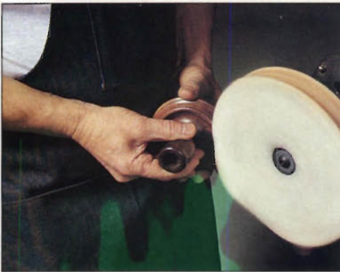
Photo M: After the oil finish has cured, buff the holders to the desired sheen.
