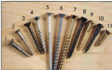
Photo G: Screw materials and coatings: (1) plain mild steel (no coating or plating), (2) stainless steel, (3) dry-lube coating, (4) zinc plate, (5) galvanized, (6) ceramic coating, (7) yellow zinc plate, (8) black phosphate coating (pre-lubricated), (9) solid brass, (10) blued, and (11) brass-plated steel.
