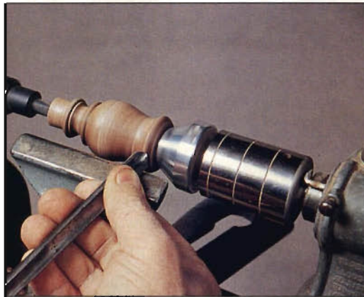
Photo F: Turn the half-bead at the end of the spindle (section 3) using a \frac{3}{8} " gouge.
