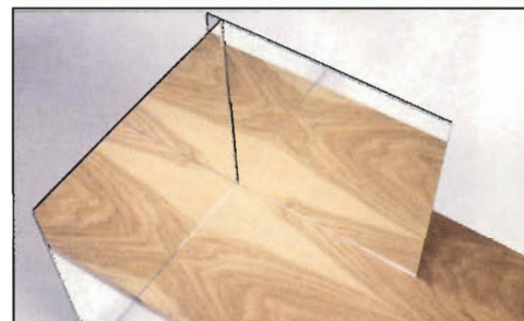
Photo A: Mirrors held perpendicular to the veneer surface enable you to visualize patterns and find the best locations for the edges.
