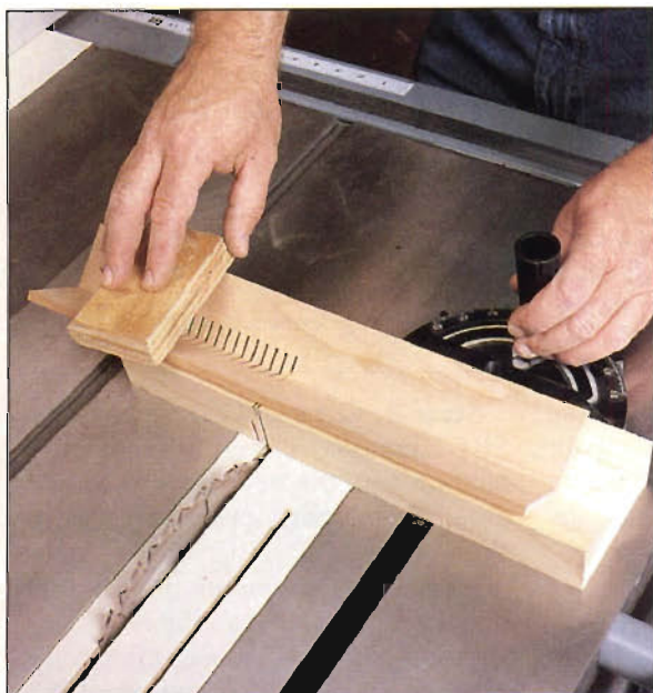
Photo B: Use a slotted V-block with a key to get clean, uniformly spaced cuts in the shade ridge (O).
