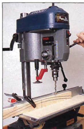
Photo B: After laying out the curved back legs, drill holes in the blanks before bandsawing legs to shape.
