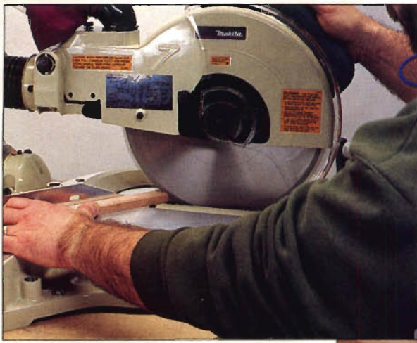
Photo D: To prevent tear-out when cutting the frame miters, the author places the inside edges of the frame pieces against the fence with the front face up.
