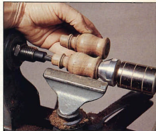
Photo G: Compare the two candle spindles and fine-tune them to correct any discrepancies.
