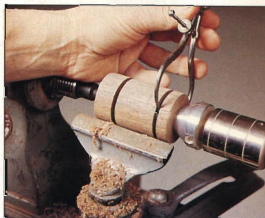
Photo B: Use a parting tool and caliper, part the cylinder in at least two places to establish a 1\frac{1}{2} " overall diameter.
