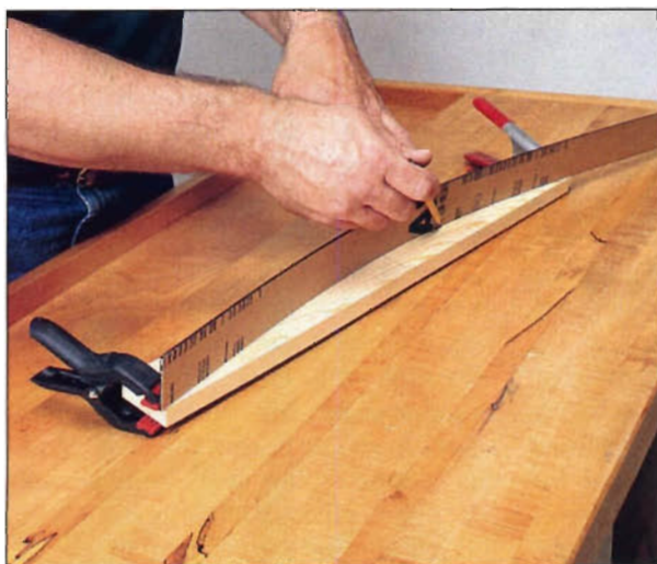
Photo A: Use a flexible straightedge to lay out the curved back legs.
