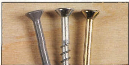
Photo F: Self-countersinking screw heads. Note nibs on underside of head for cutting the countersink.
