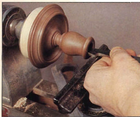
Photo L: Use a side scraper to taper the inside of the candle hole.
