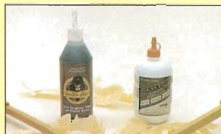
Photo E: Gorilla Glue and Excel polyurethanes require 8 to 20 percent moisture in the surrounding wood to cure properly.
