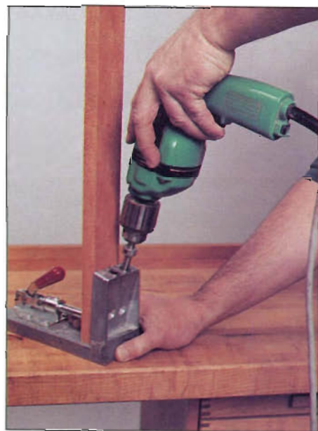
Photo A: To drill pocket holes in the rails, clamp a pair of guides to the workpiece, then use 3/8" step drill bit to counterbore and drill shank holes at 15° angle. Note: Holes enter the face, exit the end of the rail.
