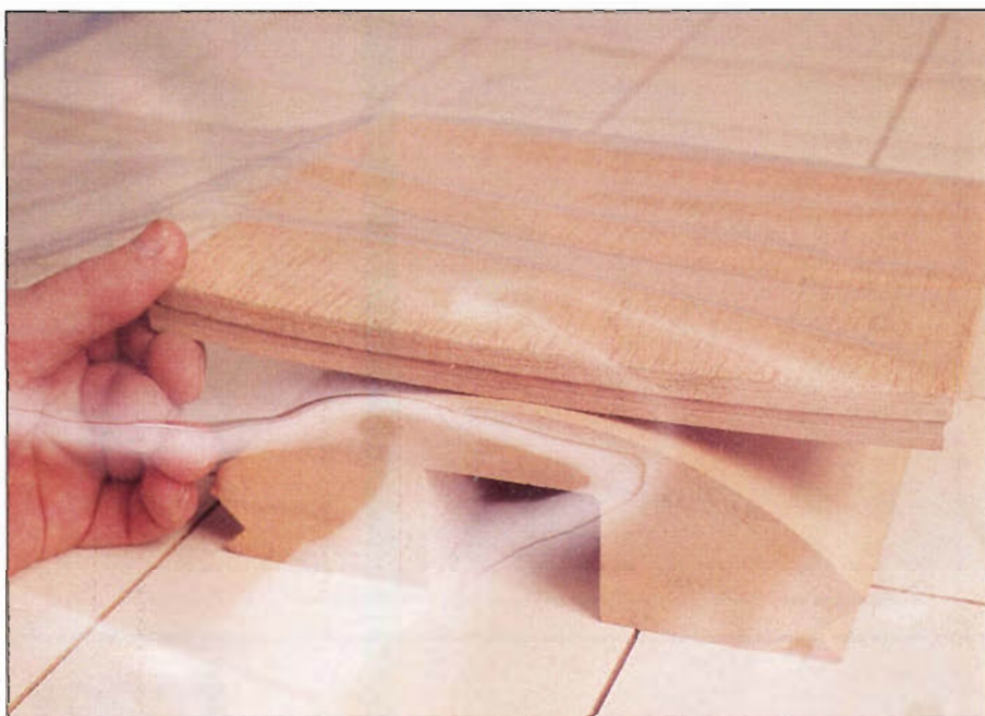
To create a curved substrate for veneering, we glued up two pieces of bending plywood, then positioned them over a particleboard form on a gridded, melamine-faced platen inside the bag.
