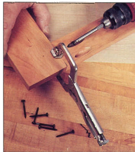
Photo B: Before joining rails to stiles, align faces of mating parts flush using special clamp. Then, drive self-tapping face-frame screws, which eliminate need for drilling pilot holes in stiles.
