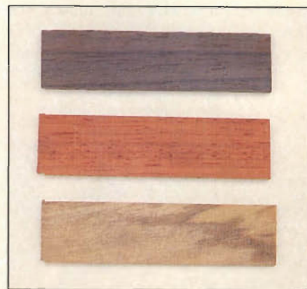
Photo E: Select three woods that contrast in grain or color or both. Cut a \frac{3}{16} "-thick slab from each wood large enough to generously cover the knife handle recess.
