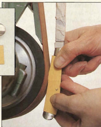
Photo C: Sand the template edges to match the knife contours. Be careful not to oversand and remove any knife metal.
