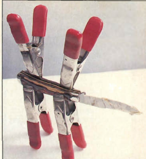
Photo M: Epoxy and clamp the mountainscape inserts to the knife blank one at a time. On the bottom edge, clamp insert to the knife liner on that side. On top edge, clamp across back spring.
