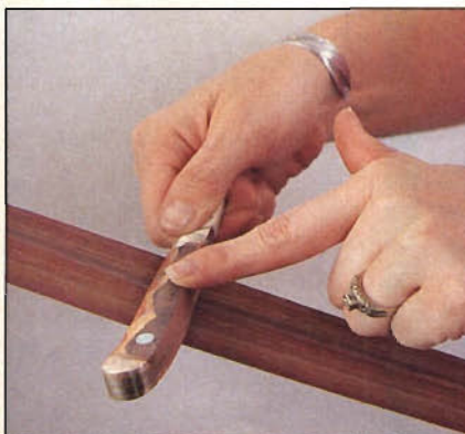
Photo P: Remove platen from belt sander, change to 120-grit belt, then gently round insert faces and bolsters. Sand up to 220- and then 320-grit to achieve a satin-smooth finish.
