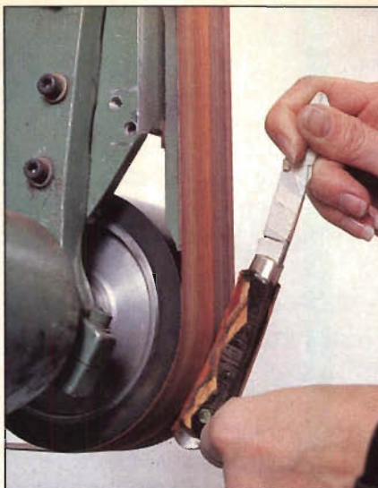
Photo N: Sand edges of the two inserts to match contours of knife. Be careful not to sand away any metal.
