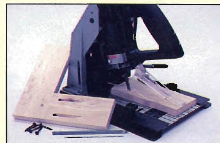
Photo Q: Working in a commercial cabinet shop's assembly line, I built face frames using a pocket-hole cutter, a handy device that didn't slow down the production line. Consider the Pocket Cutter by Porter-Cable (shown), the Kreg Jig, or one of the other guides now available.
