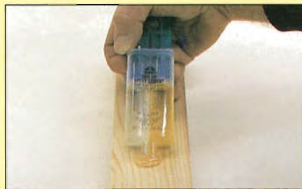
Photo D: Epoxy is widely available in syringe-type dispensers that help ensure a 1:1 mixture of resin and hardener.
