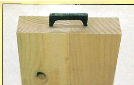
Photo X: Pinch dogs (Lee Valley Tools) come in different sizes. They can be used across any glue joint regardless of the shape of the two pieces.
