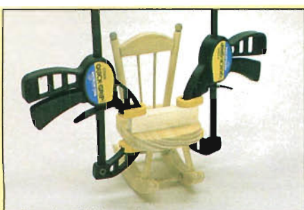
Photo U: To assemble this tiny rocking chair, I used the ultralight Micro Bar Clamp/Spreader by Quick-Grip (American Tool).
