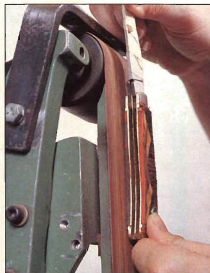
Photo O: Using a 100-grit belt, carefully sand insert faces nearly flush with bolsters to remove excess epoxy, wood, and turquoise.
