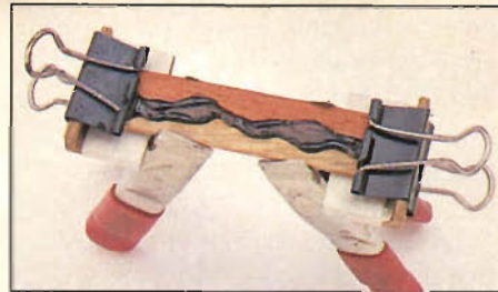
Photo J: Epoxy and spring-clamp the mountainscapes, using binder clips and scraps of laminate on the ends to keep them flat.
