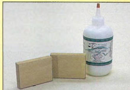
Photo C: There's no glue failure here. When the joint was broken apart, the acrylic resin adhesive pulled the melamine surface with it.
