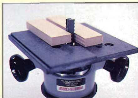
Photo L: Porter-Cable's Tru-Match system (shown upside down) includes models 42190 (subbase) and 43692 (bit). Look closely at the subbase and notice the two different levels this gives the true match you'll need. If you plan to use such a system, purchase an extra base so you don't have to keep changing the subbase.
