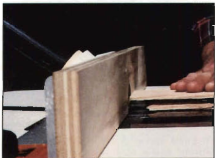
Photo A: Profile 1 bit cutting drawer front. Note that a rabbet must be cut around drawer face to the same depth as the joint. Make several passes, resetting fence to reach final depth.
