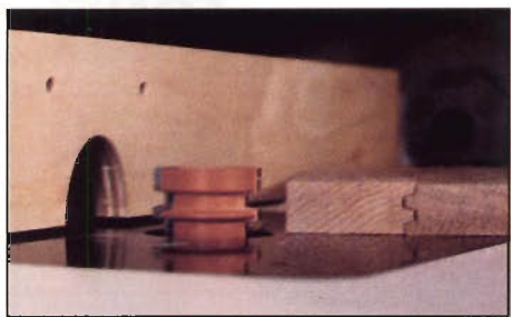
Photo E: Profile 1 bits will also cut edge joints that enhance the strength of edge-glued panels. For this purpose, adjust depth so bit centers on stock, then run one piece faceup, the next facedown.
