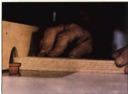
Photo B: Profile 2 bit cutting drawer front. Use a backing board behind the part to minimize tearout and provide stability. Make several passes, resetting the fence to reach the required depth.
