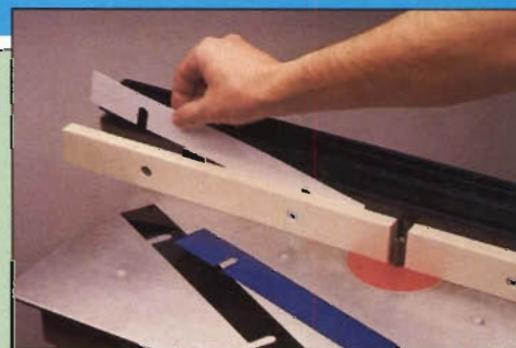
Photo I: Veritas offers an optional set of plastic shims that let you offset the two subfences for basic jointing.
