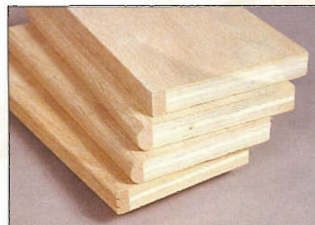
Photo H: Nosings made of \frac{1}{4} " or \frac{1}{2} "-wide hardwood strips make durable edges. Shape them before or after application.
