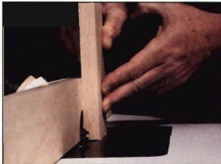
Photo C: To cut the drawer sides with a Profile 1 bit, stand the parts on end with the inside face against the fence. Use a backing board to minimize tearout and increase stability.
