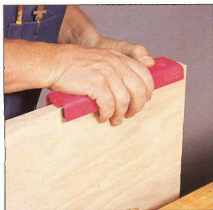
Photo G: Trim the edges of the banding flush with the panel's faces. Here author uses a single-edged trimmer.
