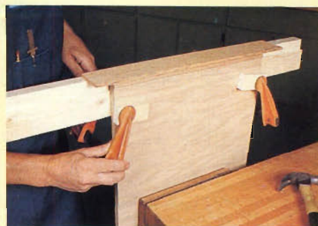
For quick, easy alignment of 2x4 router support with workpiece, tack a piece of 1/4" plywood to top edge of 2x4; align and clamp 2x4, then remove plywood strip before flush-trimming.
