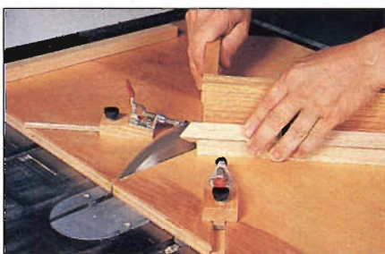
Photo N: To miter the ends, author uses a small V-block to hold the edging at the correct angle.
