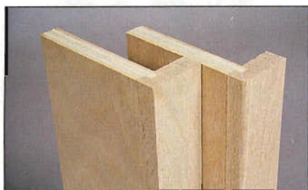
Photo R: Hardwood edgings applied to cabinet sides form a face frame that also conceals plywood edges. Both a square and a radius corner are shown here.
