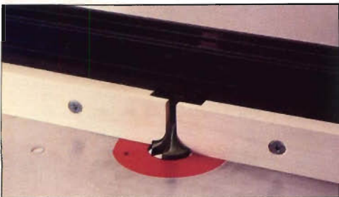
Photo C: On several tables (including the Veritas shown here), you can attach wood subfences for zero-clearance routing. Note how the subfences conform precisely to the router bit.
