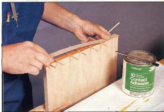
Photo D: Use contact cement to adhere plain-backed tape. Author inserts small wooden strips to prevent contact between surfaces before positioning the tape.
