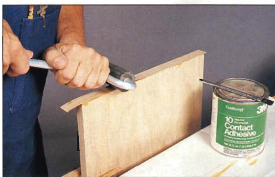
Photo E: Roll the banding with a veneer roller to remove air bubbles and ensure good contact between tape and edge.
