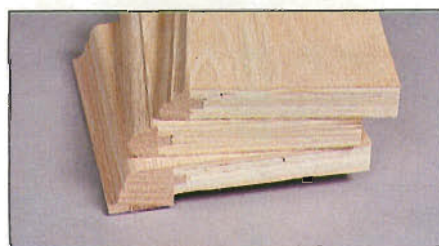
Photo U: To avoid clamping difficulties with shop-made molded edging, author suggests attaching the edging to the panel first, then molding it to shape.
