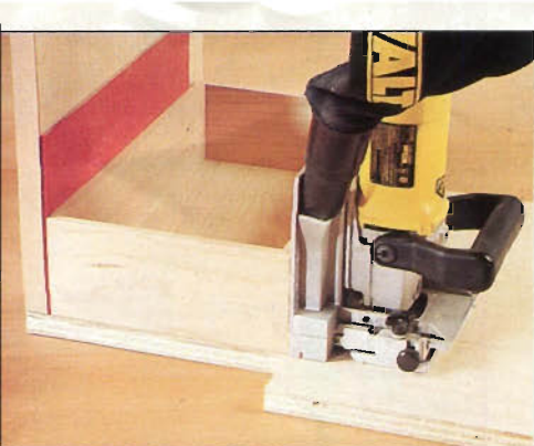
Photo B: Use a drawer and a \frac{1}{8} "-thick spacer as a fence for the plate joiner.
