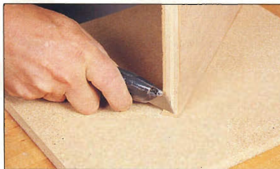
Photo F: Trim the end of the banding with a sharp utility knife. Tape will cut cleanly across the grain.
