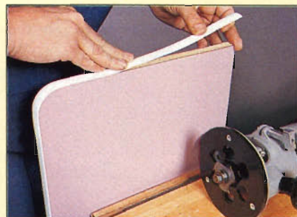
Photo R: For plastic T-moldings, cut a \frac{1}{16} " slot along the panel edge, then press barbed tongue on molding into the slot.
