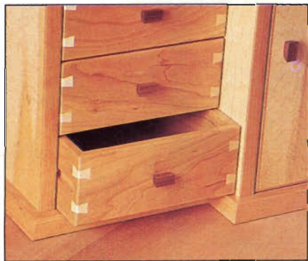
Photo A: Note corner keys, pull, and runner groove on the bottom drawer. Dimensions allow 1/16" clearance on all sides of each drawer.
