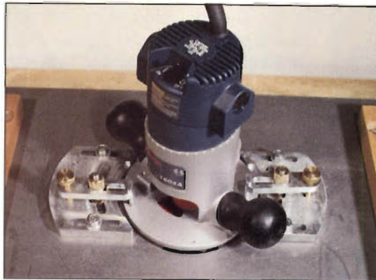
Photo A: Unique router clamp on the Veritas table top enables you to attach and detach router quickly without using tools or removing the router subbase.
