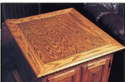
Photo P: Wide edging with mitered ends enhanced by small groove at the glue joint produces a framed effect on this cabinet top.
