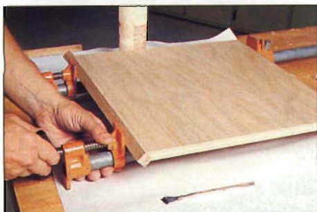
Photo J: Trim a corner of the hardwood blank to keep it from bottoming out, then glue and clamp the square into the V-groove.
