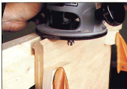
Photo K: Using a router and a piloted flush-trim bit, trim the hardwood edging flush with the plywood panel faces.
