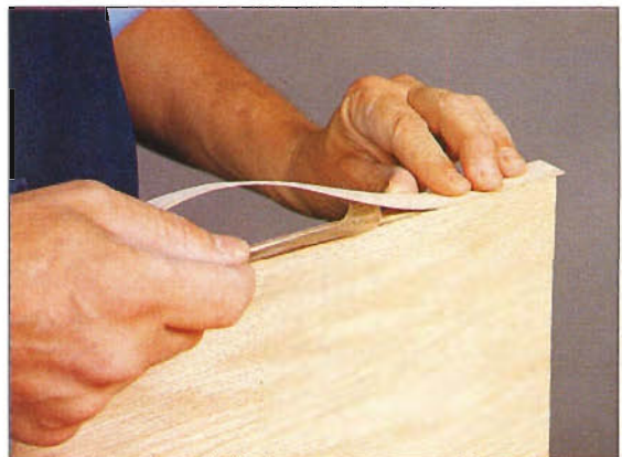
Photo B: To apply self-adhesive tape, peel off the protective paper backing and press the tape into position.
