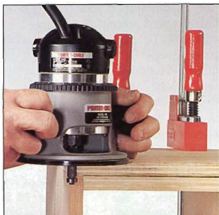
Photo C: Use the sides and dividers as a pattern for flush-trimming the base cutout.
