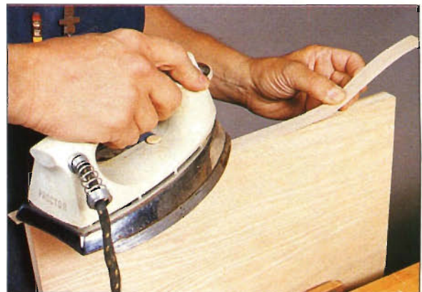
Photo C: Tape with heat-activated backing requires heat to melt the adhesive. Here, author uses a household iron on high (cotton) setting.
