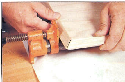
Photo M: Miter the ends of the hardwood squares, test-fitting them as you work.
