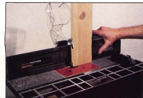
Photo D: Sears "unitized" fence incorporates a sliding push-shoe clamp for safer, more stable routing of board ends.
