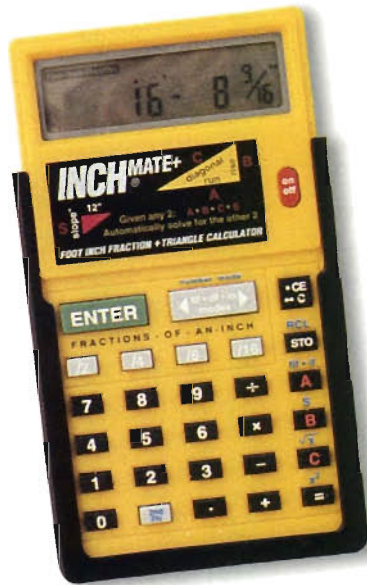
Photo A: The InchMate+ will instantly solve right-triangle problems. The simple but straightforward key pad and prompting display take only a few minutes to figure out.
