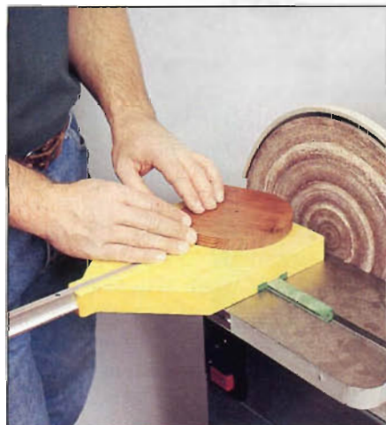
Photo B: The EZ load also works on stationary disc sanders that have a \frac{1}{4} " miter-gauge slot. Secure it as you do to the bandsaw, position the workpiece against the sanding disc, turn on sander, and then rotate the workpiece.
