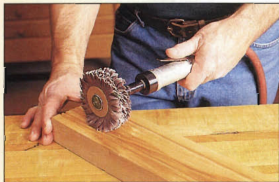
Photo B: Sand the carved rail texture to give it a smooth, worn feel. Dynabrade air sander with 180-grit flap sander is shown here, although a portable electric drill and flap sander would also do nicely.
