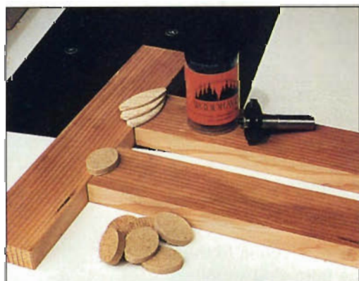
Photo B: Woodhaven makes its "Itty Bitty" biscuits from \frac{1}{8} " hardboard. The firm also sells Baltic birch plywood plates sized to fit its slotting cutters.
