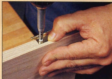
Photo R: To center and drill screw holes in one step, use a Vix bit.
