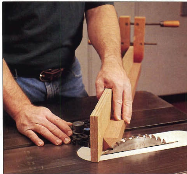
Photo B: Repeat 60° miter cuts to form point on top end of each leg.
