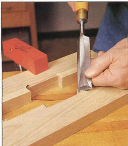
Photo E: Use sharp chisel and shearing motion to square the chamfer corners on spindles and rail trim. At each corner, cut end grain first, then long grain.
