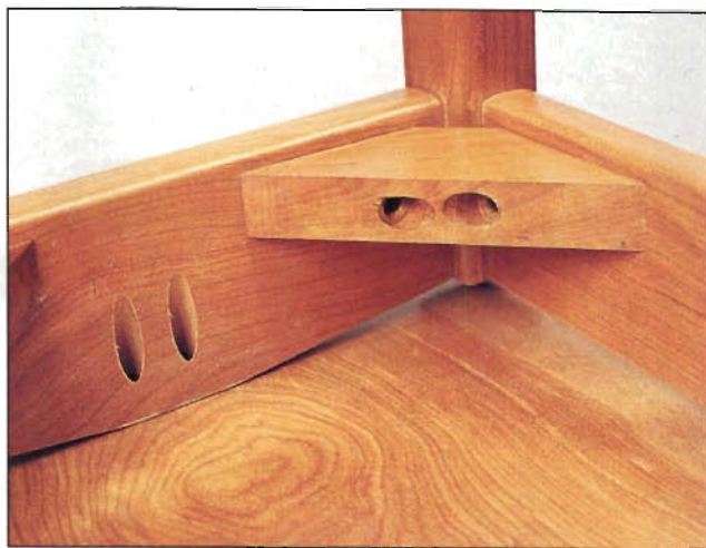
Photo D: Locate corner braces low on aprons so they won't be visible through the gap.
