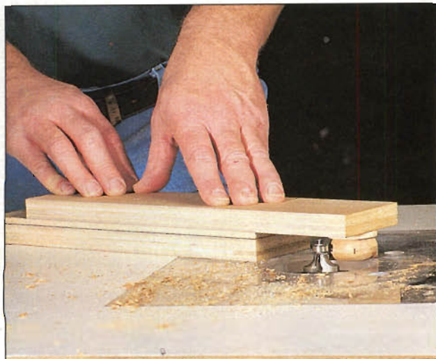
Photo C: Use this jig to safely round over both edges of the feet.
