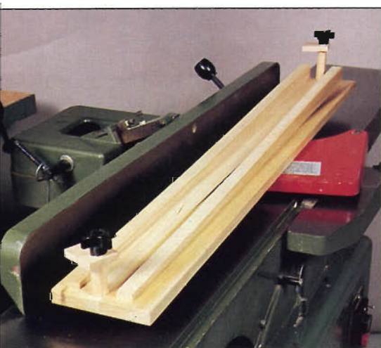
Photo A: Tapered strips glued to the inside face of the auxiliary fence automatically place it at an angle to the jointer fence, altering the line of feed to less than 90°.
