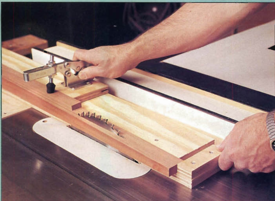
To cut second taper, rotate piece 90° and reclamp using waste from first cut as a clamping block.
