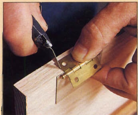
Photo H: Using a utility knife, scribe the outline of the hinge. Note shim behind leaf.
