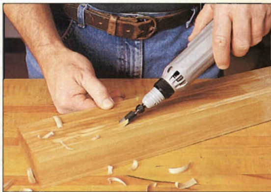
Photo A: To streamline the rail texturing, use a reciprocating power carver. Vary the cuts in depth and length, but keep \frac{1}{8} \times 1 " as the "nominal" dimensions.
