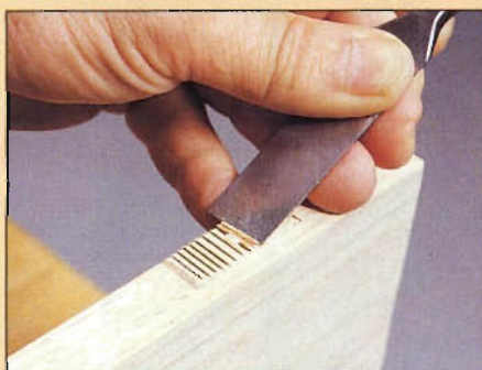
Photo P: To remove the chips, hold the chisel bevel side down and adjust the angle as you cut to keep the bottom of the gain flat.
