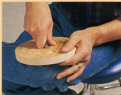
Photo A: To keep the chip-carving knife oriented at the proper 65° angle, wrap fingers around the back of the knife handle, using thumb to brace knife against workpiece.
