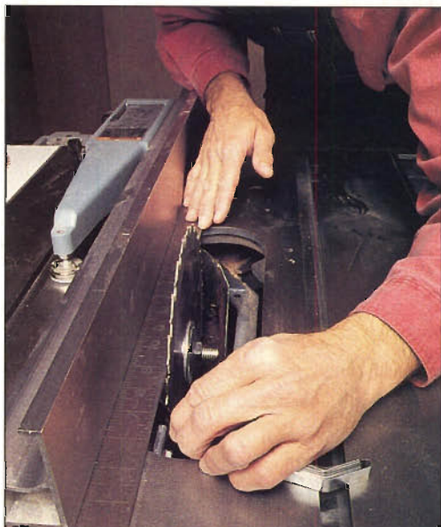
Photo O: To align rip fence with blade, raise blade to full height, place straightedge between the fence and blade, then adjust height until straightedge contacts a tooth at front and back edges of blade.
