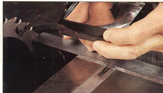
▲ Photo K: To check alignment of blade with miter-gauge slot, measure distance between tooth and miter-gauge centerline with tooth positioned "up front." Measure again at rear edge of blade using the same tooth. A magnifying glass makes precise readings easier.
