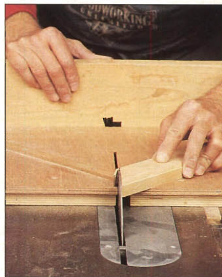
Photo M: With arbor aligned with slots, jigs and cutoff sleds will make clean cuts with blade at 90^\circ , but axis of tilt still needs to be aligned with table.
