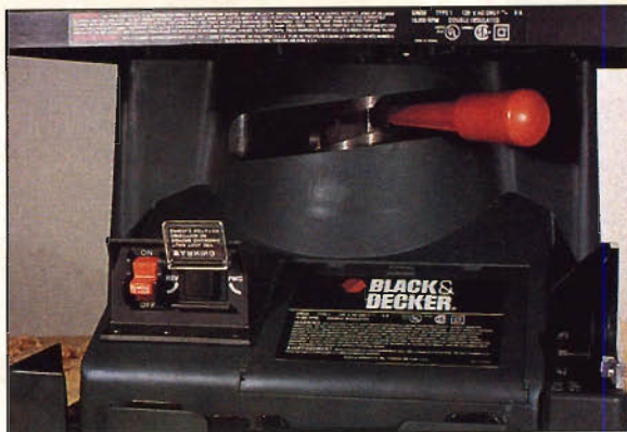
Photo A: The Black & Decker features an easily accessible "twist to lock" handle for adjusting spindle height. Other handy features include a separate forward-reverse switch and onboard storage for wrenches and miter gauge.
