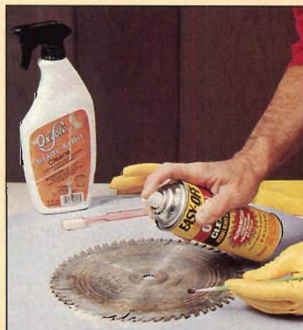
Photo E: Pitch-covered blades cause almost as much trouble as a misaligned saw. To remove, apply a blade-cleaning product or oven-cleaner, then scrub with a toothbrush.
