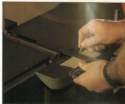
Photo E: Clamp the cutter head at top of cutting arc, then apply masking tape where shown. Use combination square to mark the forward edge of knife slot on tape.
