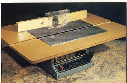
Photo F: Delta's optional table extension comes in handy when shaping long boards or large panels.
