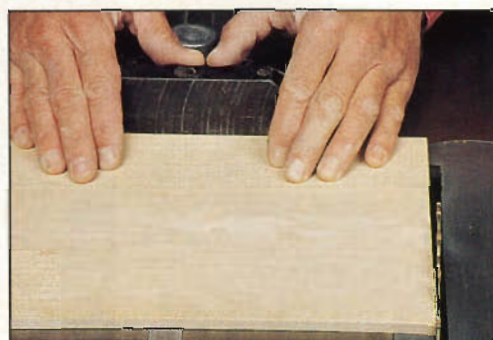
Photo H: If the blade does not align with miter-gauge slots, miter gauge will push workpiece into or away from the blade while moving it forward.
