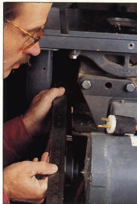
Photo B: Using a straightedge, align arbor and motor pulleys to make them coplanar.
