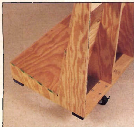
Photo A: Secure casters to base using \frac{1}{4} \times 2 " carriage bolts. Locking casters make loading/unloading rack much easier.
