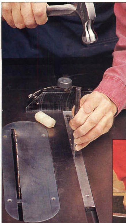
▲ Photo J: Take the "slop" out of the miter-gauge bar by centerpunching the bar at several points along both edges to bulge steel outward.
