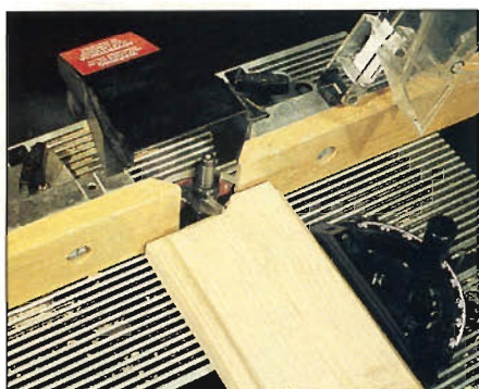
Photo E: A few operations call for a miter gauge, such as shaping the end of a board (Delta shown). This nice, sturdy gauge from Delta fits the P-C as well and accepts an optional hold-down clamp.
