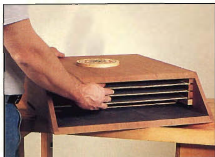
Photo C: The ceiling/partition subassembly slides into position between the side-mounted cleats (viewed from bottom). Simply remove the roof if partition repair is required.
