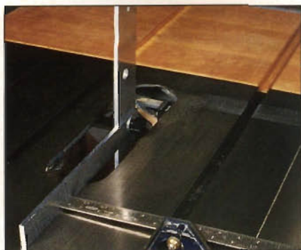
Photo A: Using the arbor and heel bars and a combination square to align the saw table with the saw arbor.
