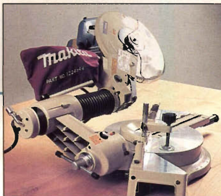
Photo A: The LS1211 is the only 12" sliding saw out there that can cut 60° left and right miters, 45° left and right bevels.
