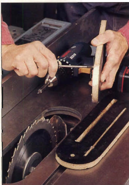
Photo R: Make custom throat plates by laminating countertop material to plywood or particleboard. Install #8x½" flathead screws in the underside to serve as levelers.
