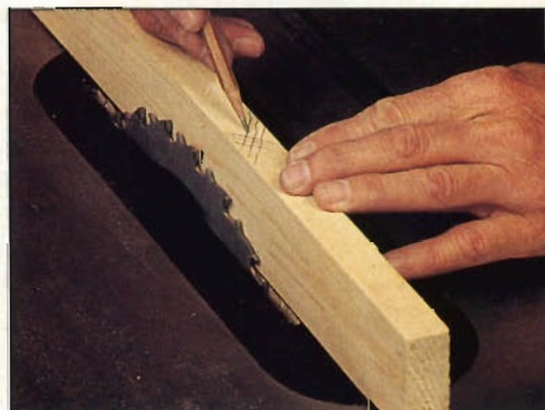
Photo I: A good cut (shown here) has half its tooth marks arcing upward and half arcing down. If downward marks predominate, the leading edge of the blade is set too far in. If most marks arc upward, the tail edge of the blade is doing too much of the work.
