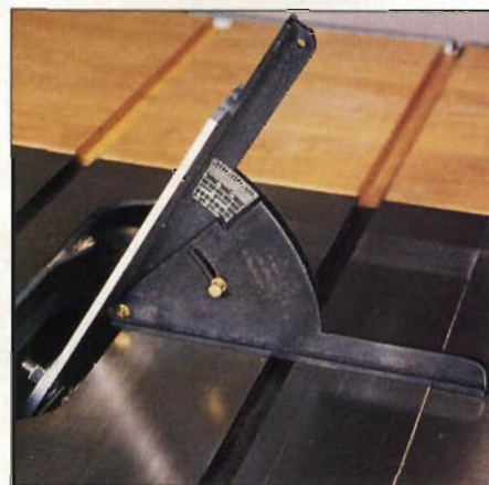
Photo C: Setting the bevel angle using the arbor bar and "A"-Justable Square.
