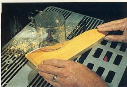
Photo C: To do freehand or curved shaping, remove the fence and insert a starting pin in the table. After you start a cut, the shaper collar or pilot bearing supports the work. All machines come with plastic ring guards for this operation (B&D shown).
