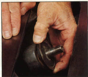
◀ Photo F: Check the condition of arbor bearings by wiggling and rotating the arbor. Listen and feel for rumble or stiff or sloppy action.
