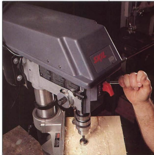
Skil HD3580 benchtop drill press features five speed options, a 6½" spindle-to-column clearance, a 9x9½" tilting table, and an optional column-mounted fence.
