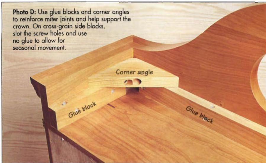
miter the front ends. Trim the back ends to length, then glue and clamp them to the front molding and crown sides only—not to the cabinet sides. Use glue sparingly and with care. Note: Gluing this strip to the case sides could cause the miter to fail when the wood expands.
