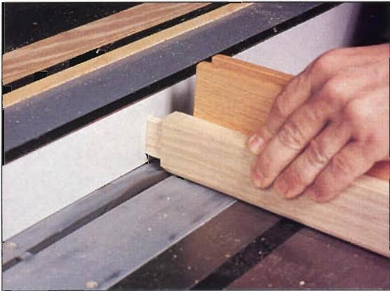
**Photo F:** Without changing blade setting, cut the same 45° miter across both ends of the rail sticking.
