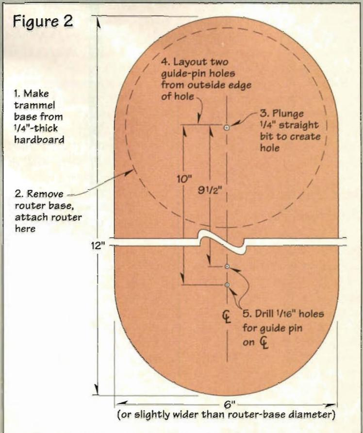
Switch to the 10" guide-pin hole on the base, and reattach it to the template blank. Before you start the router, position the bit just to the right of the centerline on the blank. Plunge in at this point, and rout to the left edge of the template blank.
