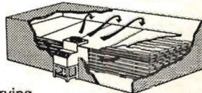
Our L-50 Kiln dries 300 to 1,200 BF. Your kiln chamber can be as small as 9' x 7' x 6'!
