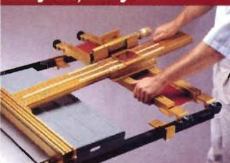
Dismounts for cross-cutting operations, and remounts in less than 10 seconds.
