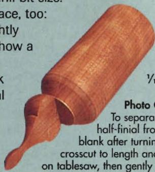
**Photo C:** To separate lower half-finial from split blank after turning, first crosscut to length and depth on tablesaw, then gently insert a razor blade between finial halves to loosen double-faced tape.
