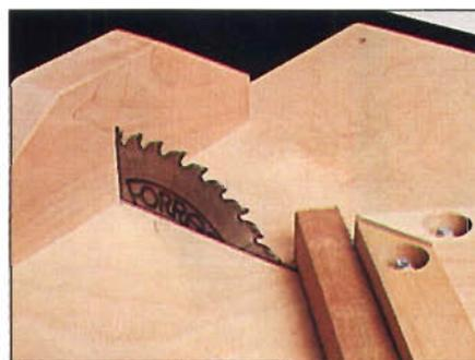
cernible resistance or slowing. On the smaller saws, switching to the thin-kerf blade allowed very similar feed rates, again with barely noticeable resistance.
