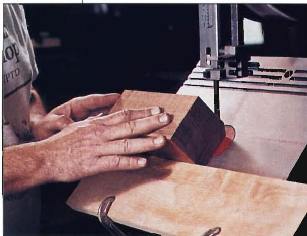
The 7" cutting height gives the Skil bandsaw good capacity.
