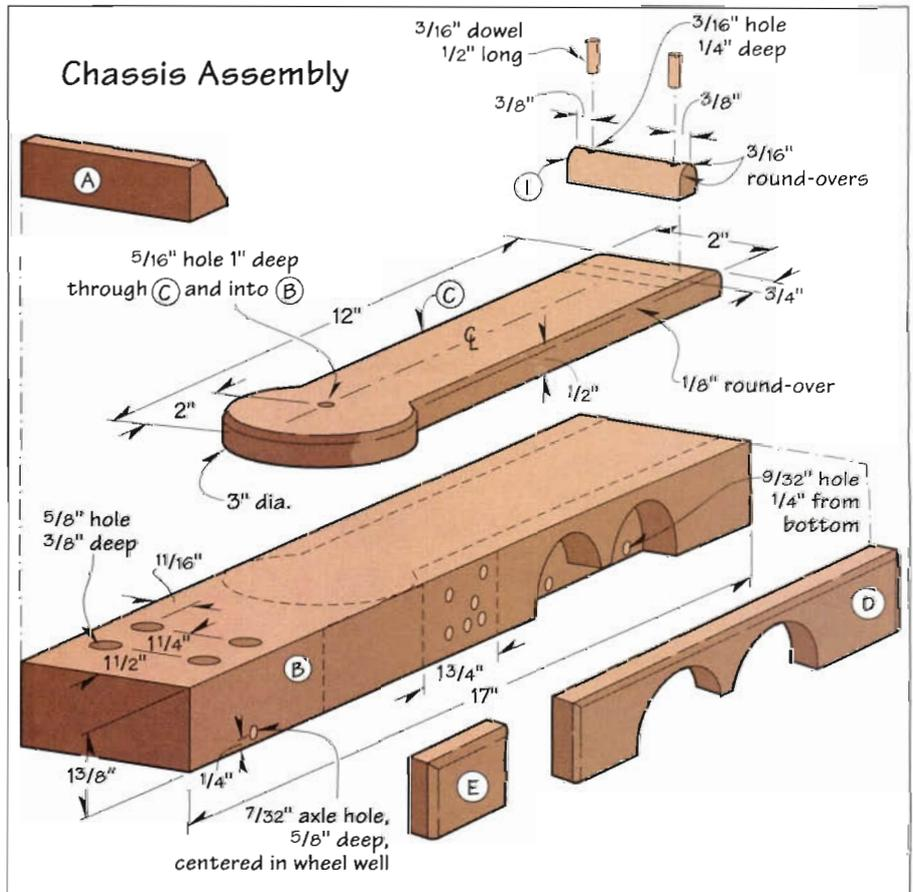
and locations.) Next, rout the front and back edges of each side, stopping the round-over  $\frac{1}{8}$ " from the bottom end of the front edge (where it joins the bumper).
