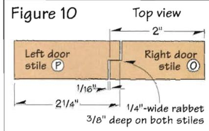
ary fence to your rip fence, then partially "bury" the dado head in it to leave  $\frac{1}{4}$ " of cutting width exposed. Elevate the dado to remove one-half the stile thickness. Cut a  $\frac{1}{4}$ "-wide rabbet along one edge of both inner stiles (P and one part O). This edge will become the back inside edge on the narrower, overlapping stile (O) and the front inside edge on the wider, overlapped stile (P).
