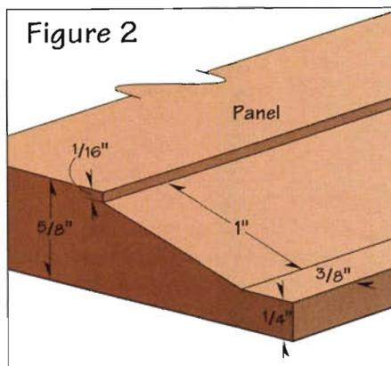
sion. Note: You may need to adjust rail length if your stile and rail bits cut a different profile from ours. To determine this, calculate the difference between the cope cutter diameter and its bearing diameter. The difference on our set was  $\frac{1}{16}$ ". If your set is more or less, adjust the rail length accordingly.
