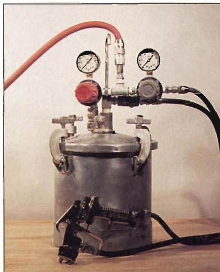
Most HVLP guns can be used with remote two-quart cups or larger paint pots, such as this 2 1/2-gallon Binks unit. The regulators and gauges control air and fluid pressures to the gun.
