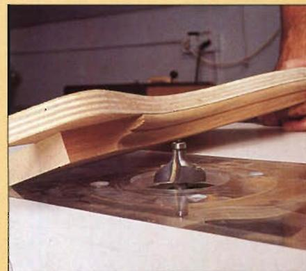
Photo B: After flush-trimming, rout profile on the crown molding using a large cove and bead bit.
