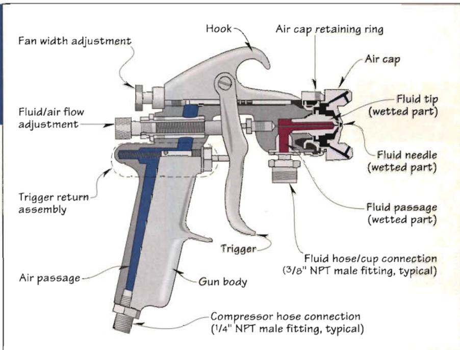
Conversion spray guns, as illustrated in this DeVilbiss cutaway, incorporate special baffles, enlarged air passages, and modified air caps to reduce the pressure and increase the volume of compressed air available for spraying.
