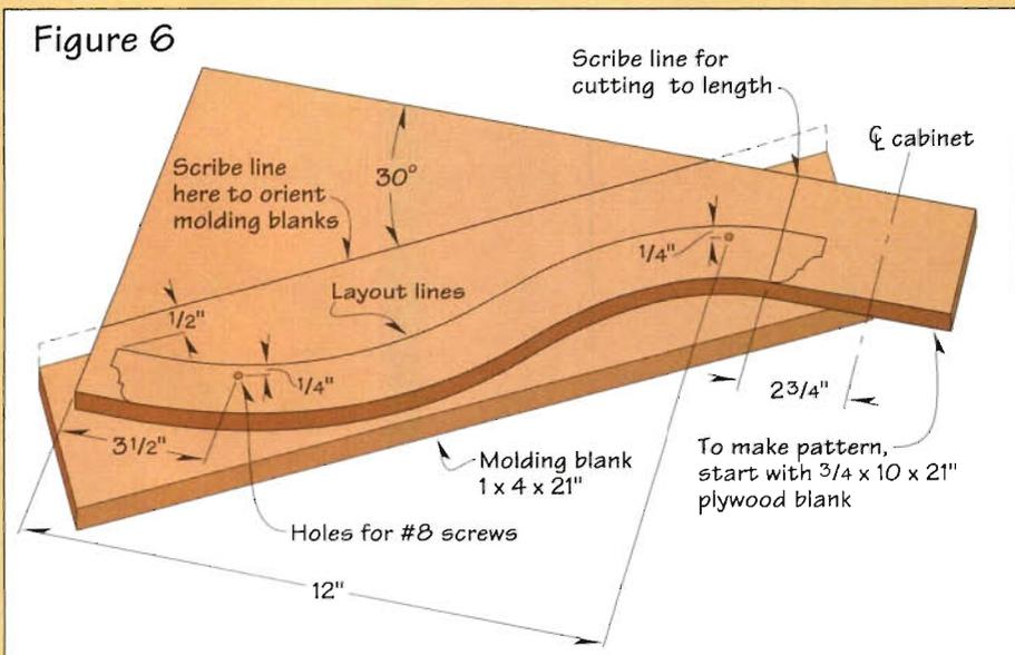
table-mounted router, rout the profile along one of the blank's edges. Rip a 1/4"-wide molded strip from the piece. Miter both ends. (These mitered ends will be used for the molding returns on the crown top.)
