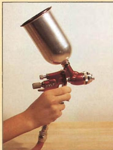
the 90P nozzle, the M1-G is even more air-miserly.) Using the standard setup, I had no trouble spraying my test finishes, although they went on at a slower rate than with the "high-volume" guns.
