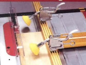
Universal T-Slots for hold downs or other fixtures on the front face and top of the fence
