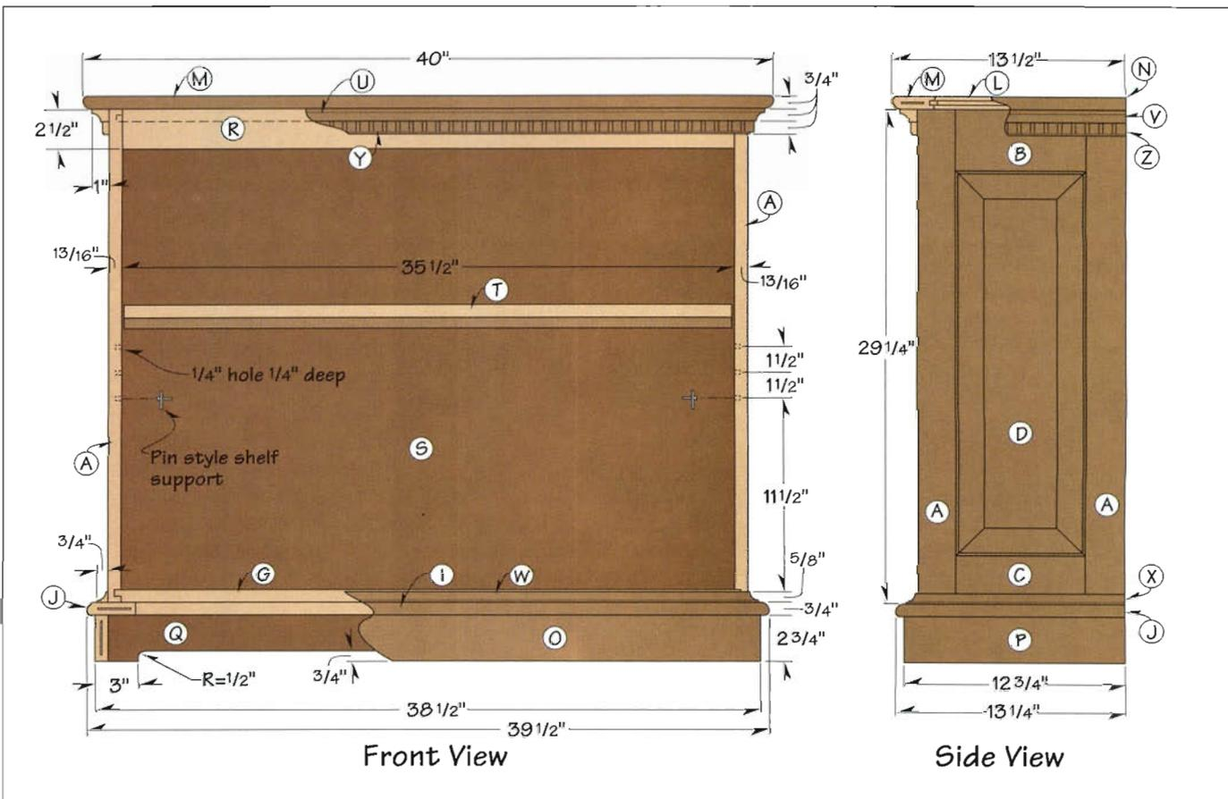
flush with the bottom edge of the side, so adjust the height of the dadoes to compensate for the actual thickness of your plywood. Also, the trim covers the top dadoes and nearly all of the bottom dadoes.
