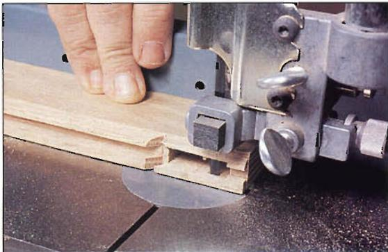
**Photo G:** Bandsaw away most of the waste sticking on the stiles, but keep the blade at least 1/16" from the shoulder.
