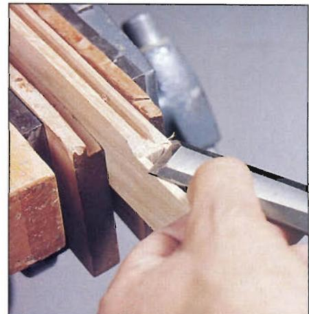
**Photo I:** After routing the remaining waste sticking, finish cleaning up the surface with a chisel.
