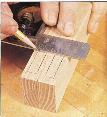
Photo A: Carefully lay out mortises on the edges of the stiles.
