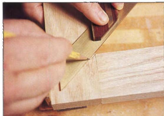
Photo D: Mark the position of the miter cut on the stile, then lay out the  $45^\circ$  angle from the mark.
