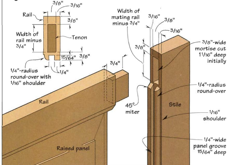
**Step 5.** Without moving the rip fence, raise the blade to cut  $\frac{3}{8}$ " deep. Then, make the shoulder cut on both rail edges on each end (*figure 4*).
