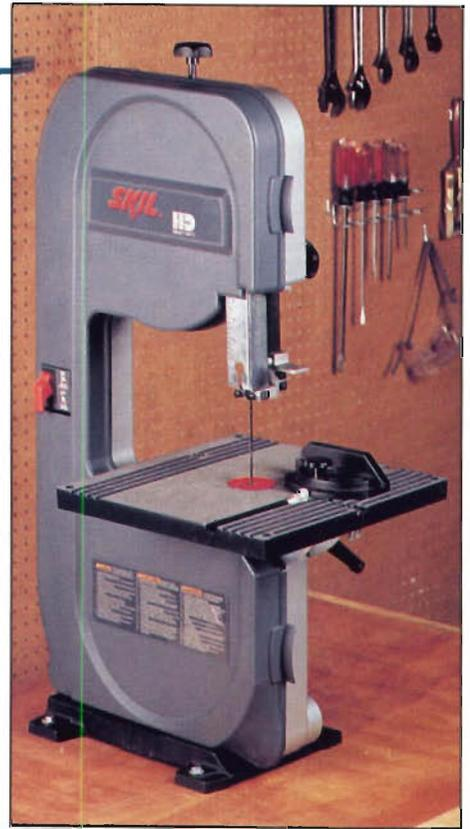
Skil HD3640 benchtop bandsaw features 10" throat depth, 7" cutting height, and a 13 $\frac{3}{8}$ "-square table. The saw requires less than two square feet of bench space.
