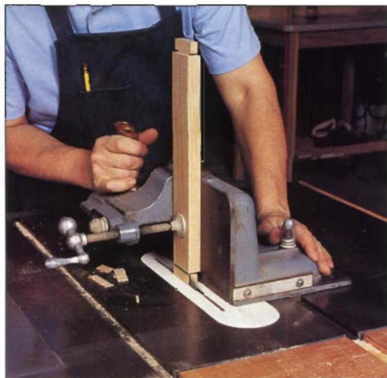
Photo B: A tenon jig allows accurate cutting of the cheeks on the rail tenons.
