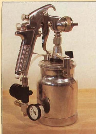
As with the other guns, you can adjust the pattern size and material flow on this model to do fine detail work and small projects. However, like the other guns with full-sized cups, it's a bit too bulky to allow precise control. (See the DeVilbiss EGHV comments).
