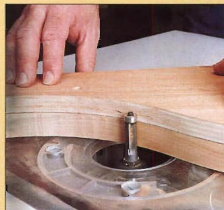
Photo A: Bandsaw outside the line, then attach pattern and flush-trim the edge of the crown molding to shape.
