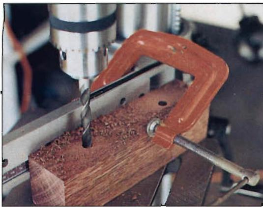
The optional fence accessory attaches to and pivots from the column. It proved an excellent addition, especially for operations that required clamping.
