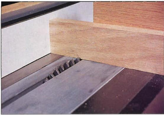
**Photo E:** Set up the tablesaw and cut a 45° miter across the stile sticking where marked.
