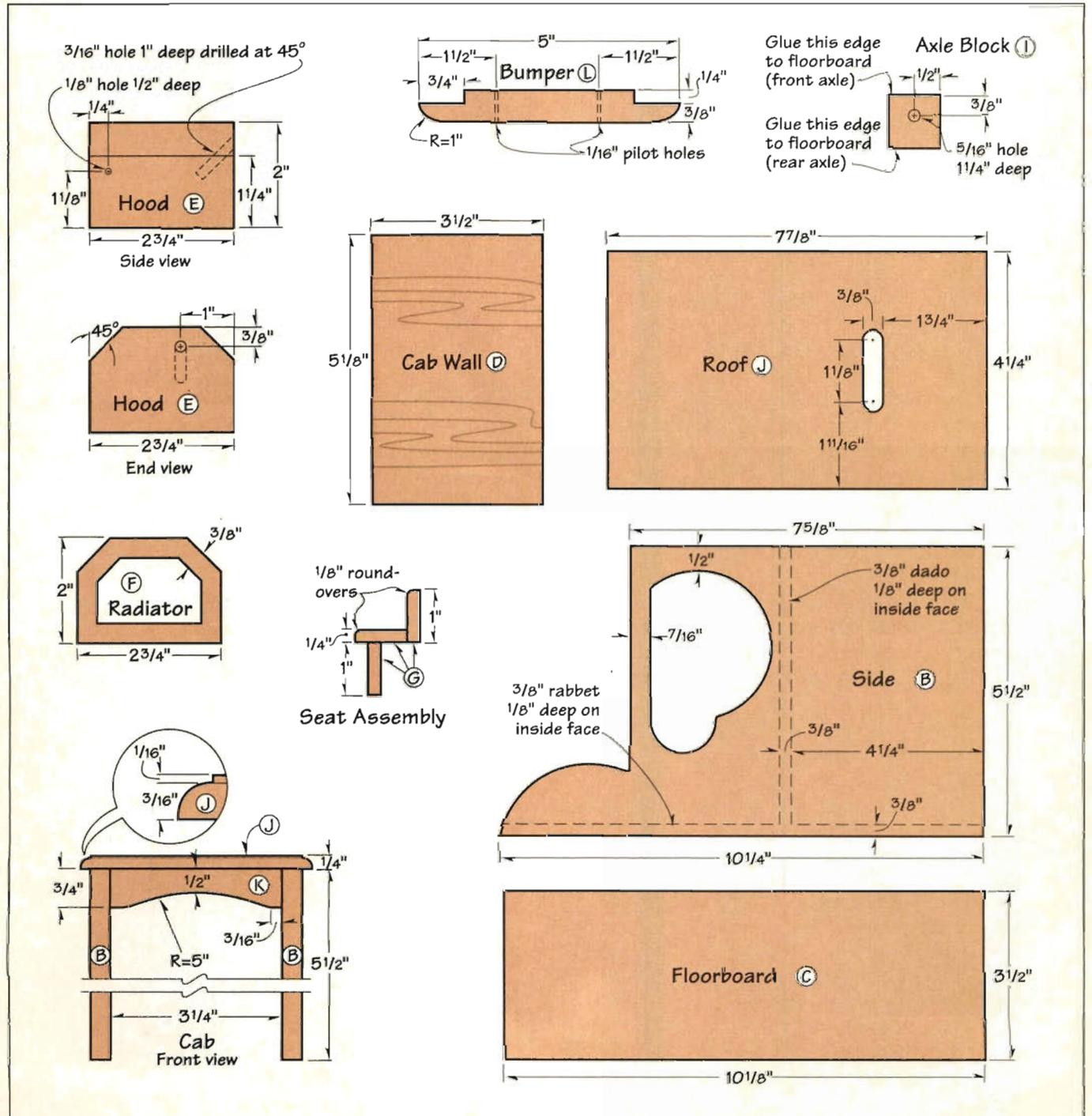
fence on your drill-press table, drill overlapping  $\frac{3}{8}$ " holes to rough out the slot. File or scrollsaw the slot edges flat, keeping in mind that this slot will be concealed by the escutcheon plate. Now, finish-sand the roof.
