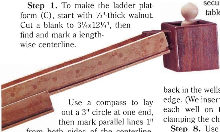
Use a compass to lay out a 3" circle at one end, then mark parallel lines 1" from both sides of the centerline, stopping at the circle. (See the Chassis drawing.) Bandsaw the platform to shape, keeping the blade outside the line, then sand to the line.
