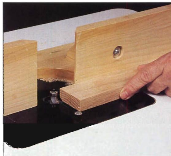
Photo C: Using a  $\frac{1}{4}$ " round-over bit, rout the sticking profile on the inside edge of each rail and stile.
