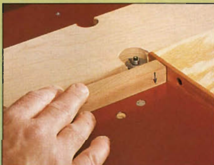
Photo C: Use same setup (with shim still in place) to slot stile edges for bottom-rail joints.
