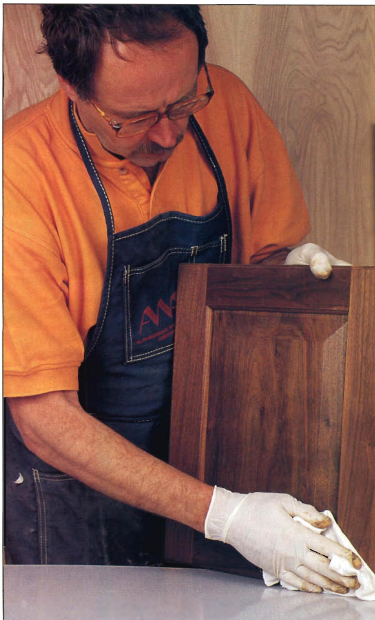
For color uniformity, author prestains walnut sapwood first, then overcoats entire panel with oil stain, wiping off excess with a lint-free, absorbent cloth.
