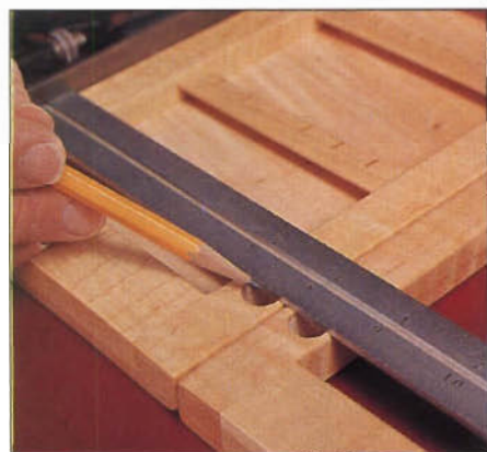
Photo G: To lay out mating hinge holes accurately on adjacent frames, use combination square to establish hole location vertically.
