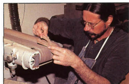
Photo D: Using the roller on a stationary belt sander, bevel the interior edges of the sky and planet sections.
