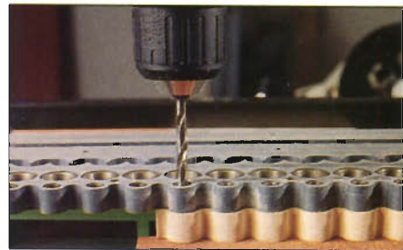
Photo F: Drilling pin holes (centered in crescents) in ends of drawer sides using brad-point bit and portable drill.
