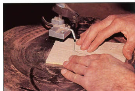
Photo B: Transfer the landscape pattern to the face of the stacked pieces, then scroll saw the sky, planet, and canyon sections to shape.
