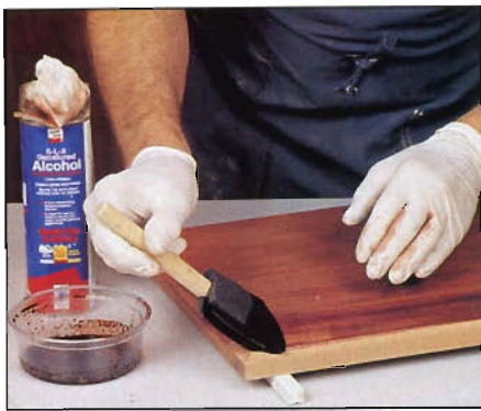
Photo G: To apply water-based stains, use a foam brush, dampening just the tip and following the grain. Avoid overlapping, but use an alcohol-dampened rag to blend streaks where you do overlap.
