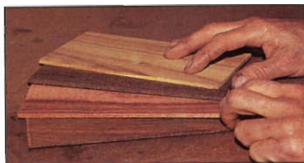
Photo A: To create the bottom puzzle layer, select four contrasting woods, then align and stack them using a drop of epoxy at each corner.
