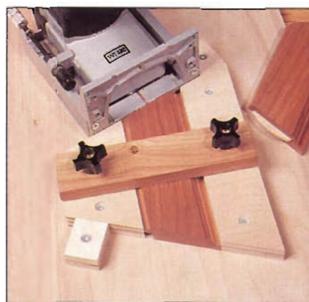
Photo A: Use the slotting jig to ensure accurate slots on mitered ends of frame parts
