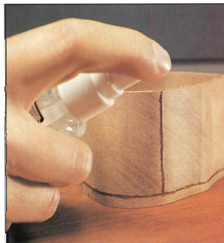
Photo F: Use medium-grade, gap-filling CA to close entry/exit kerf in bandsaw box. Apply CA along kerf, close joint with hand pressure, then spritz with accelerator.
