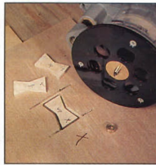
Photo E: To cut out keys, remove spacer ring from guide bushing, reset cutting depth, then rout.
