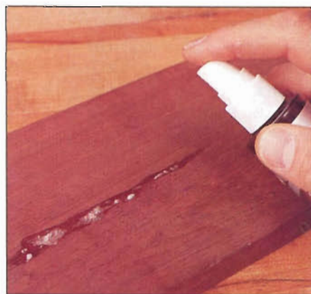
Photo B: Spray-on accelerator causes slow-cure CAs to bond instantly, but too much of it can leave an unsightly white residue that's difficult to get rid of. Accelerator "overdose" also can weaken bond, make it more brittle.
