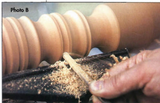
The Ryobi lathe handles spindles up to 18" long, plates up to 10" in diameter, and accepts standard spur centers, face plates, and chucks. The author especially liked the unit's variable-speed control feature.
