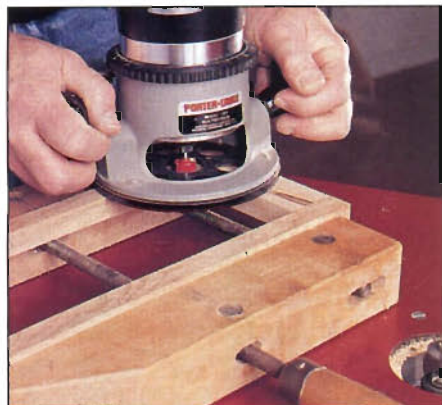
Photo F: Dry-clamp frames using large handscrew, then rout \frac{1}{8} " round-over on inside frame edges.
