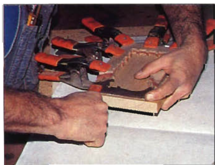
Photo K: Glue and clamp frame sections to backing, then square and trim using table- or radial-arm saw.
