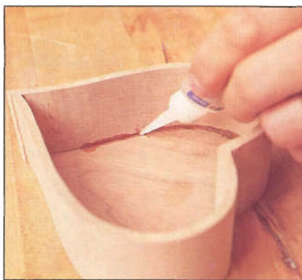
Photo G: To create reinforcing fillets along butt joint, apply bead of slow-cure CA, then spritz with accelerator to "tack-weld" parts.
