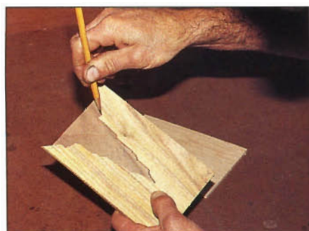
Photo F: To lay out middle and top canyon layers, either follow the patterns, or trace the outline of the preceding layer onto contrasting stock, then draw a slightly lower and wider contour (outside the traced line).
