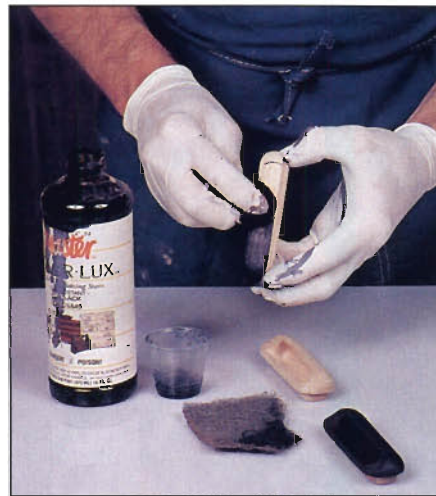
Photo E: Use a solvent-based jet-black stain for ebonizing. Here, author applies several coats of Behlen's to maple drawer pulls, scrubbing between coats with a purple Scotch-Brite pad.
