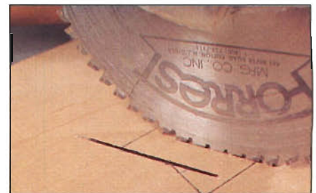
Photo B: Cut out the interior waste from the template. We cut ours by making plunge cuts with a sliding compound miter saw.
