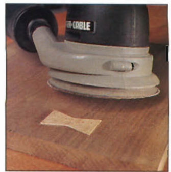
Photo F: After gluing keys in sockets, carefully sand them flush with the surrounding surface.
