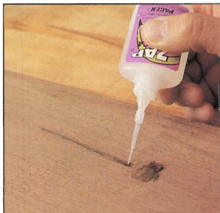
Photo E: To fill surface check neatly and invisibly, pack check with sanding dust, then apply just enough low-viscosity CA to saturate dust.
