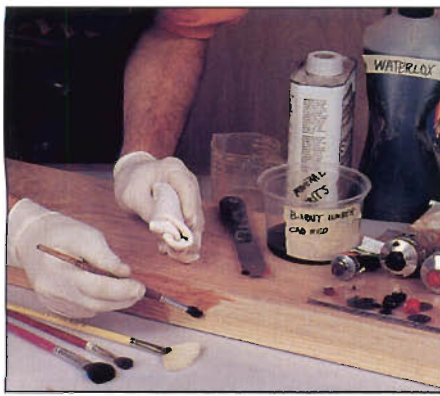
Photo C: To make your own stain, start with a half-cup of clear oil finish (Waterlox in this example), then add small quantities of artist's oils to fine-tune the color.
