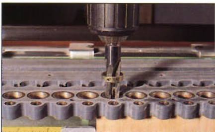
Photo C: Portable drill and tenon-cutter complete the fully rounded pins.
