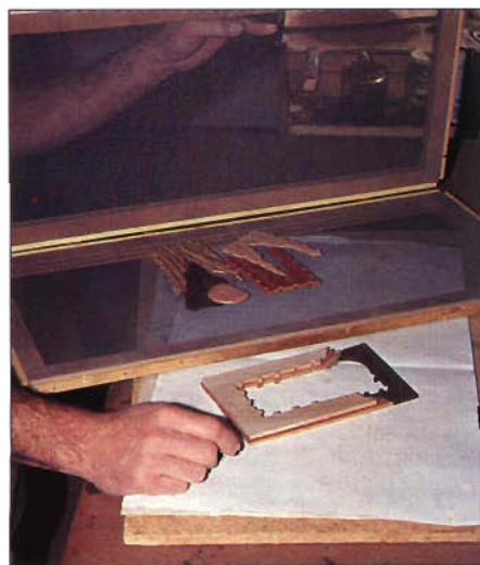
Photo J: After finish-sanding, blow dust off pieces using compressed air and a hinged sandwich screen.
