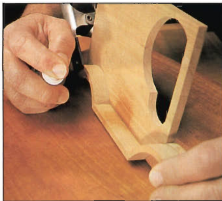
Photo C: Thicker, slow-cure formula works best for attaching small, fragile hardwood parts. To speed curing, spritz joint with accelerator after gluing and positioning.
