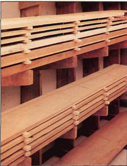
Photo B: Store lumber on flat, level supports well off the floor with evenly spaced stickers to ensure air circulation between boards.
