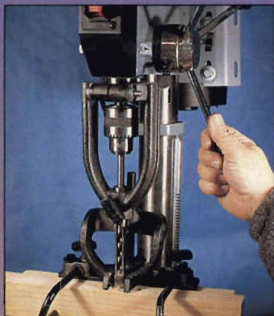
Photo C: The AMT drill-press mortising attachment can be fitted to almost any brand of drill press. This model accepts chisels with 3/4"-diameter shanks.
