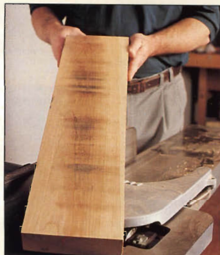
Photo E: To eliminate a mild case of cup, first joint a solid end-to-end "hit line" on the hollow (concave) surface, as shown on this piece of 8/4 cherry. Move to the surface planer, plane the crown flat, then finish flattening the hollow.
