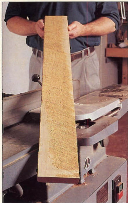
Photo F: A board suffering from twist is the hardest to salvage. Start with the hollow, jointing diagonally opposite corners flat. Next, surface-plane the crown flat, then the hollow.
