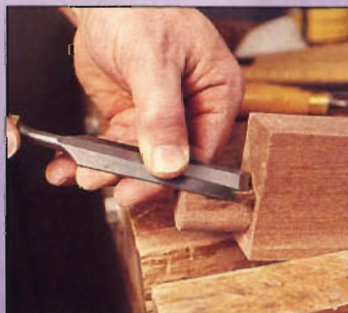
Photo E: Remove the waste left at the shoulders using a dovetail saw and chisel.
