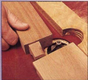
Photo C: Use a couple of different fence and stopblock settings to rout the tenon round.
