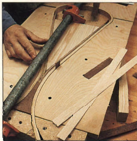
Photo F: Dry-clamp yoke/wedge lamination, and shim any small gaps around form.
