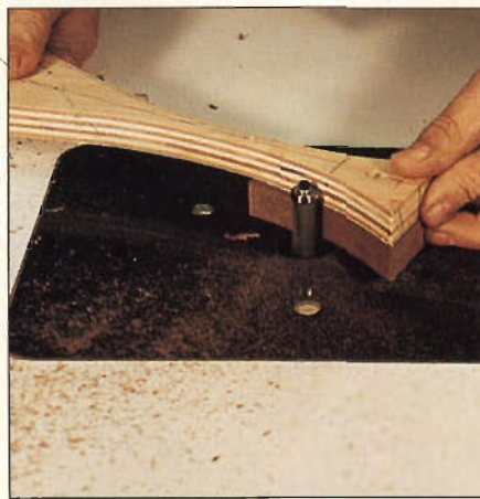
Photo E: Use center gluing form as template to shape handle insert, then flush-trim on router.
