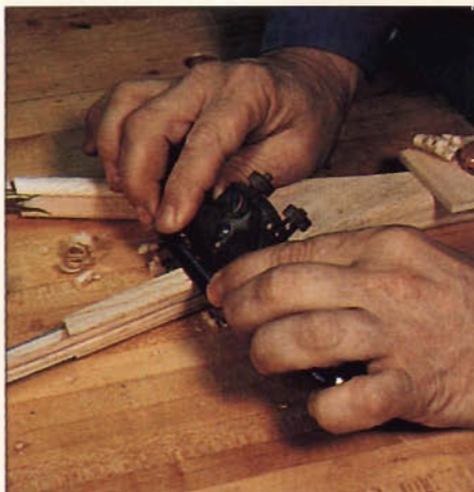
Photo I: Use spokeshave to taper thickness of handle cap down to hoop thickness.
