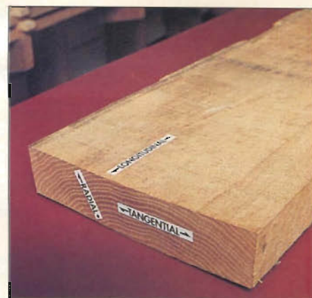
Photo A: The three axes of wood that pertain to grain direction and growth rings, labeled here on a slightly cupped, 8/4 red oak board.
