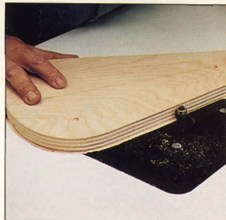
Photo C: Separate the center form from the router form, then flush-trim the form edges with your router.
