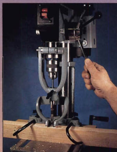
Photo D: The Reliant attachment accepts only chisels with 1/2" shanks. It comes with two sets of bushings to fit quill shafts on most drill presses.
