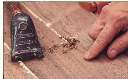
Photo A: Excess glue squeezed from a joint foams as it absorbs moisture from the air and cures. Once cured, the excess can be scraped. Note the nearly invisible glue line between the two pieces of unfinished walnut.
