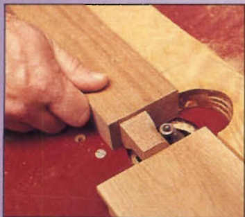
Photo D: On some tenon edges, you'll rout from the shoulder out to the end of the tenon.
