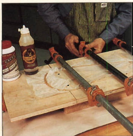
Photo D: Line the gluing form with waxed paper before laminating. Clamp the lamination as shown with pipe clamps.
