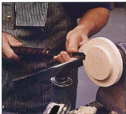
Photo N Using your parting tool, cut a lip into the backing block to accept the box.
