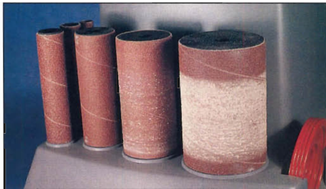
Photo 8: The Ryobi provides convenient on-board spindle and table-insert storage built into the base. The Sears model (not shown) provides a clip-on tray for these parts.
