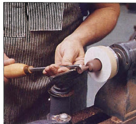
Photo P To form the knob, bore a 1 1/8" hole into the backing block, insert the blank, then turn the knob to shape.
