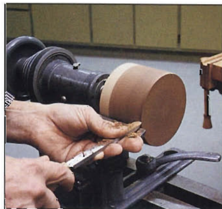
Photo B With a roundnose scraper, round down the blank before you form the box contour.
