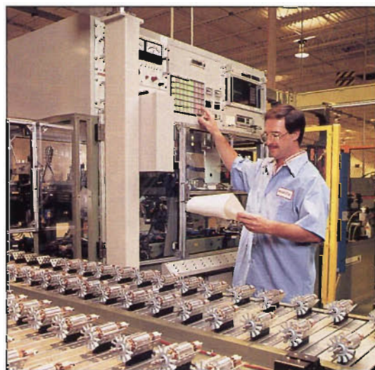
Automation helps some manufacturers hold down tool prices. Here, Clark Vaughters operates the final inspection station for motor armatures at Makita Corporation of America's highly automated plant near Buford, Georgia.
