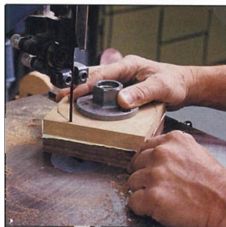
Photo A Bandsaw both turning blanks/backing blocks round. Note: We've raised the blade guide to better show the process.
