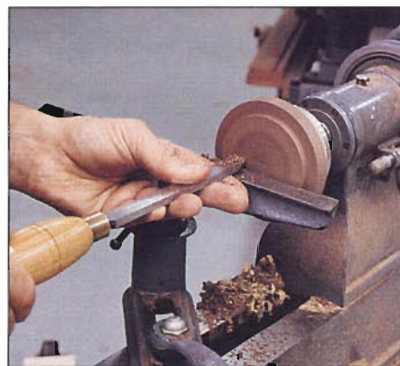
Photo I Shape the inside of the lid. For best results, work the gouge from the center to the outside edge.
