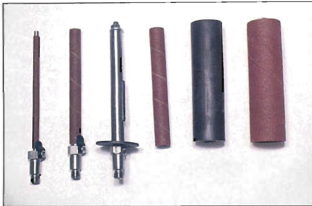
Photo 5: The Powermatic uses a combination of different spindles and drum sizes to accept 1/4"- to 3"-diameter sanding sleeves.
