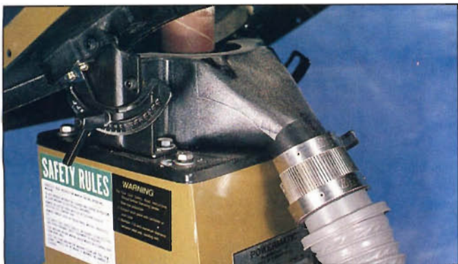
Photo 7: Undersized dust port on Powermatic makes connecting to 2 1/2" shop vacuum hoses difficult. Note the jury-rigged connection used by author during testing.
