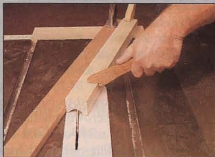
Photo C Set the blade \frac{1}{16} " above the saw table, then cut the cove. Raise blade in \frac{1}{16} " increments, repeating the cut until you reach \frac{1}{2} " depth.
