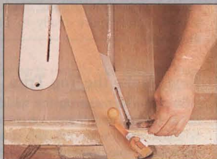
Photo B Using angle on bevel gauge, set auxiliary rip fence \frac{1}{4} " from exiting tooth on saw blade.
