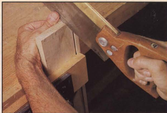
Photo M ▶ To form the pins and tail sockets, start with an angled sawcut as close to the knifed lines as you can get.
