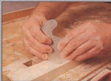
Photo D Remove machine marks from cove with curved, handheld cabinet scraper shaped to fit the cove contour.
