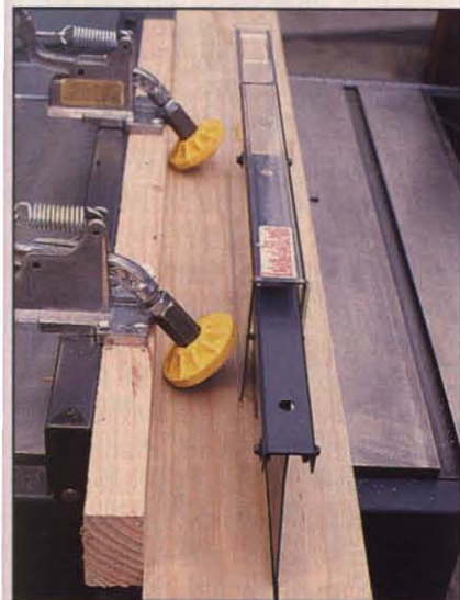
Photo B: The blade guard on most saws interferes with the outfeed wheel on all four hold-downs tested (as shown here with the Shophelper), limiting inboard rip cuts to a minimum of 3 to 3\frac{1}{2} " wide.
