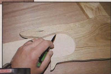
Photo 2 ▲ Scribing the neck profile onto the mating throat piece
