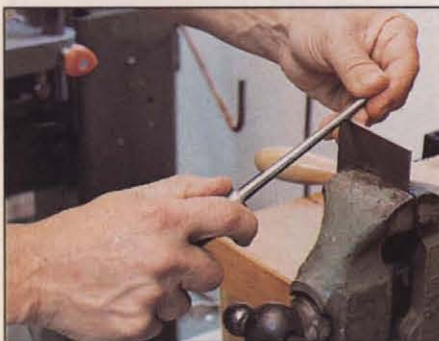
Photo D Applying uniform pressure, make several strokes across the edge with a burnisher held at a 75° angle to form the necessary 15° hook.
