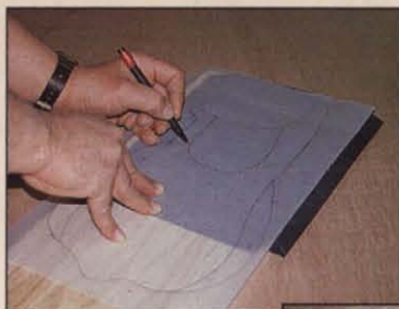
Photo 1 ▲ Transferring the neck pattern to the stock
