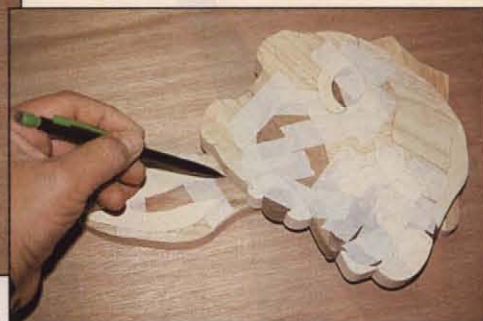
Photo 10 Tracing head outline onto mating ear
