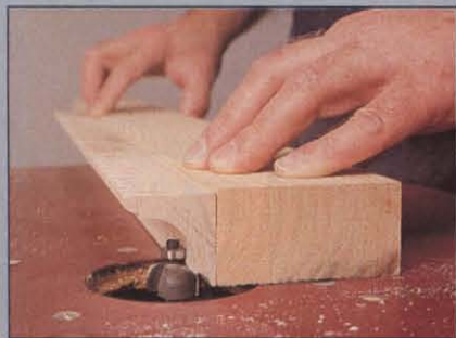
Photo I Using a \frac{3}{16} "-radius piloted cove bit, rout a shallow cove along the inside edge of the opposite corner of the workpiece.
