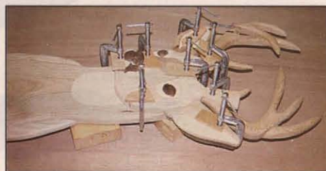
Photo 22 ▲ Clamping head to body while the glue dries
