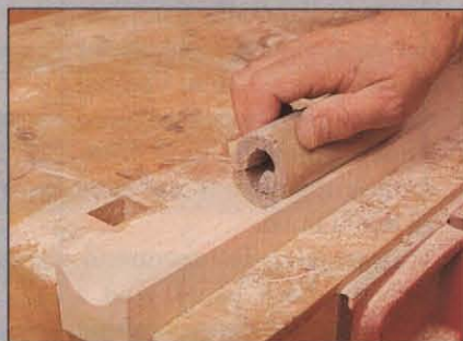
Photo E Wrap sandpaper around a cylindrical form (we used foam pipe insulation), then finish-sand the cove.
