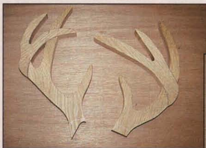
Photo 7 ▲ Antlers cut to shape with extra stock left at the head ends
