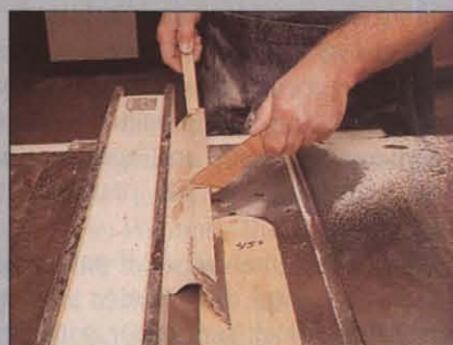
Photo F Place the workpiece cove-side down, then bevel-rip the lamination at 45° (along lines B-B') to remove the back corners or waste.
