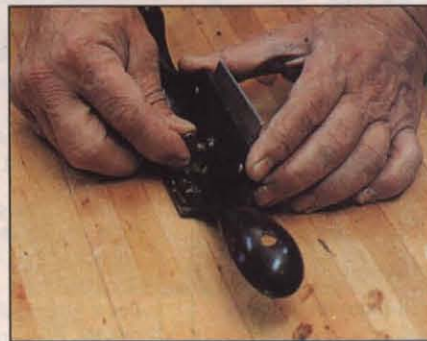
Photo F Insert the blade into the scraper body and tighten the clamp thumb screws. Turn the front thumb screw to adjust cutting action.
