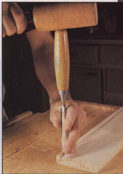
◀ Photos N and O ▲ N: Remove the bulk of the waste from the sockets by working down from the face and in from the end. O: Clamp the drawer front to your bench or work against a bench stop when chopping horizontally.
