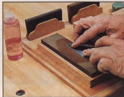
Photo E For fine work, carefully hone the edge and back of the blade after filing the edge. Then, burnish the edge to form the hook.
