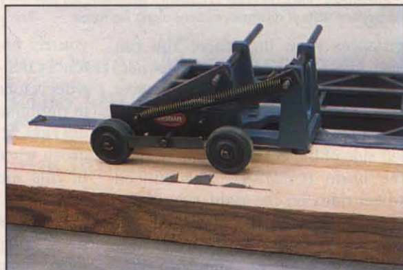
Photo E: Ripstrate includes both infeed and outfeed wheels in a single assembly. Short distance between wheels provides better support for ripping shorter lengths of stock.
