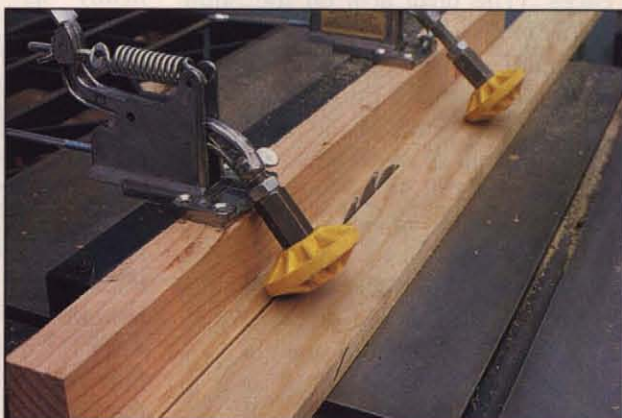
Photo C: With saw's guard assembly removed, Shophelper allowed inboard rip cuts as narrow as \frac{3}{4} ". By beveling the auxiliary wooden fence to provide clearance for the arm, you can move the wheel even closer to the fence, permitting \frac{1}{4} " widths.
