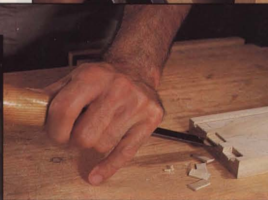
◀ Photos N and O ▲ N: Remove the bulk of the waste from the sockets by working down from the face and in from the end. O: Clamp the drawer front to your bench or work against a bench stop when chopping horizontally.
