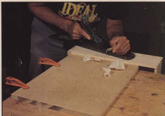
Photo S ▶ Resting on a piece of chipboard clamped to the bench, the faces of the drawer sides, front, and back are well supported for planing during fitting.
