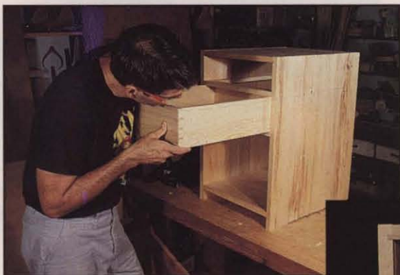
Photo T ▲ Fitting requires patience and repeated trips from the bench to test-fit the drawer in the opening.
