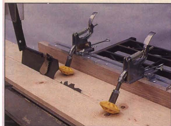
Photo A: On Shophelper, infed wheel (foreground) is positioned to left of cut line, outfeed wheel to right of cut line. Optional 24" track attached to auxiliary fence enables you to position units at different positions along the fence.
