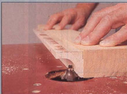
Photo H Rout along the inside edge of one corner using a \frac{3}{16} "-radius piloted beading bit, with the bearing riding against the cove.
