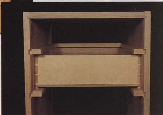
Photo U ▶ Tolerances from side to side can be very fine; this drawer (shown from the back of the carcass) slides easily with very little horizontal play.
