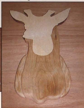
Photo 20 ▼ Gluing head, throat, neck, and shoulders together
