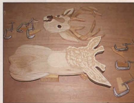
Photo 21 ▲ Applying glue before attaching head subassembly
