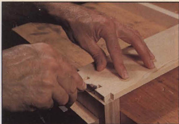
◀ Photo L Square the side to the drawer front, then knife into the end grain along the edges of the tails to establish the exact positions of the pins.
