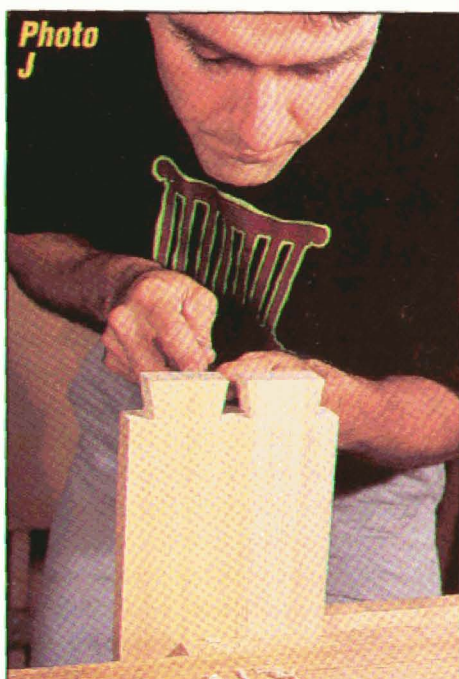
Photo J: Slice a shaving or two from the center of the shoulder so the surface will be slightly concave and won't hold the joint apart.
