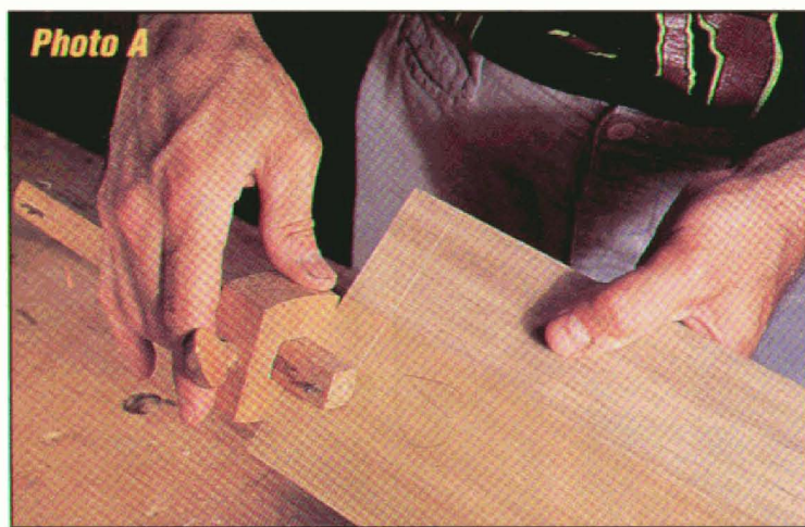
Photo A: Scribe the shoulder line for the tails around the end of each leg.
