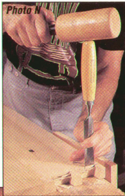
Photo N: Clean up the socket bottoms using a wide chisel.
