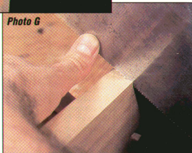
Photos F and G: Clear the bulk of the waste from the pin sockets with a coping saw, then cut away the waste at the half-pins. Cut right to the knife line on the half-pins, and you'll have little cleanup later.
