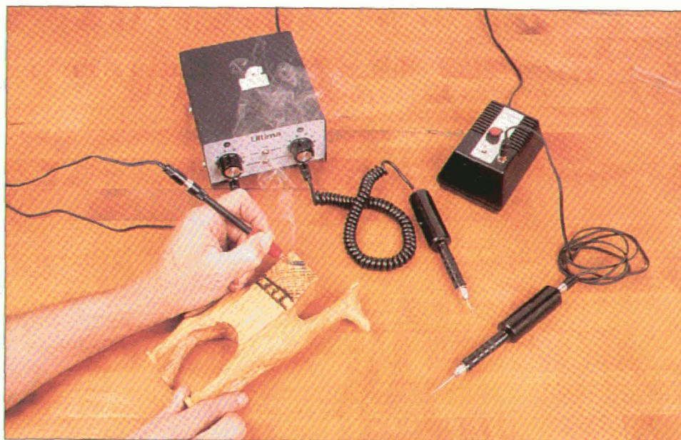
Photo 9: Ultima carver/woodburner combo (left) switches easily from "grind" to "burn" mode in seconds ($329); Optima 2 Power Carver (right) offers variable speed of 2,000 to 24,000 rpm ($275). Both are available through Woodcraft.
