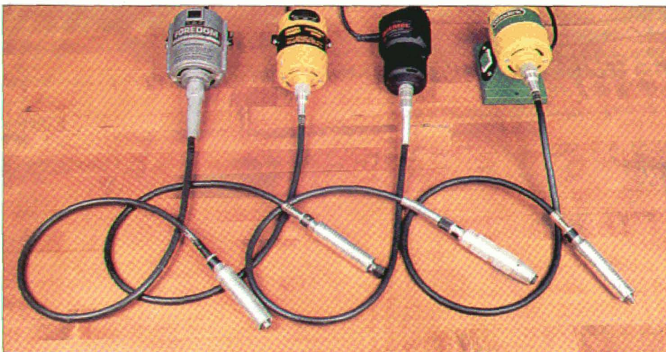
Photo 2: Flex-shaft tools, (left to right): Foredom Model SR ( \frac{1}{4} -hp, reversible, about $260 for kit); AMT model 5110 ( \frac{1}{4} -hp, reversible, includes variable-speed foot switch, $158); Dremel model 732 ( \frac{1}{4} hp, about $200 for kit); Woodtek model 876-768 ( \frac{1}{4} -hp, includes variable-speed foot switch, $130).
