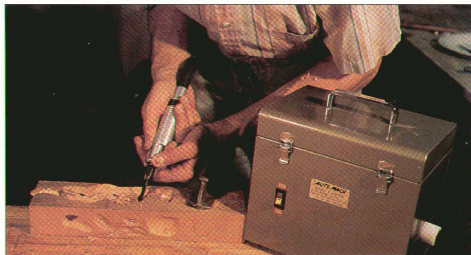
Photo 7: Automach WCS-100 woodcarver kit consists of a reciprocating handpiece connected by a flexible shaft to a quiet induction motor, which is housed in a metal carrying case. The case provides storage for the handpiece, shaft, and various accessories (about $435).
