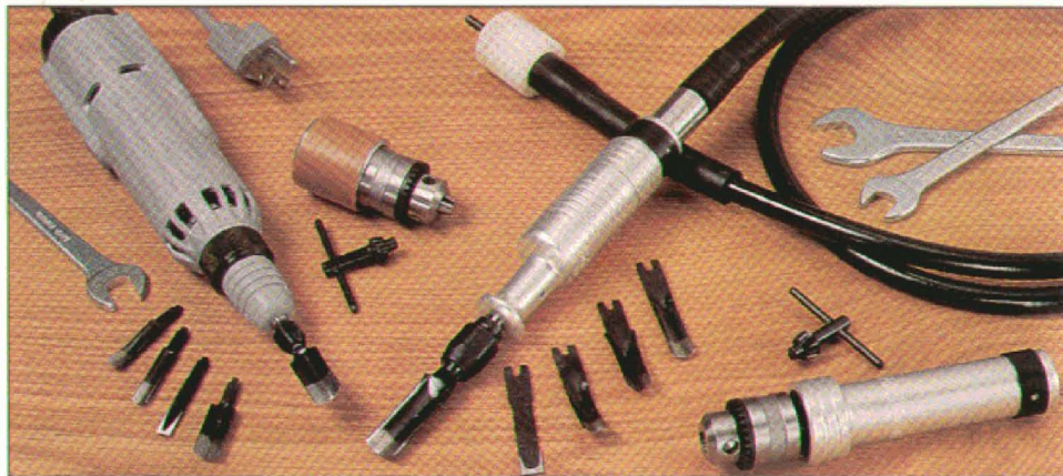
Photo 6: Automach HCT-030A reciprocating carver (at right) comes with five different cutters, wrench, and tool hanger (about $290). Jacobs-style chuck attachment converts tool to a rotary carver. Automach flex-shaft attachment (at left) fits electric drills and drill presses with \frac{1}{4} " or larger chuck capacity; it accepts rotary handpiece (bottom left). Photo courtesy Sugino Corp.
