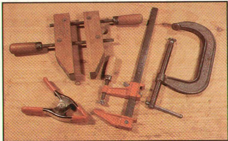
Photo C: For a wide range of clamping operations, quick-action clamps (second from right) are hard to beat. More traditional C-clamps (at right) offer many uses but less convenience. Wooden handscrew clamps (top left) are valuable for clamping non-parallel surfaces. Spring clamps (lower left), which resemble large clothespins, come in handy for small-scale, low-pressure clamping.
