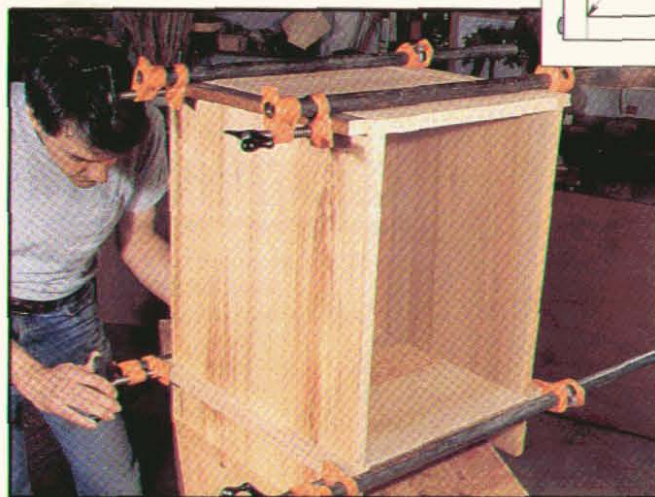
Photo M: Pipe clamps and "sprung" wooden bearers draw together the corner joints and dadoed bottom of this small carcass.
