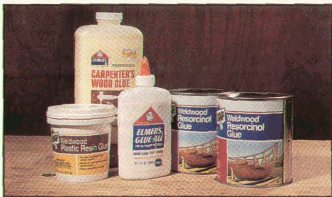
Photo A: The author finds that a white PVA glue like Elmer's Glue-All (center) takes care of most of his needs. Yellow aliphatic resin products like Elmer's Carpenter's Glue (rear) are stronger than white PVA but also set up much faster. For outdoor projects, the author uses a urea-formaldehyde glue such as Weldwood Plastic Resin. When a waterproof joint is required, he turns to two-part Weldwood Resorcinol Glue.
