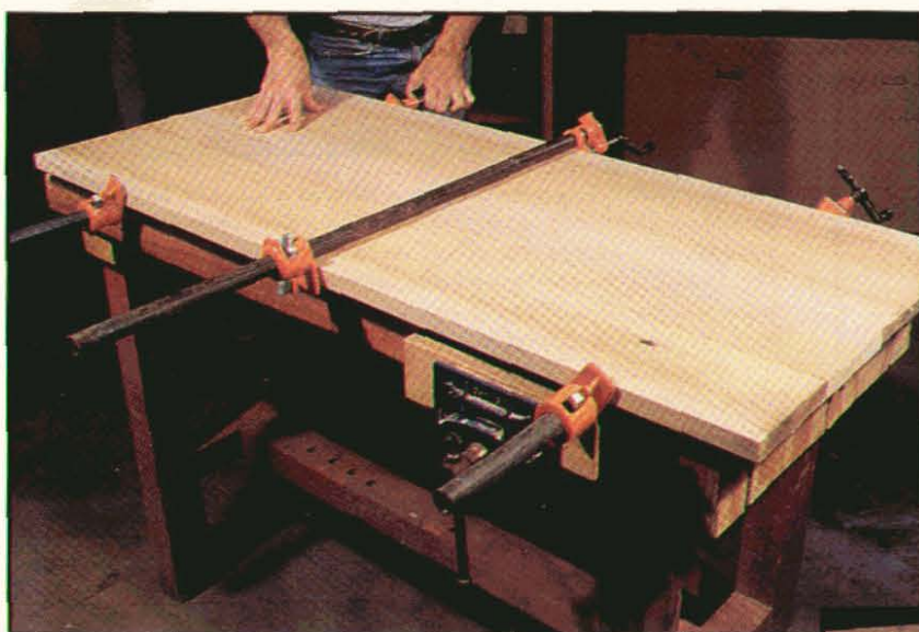
Photo D: Tabletops and panels of up to four or five feet long can be assembled with as few as three clamps, one at each end and one in the middle. Placing the center clamp on top helps counter the boards' tendency to bow away from the bottom clamps.
