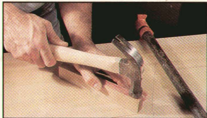
Photo H: A sharp rap with a hammer on a hardwood block will usually force edge-joined faces into alignment.
