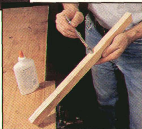
Photo G: Spread a thin film of glue on each mating surface. Here, the author uses an acid brush to spread a bead applied from the glue bottle.
