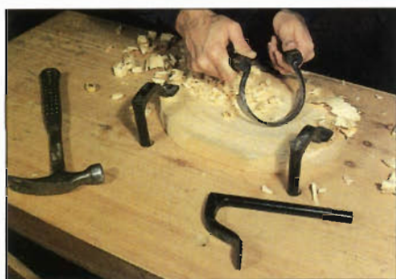
Photo D: Holdfasts are perfect for securing work, like this little Windsor chair seat, in the middle of the bench, beyond the reach of most clamps. A quick rap on the end of the shank sets the holdfast; a rap parallel to the benchtop releases it.
