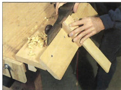
Photo H: Clamped in the face vise, the miter donkey eases the tricky task of fitting corner miters for small boxes.
