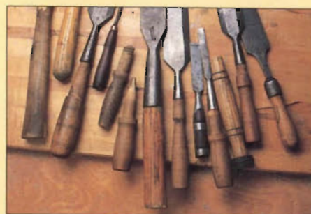
Photo 2: Most any handle can be used for a chisel, from broken broom handles to the handles of stripped old wooden clamps.
