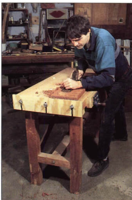
Photo A: An end stop holds the work in place for face planing and similar tasks. The pressure of planing pushes the work into the stop.
