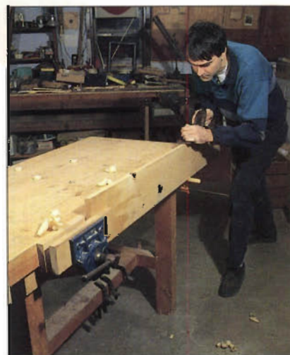
Photo C: A quick-action clamp secured to the bench leg helps support long boards for edge planing.
