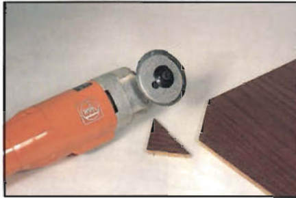
Photo 8: Mini saw blade attachment for Fein makes exceptionally smooth cuts in wood, metal, and plastics up to 5/8 in. thick. Although the blade is circular, it does not spin, but cuts in very short oscillating strokes. The adjustable disk in front of the blade serves as a stop to limit depth of cut.
