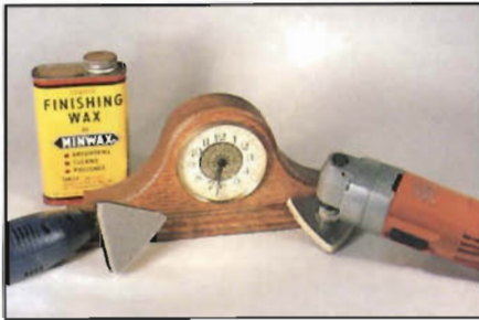
Photo 7: Foam pads (Ryobi, left), and felt pads (Fein, right) are used for a variety of wood polishing and buffing chores; here to buff out wax.
