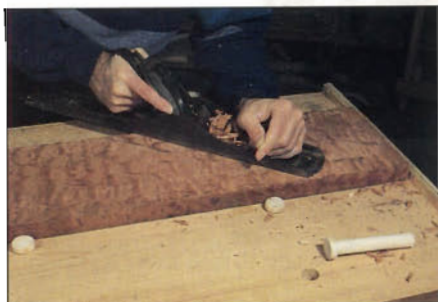
Photo B: When planing across grain, turned wooden pegs counter the board's tendency to slide sideways. A series of holes bored in the benchtop accommodate a wide variety of board sizes.
