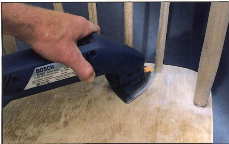
Photo 4: Quick release (orange) button on Bosch enables you to rotate sanding pad for even pad and paper wear. Triangular pad on all of these sanders enable you to squeak into tight spaces, such as between chair rungs, as shown.
