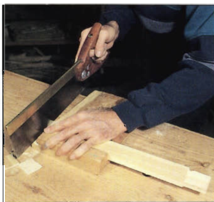
Photo E: Cutting shoulders on a tenon and other accurate crosscutting tasks are easily done with a bench hook.
