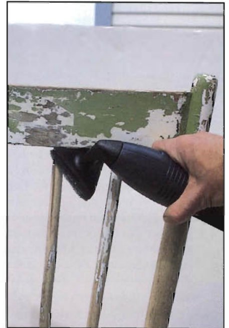
Photo 9: All three sanders have optional non-woven abrasive pads. The coarse pad shown on Ryobi can be used for stripping paint.
