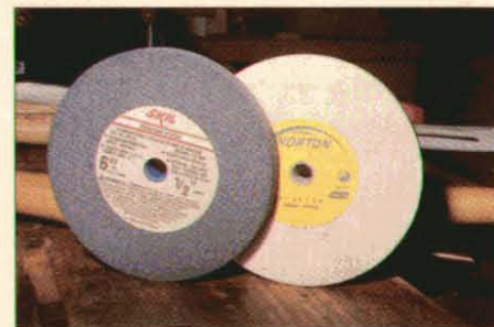
Gray carborundum wheel on left; white aluminum oxide wheel on right.
