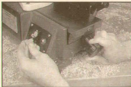
A twist knob adjusts the height of the infeed table. A removable ON/OFF switch lock prevents unauthorized use.
