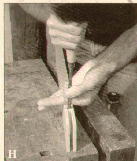
Photos G and H: Clear the mortise waste with a drill, then with a sharp chisel pare down to the layout lines marking the end of the mortise.
