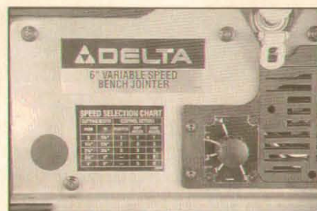
The Delta (shown) and Ryobi feature variable speed control. Both jointers have a speed selection chart attached to the machine for easy reference.
