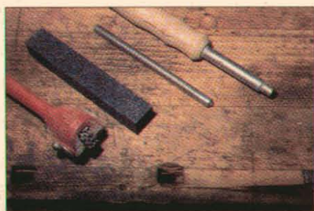
Left to right: Wheel dressers; Star-wheel; Silicon carbide dresser; Single-point diamond dresser; Diamond Jim dresser.
