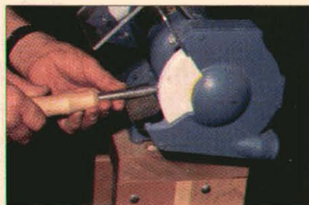
Diamond Jim being used to dress white aluminum oxide wheel on Baldor slow speed (1,800 rpm) bench grinder.
