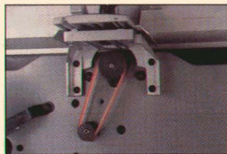
Benchtop jointers use a short belt-and-pulley drive system to power the cutterhead. The one on the Delta is easily accessible from the outside of the machine.
