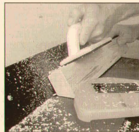
A set of push blocks is standard safety equipment on all the jointers tested. Using items such as these is one reason I still have all 10 of my fingers.
