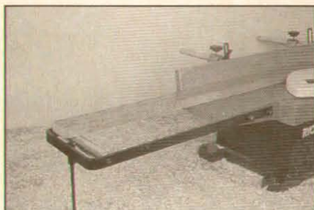
Auxiliary rollers attach to table ends on Ryobi to accommodate long stock.
