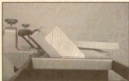
All jointers have adjustable fences, which enable you to make bevel and chamfer cuts.
