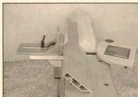
Fence on Delta has single-lever controls for tilt and across-table adjustment; fence tilts up to 45 degrees outward.
