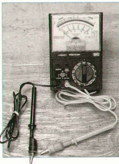
Volt/ohm meter is used to make several tests on electric motors.
