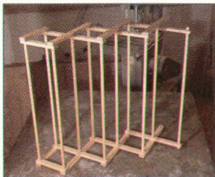
Photo A: Dry assemble the "H" subassemblies to all remaining parts
