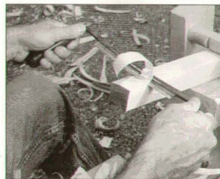
Photo D: A good way to introduce a child to the spokeshave and drawknife is to make a few cuts together, demonstrating how different movements of the hands affect the cut.
