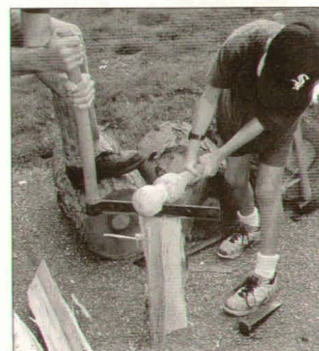
Photos B & C: To split green wood, move from iron wedges and a sledge hammer to a froe or hatchet as the pieces become smaller. Halve the piece at each stage, to help ensure a straight split. Use a large wooden mallet, not a hammer, to strike the froe or hatchet.
