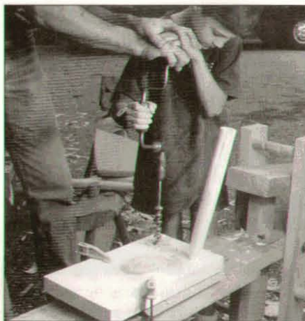
Photo J: Children usually need help steadying the brace when boring sockets in the seat. Bore the holes from the bottom of the seat, holding the brace at the desired leg angle.
