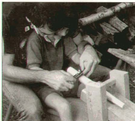
Photo D: A good way to introduce a child to the spokeshave and drawknife is to make a few cuts together, demonstrating how different movements of the hands affect the cut.
