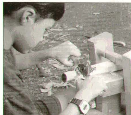
Photos E, F, G: To make a round stool leg, first shave the leg square (Photo E) along its entire length; the length of one of the square's sides should roughly equal the desired diameter of the leg. Slice off the corners to create an octagon (Photo F), then finish rounding the leg with the spokeshave (Photo G).
