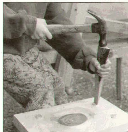
Photos K, L: After assembling the glued legs and sockets, start a split in the end of each tenon with a chisel (Photo K) then drive in a wedge to tighten the joint (Photo L).
