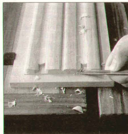
Photo 7: Remove wood with horizontal cuts.
