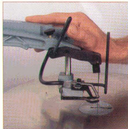
Photo 11: Front-mounted tension release lever on Delta is also available on RBI 220VS and Excaliber EX II saws.
