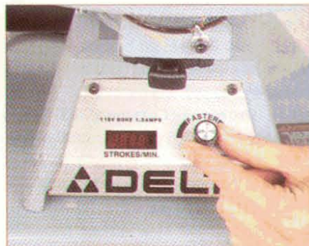
Photo 12: Delta speed control and LED readout are readily accessible (and visible) from normal operating position.
