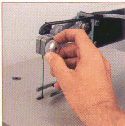
Photo 9: Finger-operated Quick Clamp on Excaliber saws: available for Delta, Hegner, and RBI as aftermarket accessory from Seyco Sales (see Sources).
