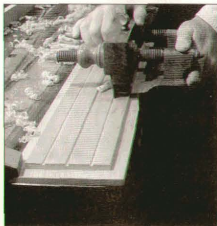
Photo 2: Use a plow plane to cut grooves.
