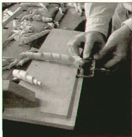
Photo 1: Cut a shoulder with a rabbet plane around the board.
