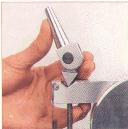
Photo 10: Cam-type lever on RBI saws enables quick tension release for changing blades.
