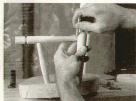
Photo P: Mark the position of the tenon shoulder on the arm.
