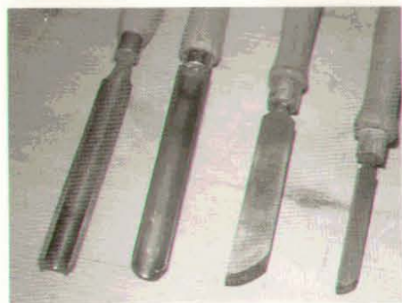
Photo A: The author turned all the parts for the child's chair with only these four tools (from left to right): A deep-fluted, 1 in. square-nose gouge for roughing out; a shallow 1 in. thumb-nail-ground gouge for shaping; a large skew, 1 in. wide, for shaping and finishing; and a small, 1/2 in. skew for trimming tenons. (The exact sizes are not critical.)
