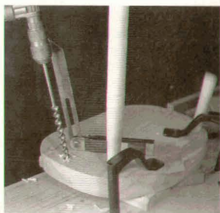
Photo N: Bore sockets for the arm and back posts, aligning the sliding bevel on the sight lines.
