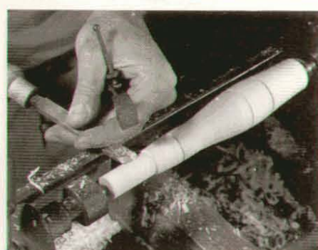
Photo F: Size the tenon with a small skew. (If you are working with green wood, do this after the tenon has dried.)
