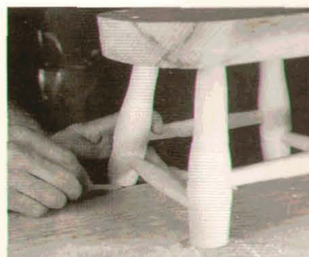
Photos S and T: Assemble the legs, stretchers and seat. Cut the front legs to length by measurement, then mark the length of the back legs using the benchtop as a straightedge.
