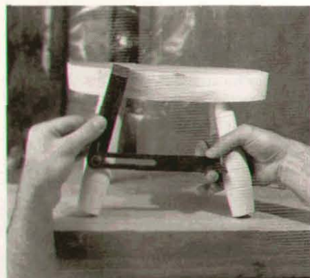
Photo J: Dry-fit the legs and seat and set a sliding bevel for the first stretcher socket in a leg.
