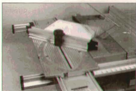
Photo 5: Sliding crosscut table on Ryobi BT-3000 can be mounted on either side of the blade.
