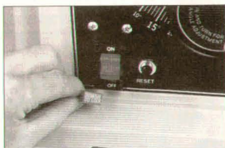
Photo 7: Removable switch on Reliant prevents unauthorized use or accidental startup; reset switch connects to circuit breaker that protects motor against overload.
