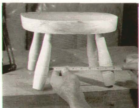
Photo H: Insert the chair legs and measure to find the length of the stretchers.
