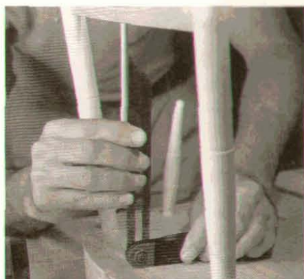
Photo Q: Set a bevel to determine the angle of the spindle sockets in the seat; a piece of dowel extends the blade to the socket position on the rail.
