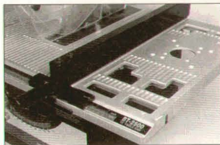
Photo 8: Like its big brother, the table on the Ryobi BT-2500 has provision for mounting a router.
