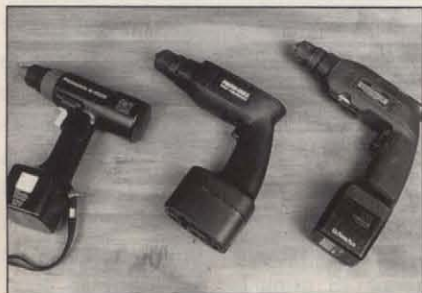
Photo 4c: Left to right: Panasonic EY6205 (12V 3/8 in. drill/driver); Porter-Cable 853 (12V 3/8 in. drill/driver); Ryobi TFD-220VR 12V 3/8 in. drill/driver).
