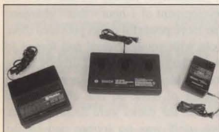
Photo 2a: Faster Chargers; Left to right: Metabo 10-minute charger takes batteries from 4.8V to 12V; Bosch three-bay multi-volt charger will charge up to three batteries at once; Panasonic 15-minute charger takes 7.2V to 12V Panasonic batteries.
