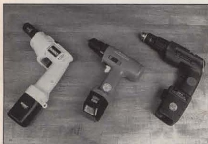
Photo 4b: Left to right: DeWalt DW945 (12V 3/8 in. drill/driver); Hitachi DS10DVA (12V 3/8 in. drill/driver); Metabo 0126 (12V 3/8 in. drill/driver).
