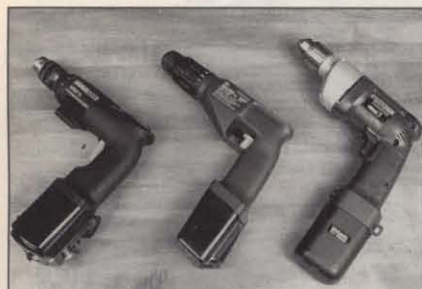
Photo 4a: Left to right: AEG ABSE 15 (12V, 1/2 in. drill/driver); Bosch 3051 VSR (9.6V 3/8 in. drill/driver); Black & Decker 2666 (13.2V 1/2 in. drill).
