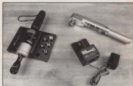
Photo 10: Two cordless tools for nuts and bolts woodworking jobs. Left: Sears Nutrunner accepts 1/4 in. drive sockets; right: SkilWrench accepts standard 3/8 in. drive sockets.
