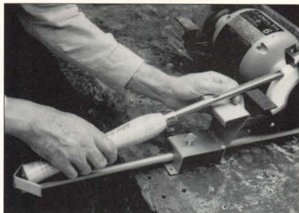
Photo 3: This jig supports long-handled turner's tools, even gouges with flat bevel profiles, as shown here. About $41 from Lee Valley Tools.
