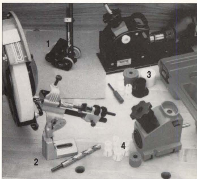
Photo 7: Universal-type honing guides from Woodcraft for straight and curved-edge carving tools: Bottom: Delux Micro Sharpening Guide ($42.50) Top: Ez-Edge Universal Sharpening guide ($79.95).
