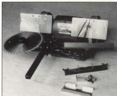
Photo 4: Makita's 5 in. bench grinder (Model 9300) includes a circular saw blade guide and planer knife guide as standard equipment. Suggested list $434. (street price considerably less).
