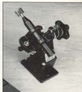
Photo 5: Router bit sharpening guide from Sears mounts to bench in front of grinder. Sears offers a similar guide for drill bits. About $20.
