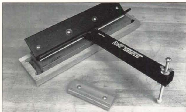
Photo 9: Top: DMT guide and 12 in. diamond benchstone handles planer blades/jointer knives up to 12 in. wide. (about $70) Bottom: Hone-Mate sharpener hones jointer knives without removing them from the machine (about $23 from Woodworker's Supply, Inc.).
