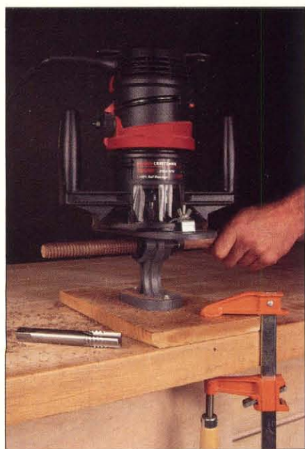
Photo C: The router-operated Beall threader quickly cuts male threads in even the hardest dowel stock—you simply twist the dowel into the unit, as shown. For portability, I mounted the unit on a short board, then clamped the board onto my bench, as shown.
