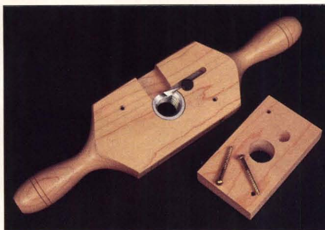
Photo A: Threadboxes from AMT and Conover (shown) enclose a V-shaped steel cutter followed by a threaded aluminum guide bushing.
