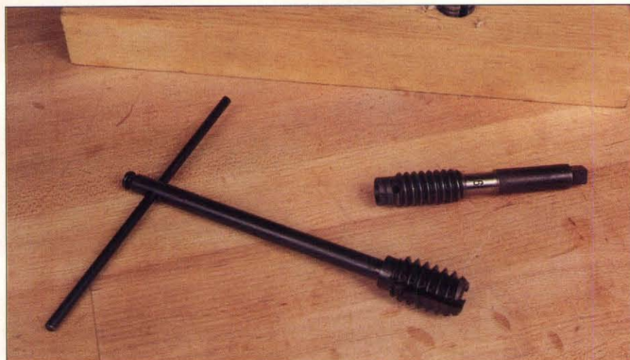
Photo E: No matter what type of threading device you buy, the taps for them all work the same way. The AMT tap in foreground has a handy T-handle; the others must be turned with a wrench.
