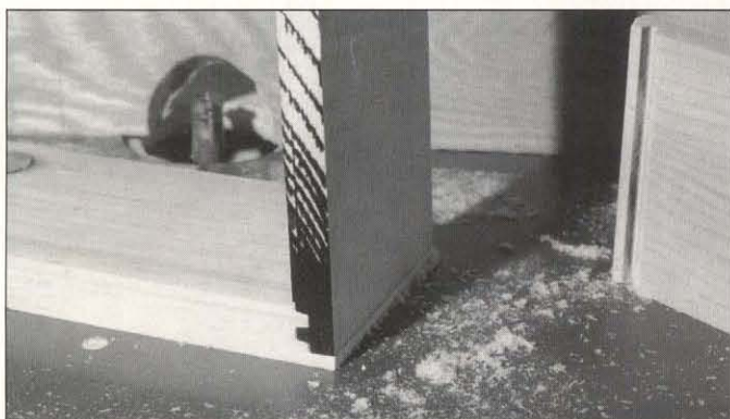
The completed drawer joint.
