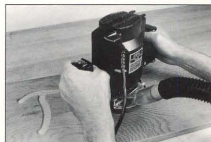
Photo 12: Clear-plastic dust pickup attachment for Skil 1835 fits standard 1 1/2 in. shop vacuum hoses, provides good bit visibility.
