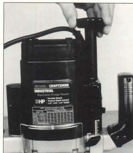
Photo 9: Extension knob on some plunge routers enables you to make fine adjustments to bit height at top of plunge stroke; facilitates use with router table (Sears).
