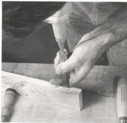
Photo G: Pare the mortise cheeks with a wide, sharp chisel. Note how the bottom hand positions and guides the tool, the top hand provides the force.
