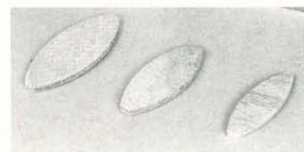
Photo 5: Depth-stop knob controls depth of cut for no. 0, no. 10, and no. 20 biscuits shown. Joiners also have micro-adjustment capability for fine-tuning the blade depth.
