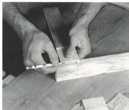
Photo L: It's easy to mark the tenon width directly from the mortise.
