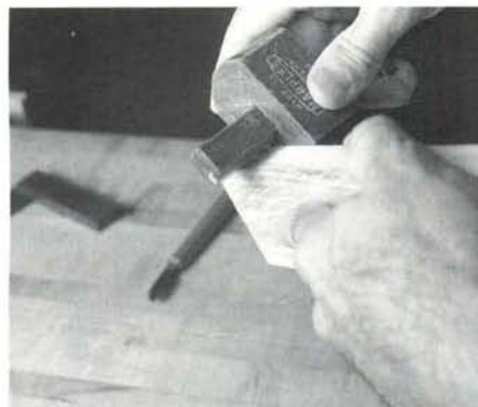
Photo C: Scribe the tenon cheeks with a mortise gauge held against the working face.
