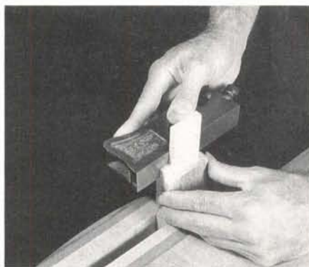
Photos M and N: A shoulder plane is ideal for trimming the cheeks (Photo M) and shoulders (Photo N) of a tenon to fit.
