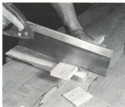
Photo K: Make the shoulder cuts right to the knifed scribe line. A bench hook is quicker to use than a vise for this job.
