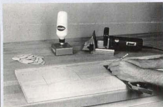
Photo 6: Align boards, then mark slot locations across the joint with a square (typically every 6–12 in. when edge-joining long boards).
