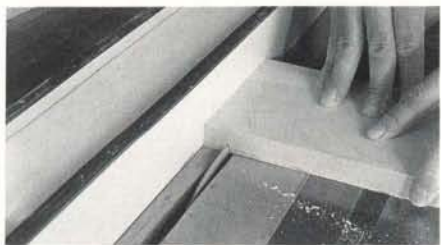
Photo F: Use a miter gauge to push narrow pieces along the fence.
