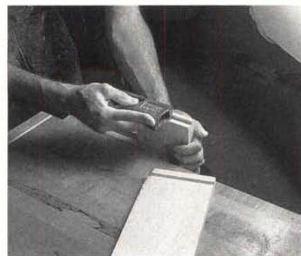
Photo H: Trim oversize tongues to fit with a sharp shoulder plane.
