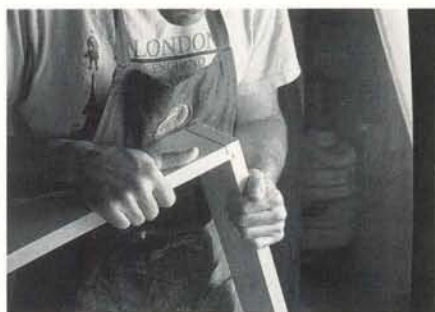
Photo E: Like its simpler sibling, the dado-and-tongue should fit snugly together.
