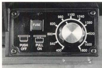
Variable speed switch on Penn State SVS-15 is fused to protect electronic circuitry. The variable speed motor and switch are sold as an accessory by Penn State, and can be retrofitted to most of the other saws in this article.
