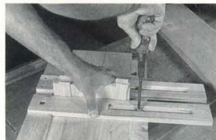
Photo B: Set the jig fences with an offcut of the correct thickness and small spacers.
