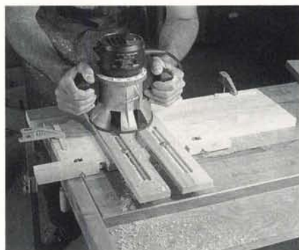
Photo A: A homemade jig makes routing dados quick and easy.
