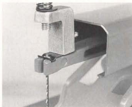
All scroll saws in this article are set up to accept pin-end blades, as shown at left. A set of small blade clamps (right).
