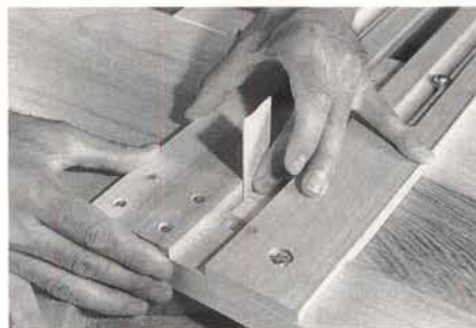
Photo C: Use a spacer to position the jig on a dado mark.
