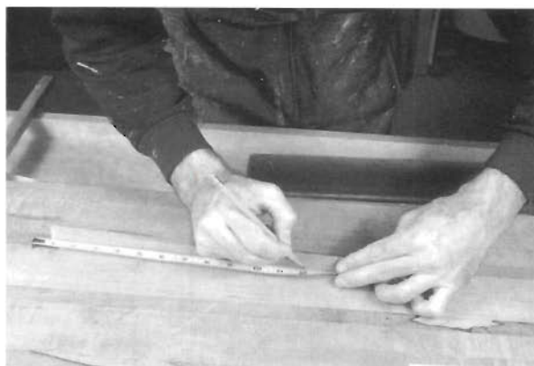
Photo 2: Measure in the rabbet to mark the length of the sides.
